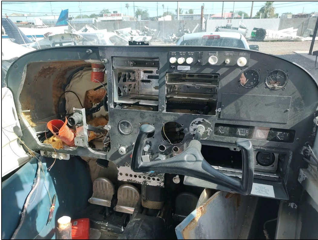
Figure 2: View of accident airplane missing various instruments (Photo courtesy of recovery company)
