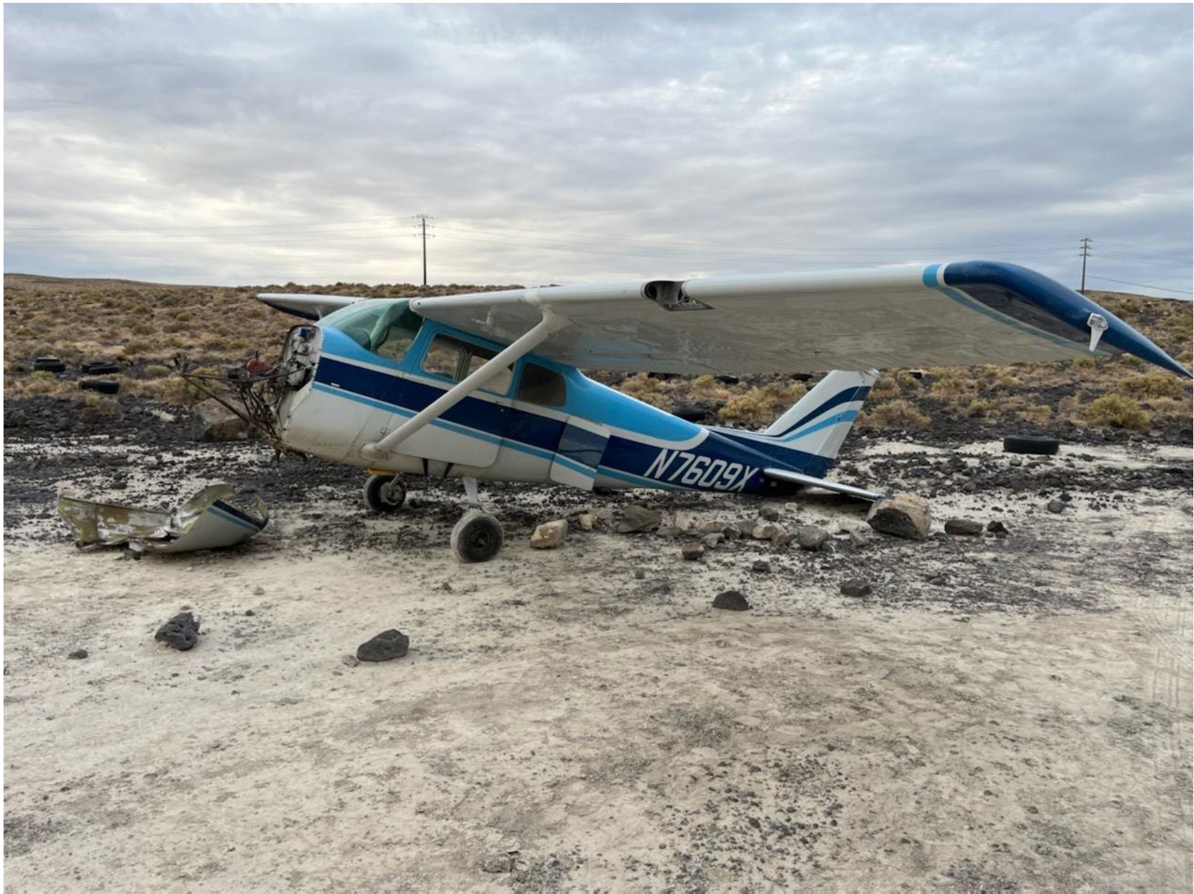
Photo 4 - View of engine missing from accident airplane (photo courtesy of recovery company)
