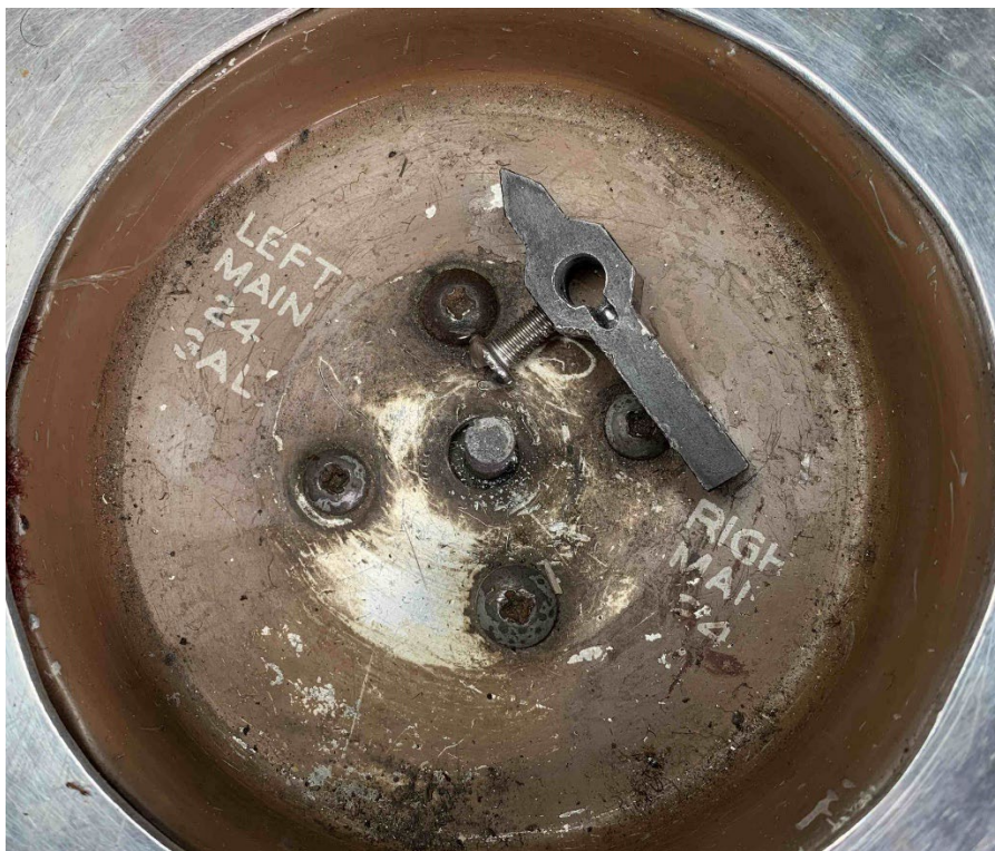
Figure 3 - Fuel selector valve handle removed.
