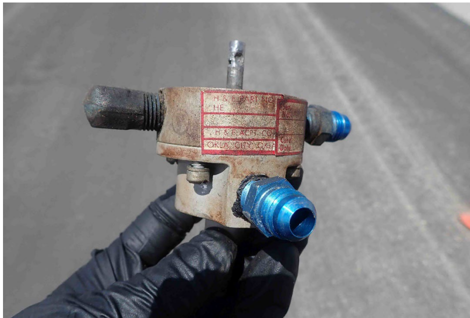
Figure 7 - Fuel selector valve removed with backed out screw.
