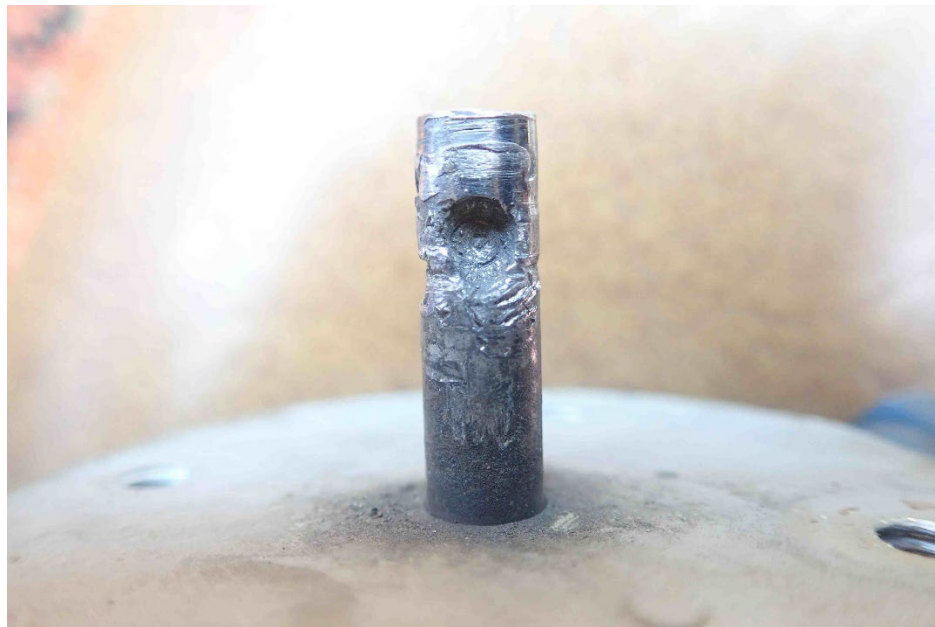
Figure 5 - Fuel selector valve shaft
