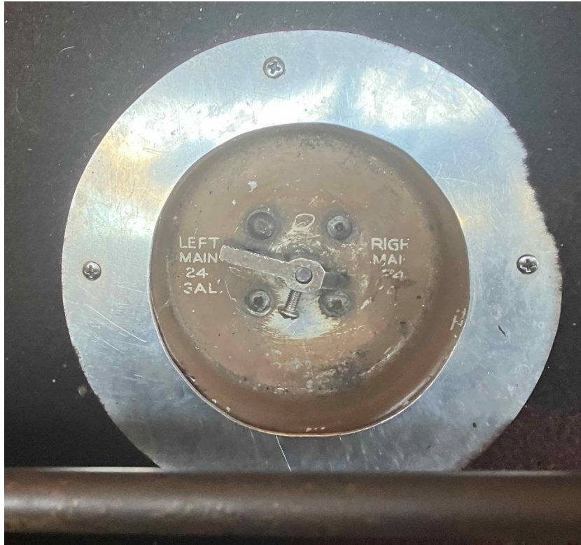
Figure 2 - Fuel selector valve immediately after accident (courtesy of Oxnard Airport Ops).
