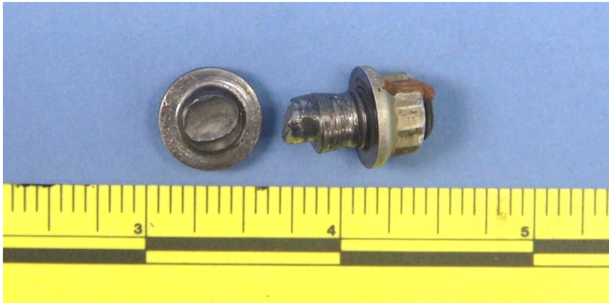
Figure 6. Mating pieces of the fractured bolt from the coupling.
