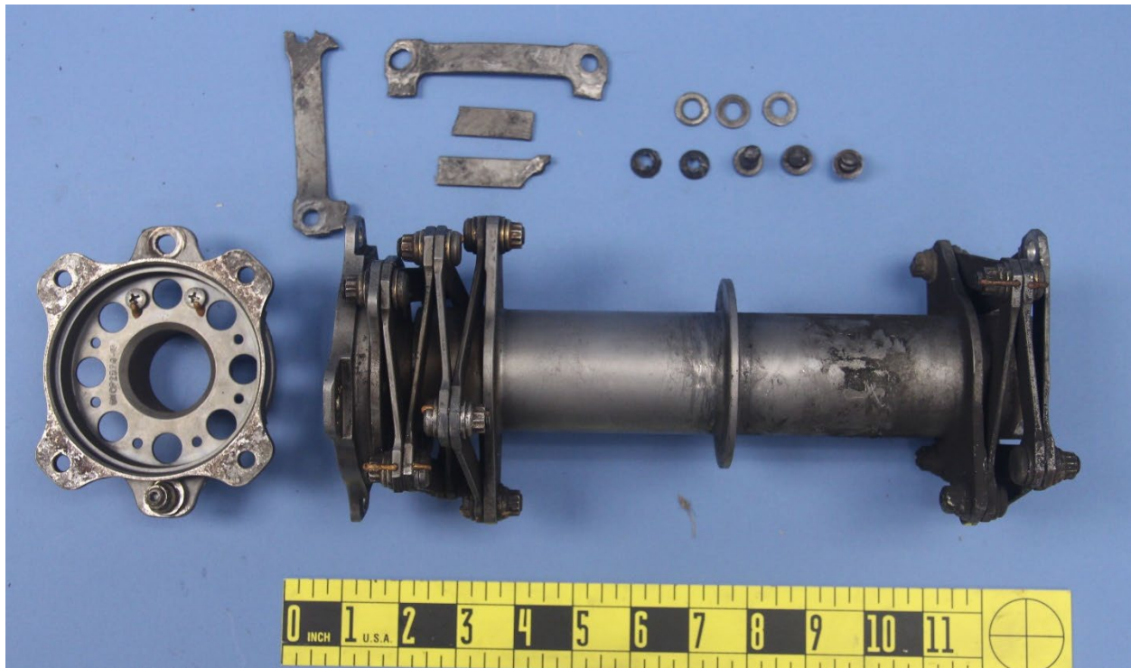
Figure 1. The components from the Kaflex coupling assembly, as received
