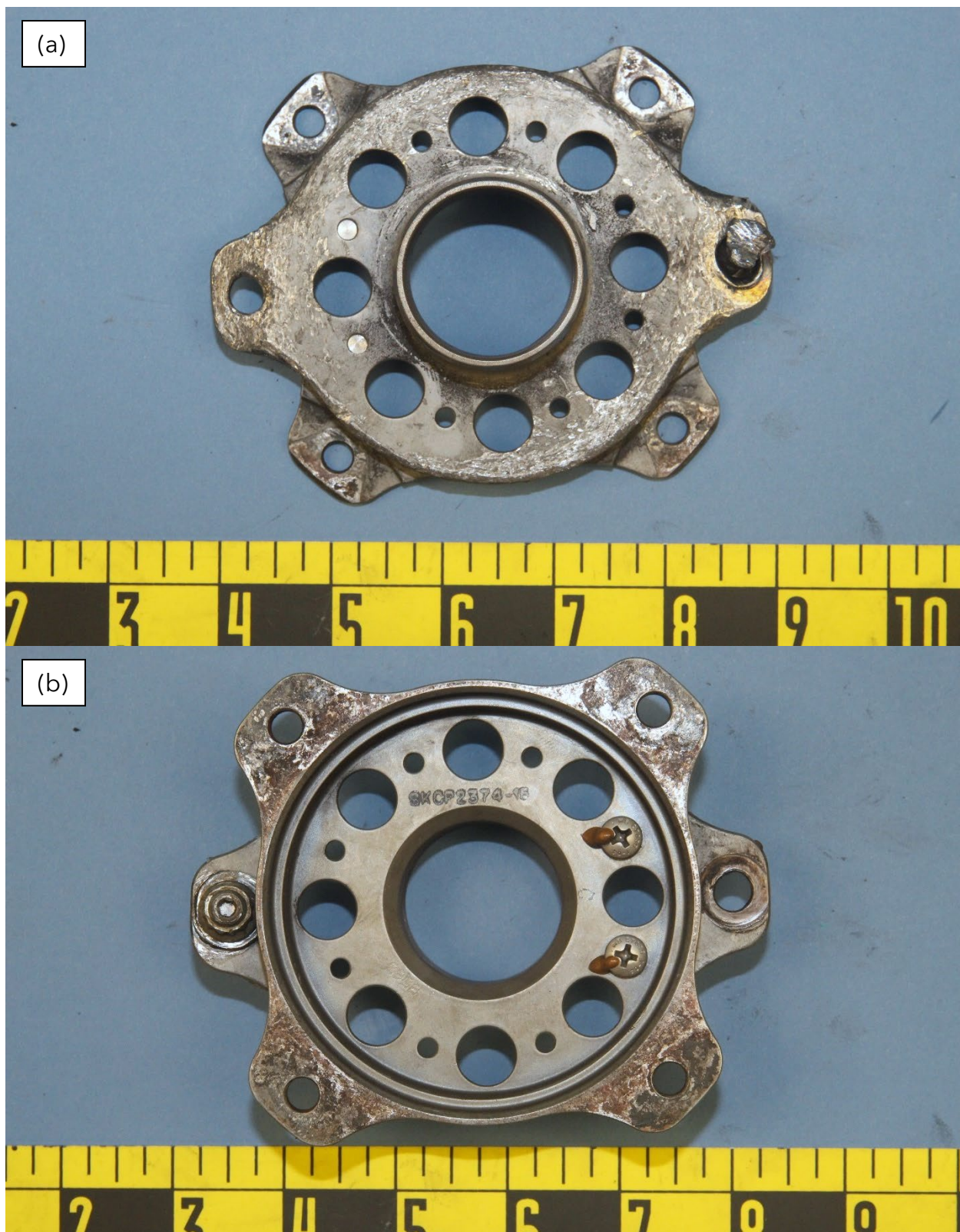
Figure 5. Views of (a) the interior and (b) exterior of the shaft end fitting.
