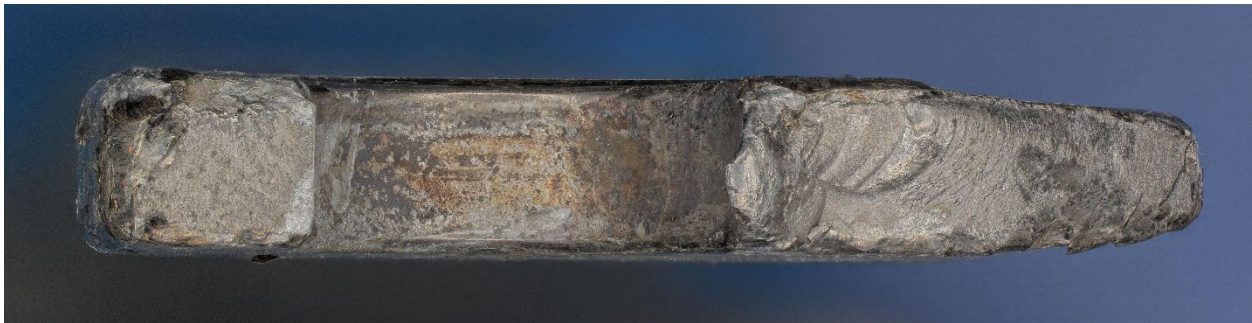
Figure 21. View of the fracture surface of the plate remnant D in Figure 20, showing crack arrest marks consistent with crack propagation from both sides of the bolt hole.
