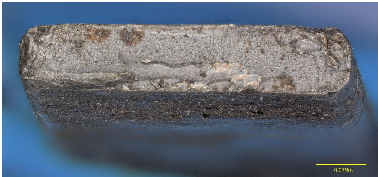
Figure 33. The fracture surface of the flex plate remnant B, showing fatigue regions, as small thumbnail cracks along the bottom edge.
