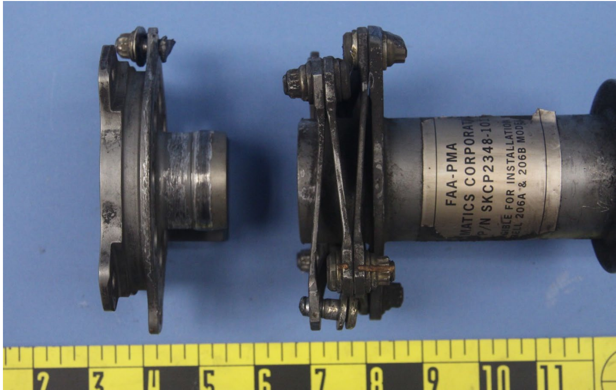
Figure 3. Closer view of the connecting cylindrical surfaces of the outer shaft end fitting and interconnect, showing circumferential wear features.
