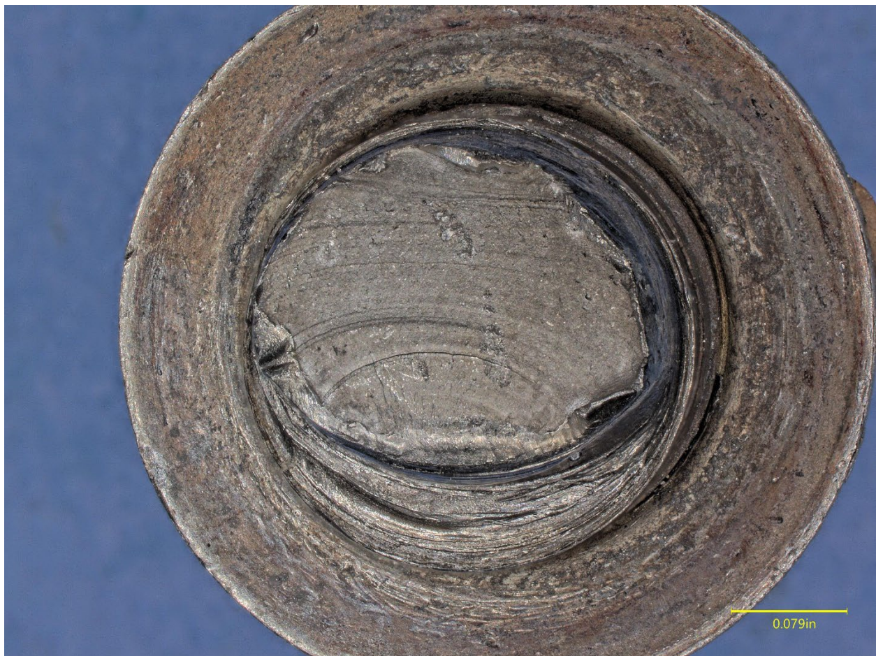
Figure 7. View of the bolt fracture surface from the shank remnant attached to the nut.
