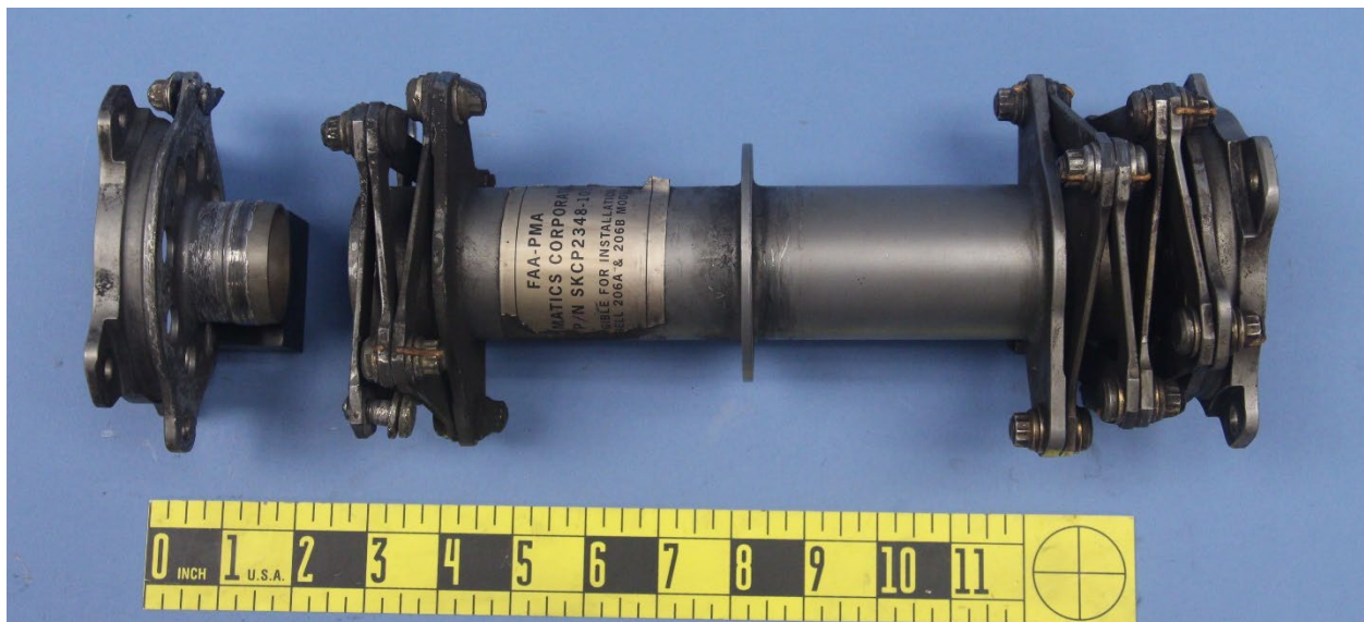
Figure 2. The shaft end fitting and interconnect fitting from the Kaflex coupling, as received.
