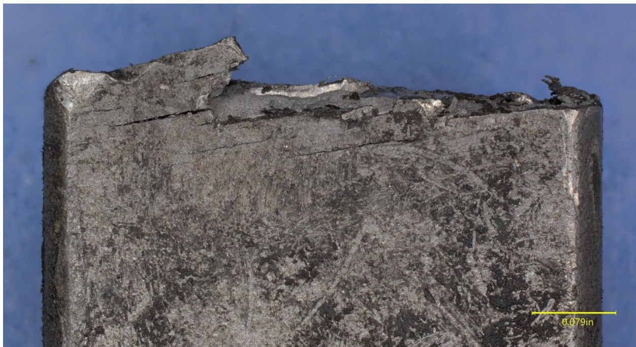
Figure 34. View of the bottom surface of the fractured plate remnant B in Figure 33, showing multiple parallel angled cracks.
