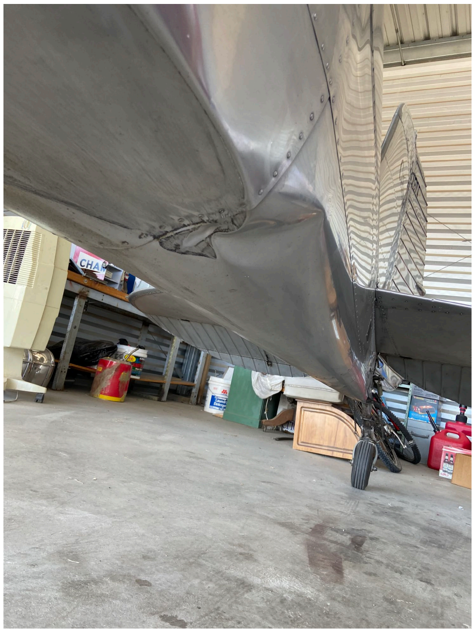
Photo 1 – View of aft fuselage damage (photo courtesy of flight instructor).
