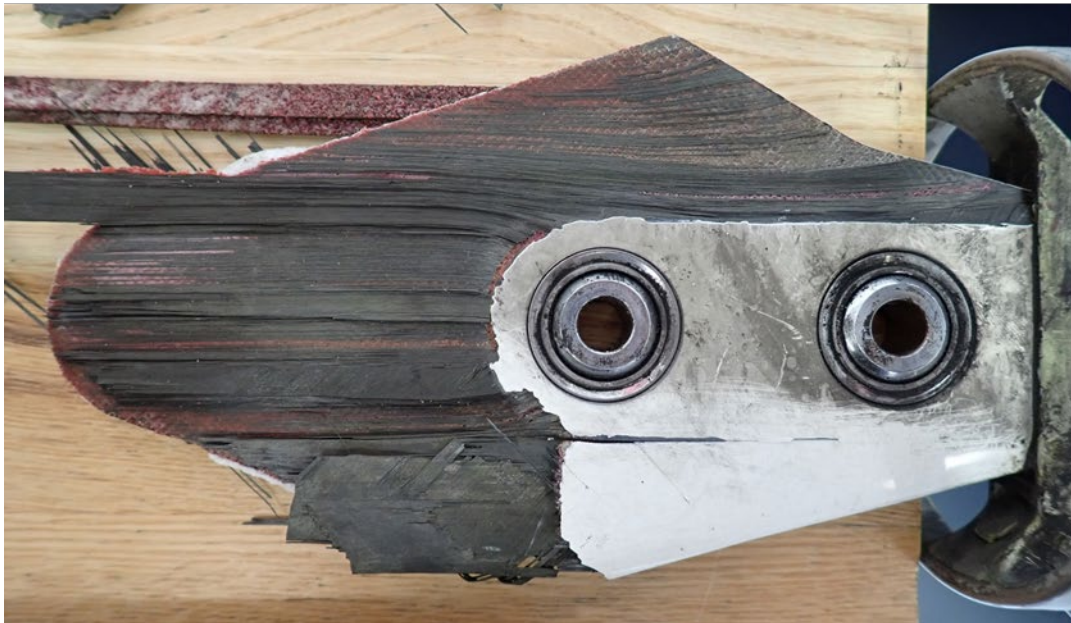
Figure 16 - C549 Root Fracture
