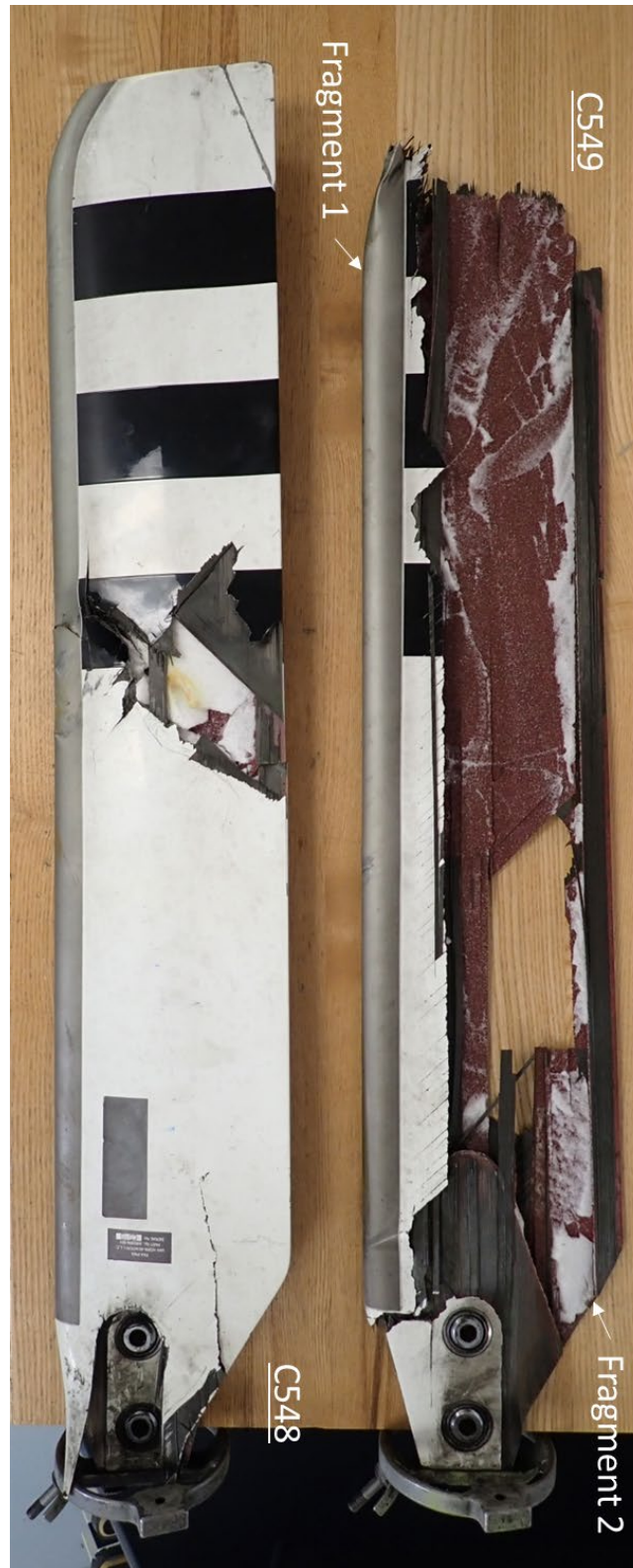
Figure 4 – Overall View of Blades C548 & C549 Upper Surfaces
