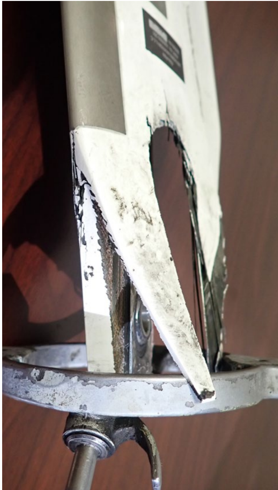
Figure 8 – C548 Root End Fracture
