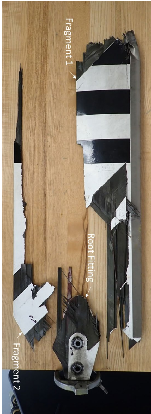
Figure 13 - C549 Fragments Lower Surface
