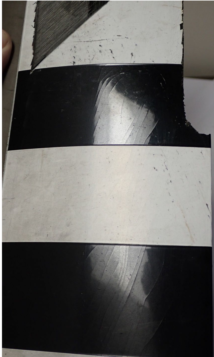
Figure 19 – C549 Fine Paint Cracks on the Lower Surface Near the Tip End
