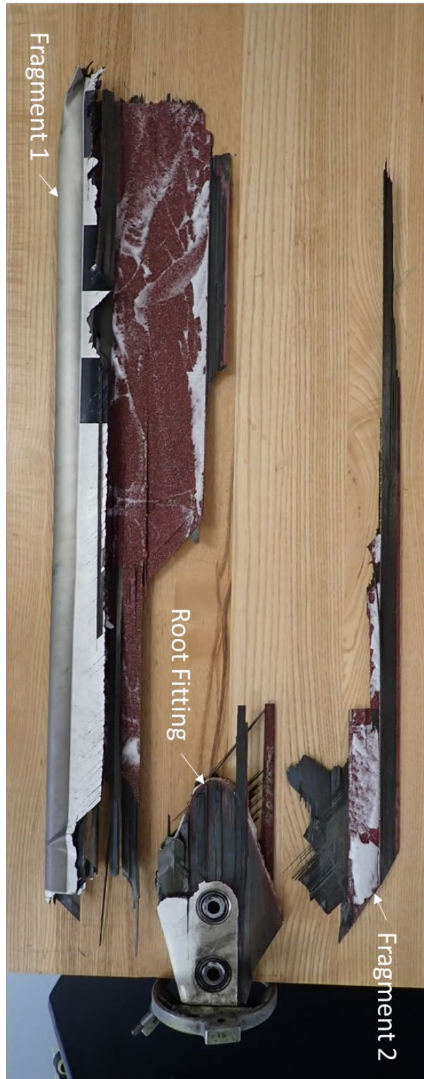
Figure 12 - C549 Fragments Upper Surface
