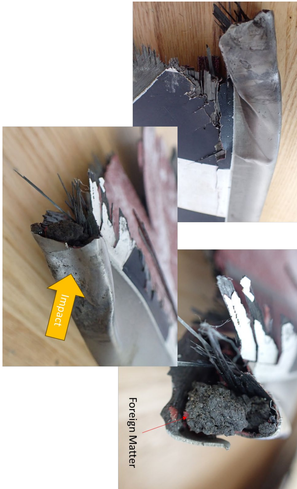
Figure 20 - C549 Tip Fracture
