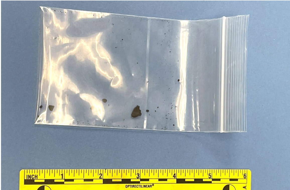
Figure 1. The debris removed from the tail rotor blade, as received.
