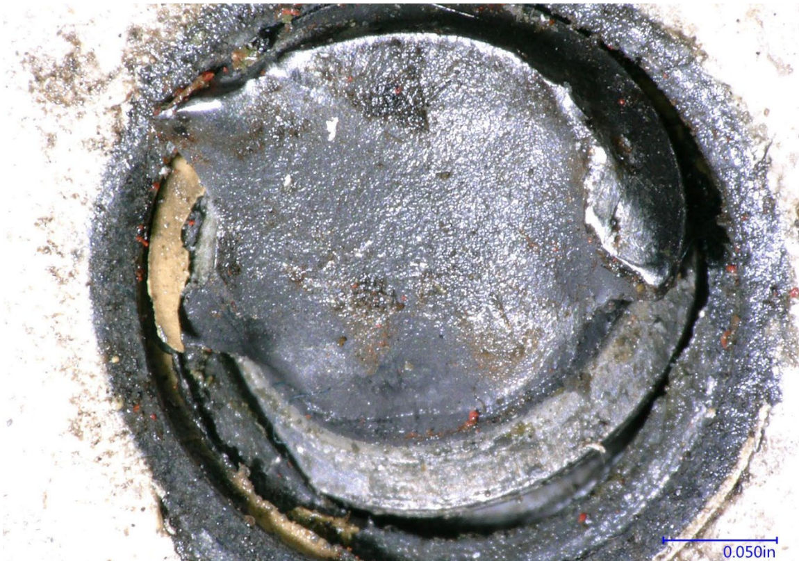
Figure 13. The fracture surface of the bolt remnant in Figure 12 , as received.
