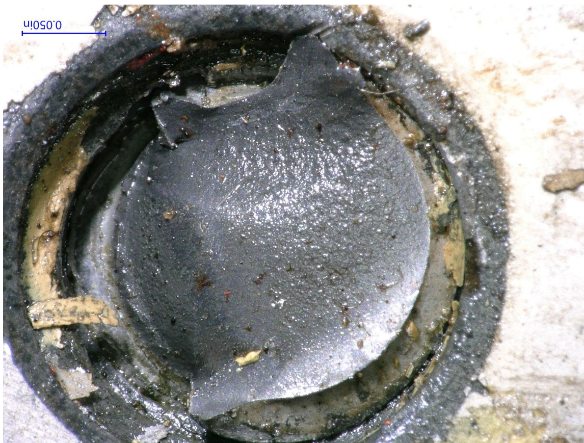
Figure 19. The fracture surface of the bolt remnant in Figure 18 , as received.
