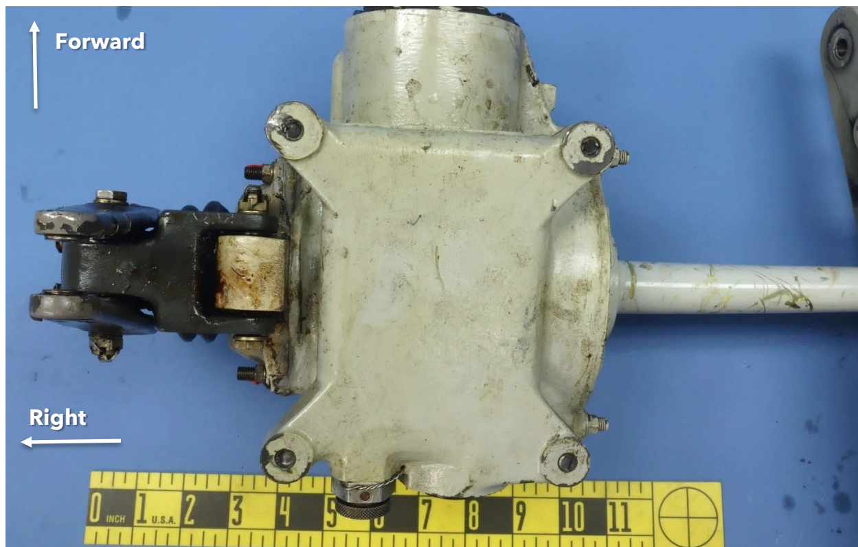
Figure 7. The interior side of the gearbox housing, showing the four fractured attachment bolts to the tailboom.
