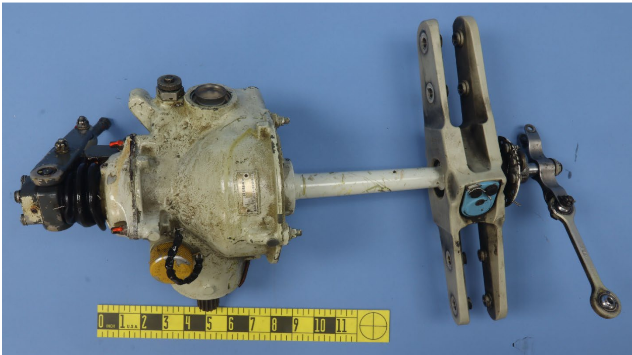
Figure 2. The reverse view of the outboard (housing) side of the tail rotor gearbox.
