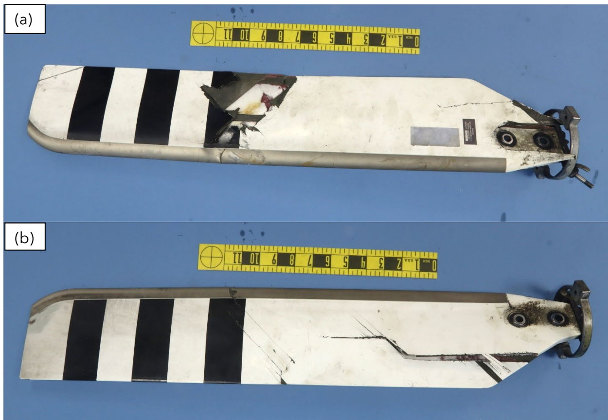
Figure 26. One of the damaged tail rotor blades from accident, viewed from (a) the exterior and (b) opposite interior sides.
