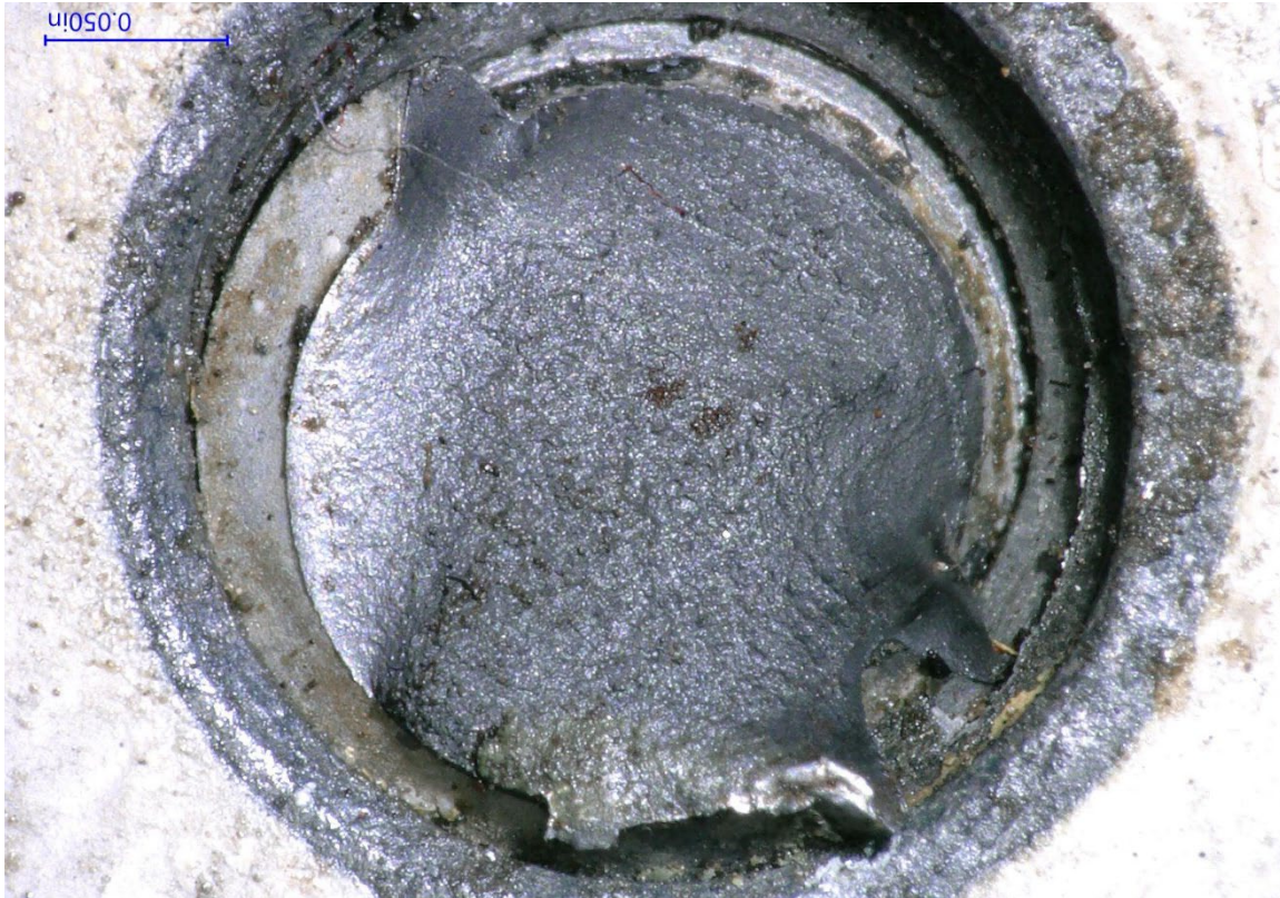
Figure 16. The fracture surface of the bolt remnant in Figure 15 , as received.
