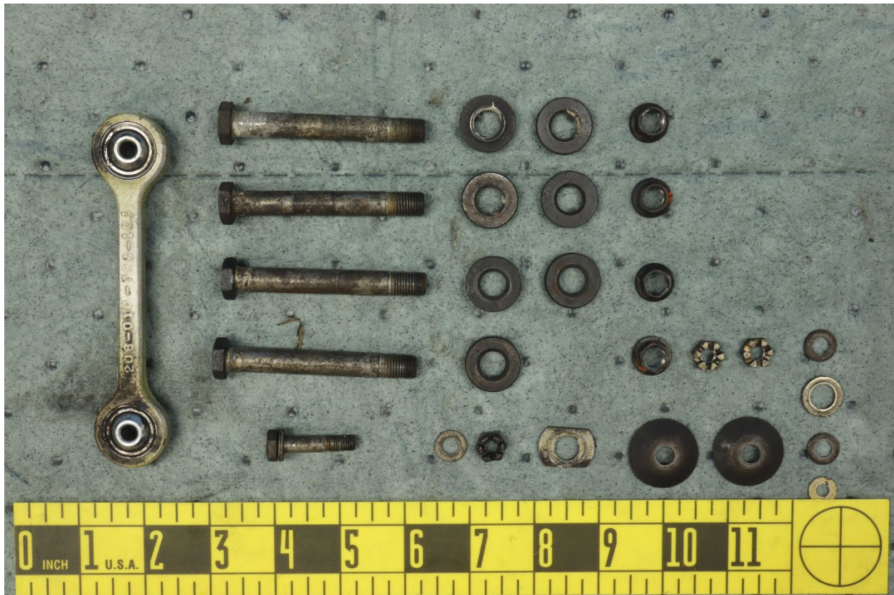
Figure 22. View of the bolts, nuts, washers, spacers, and link detached from the gearbox assembly.
