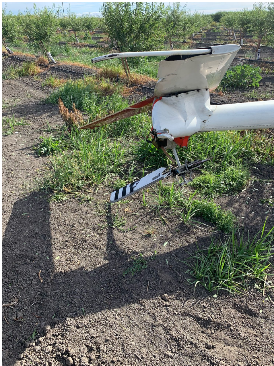
Photo 3 – Tail rotor assembly, showing the absence of one tail rotor blade. Photo courtesy of the operator.
