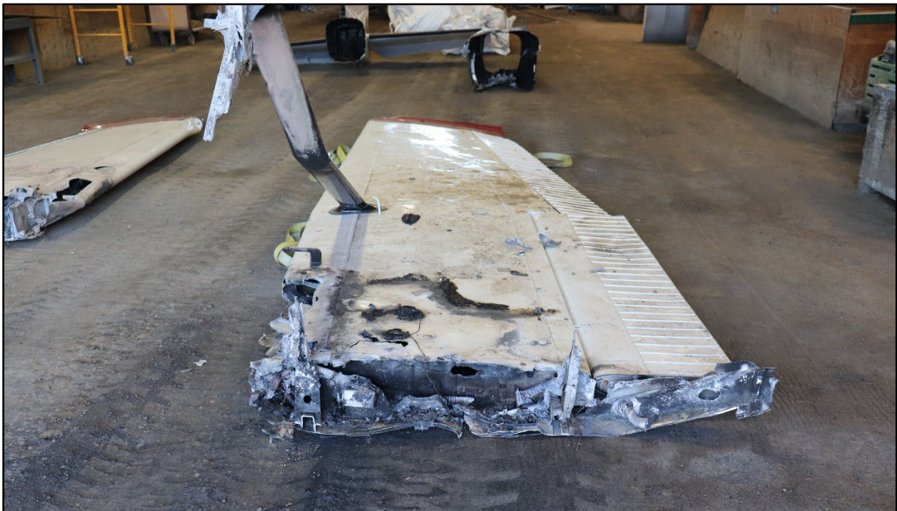
Figure 5: View of left wing thermal damage.
