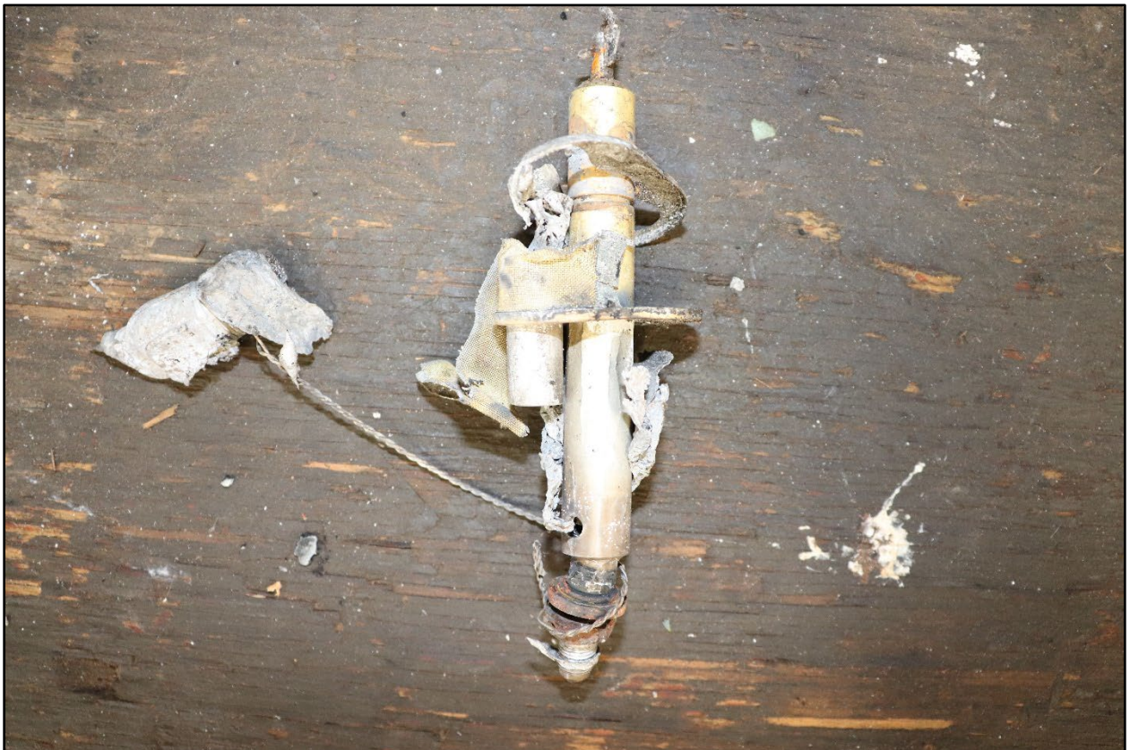
Figure 2: View of airframe fuel strainer assembly damage.
