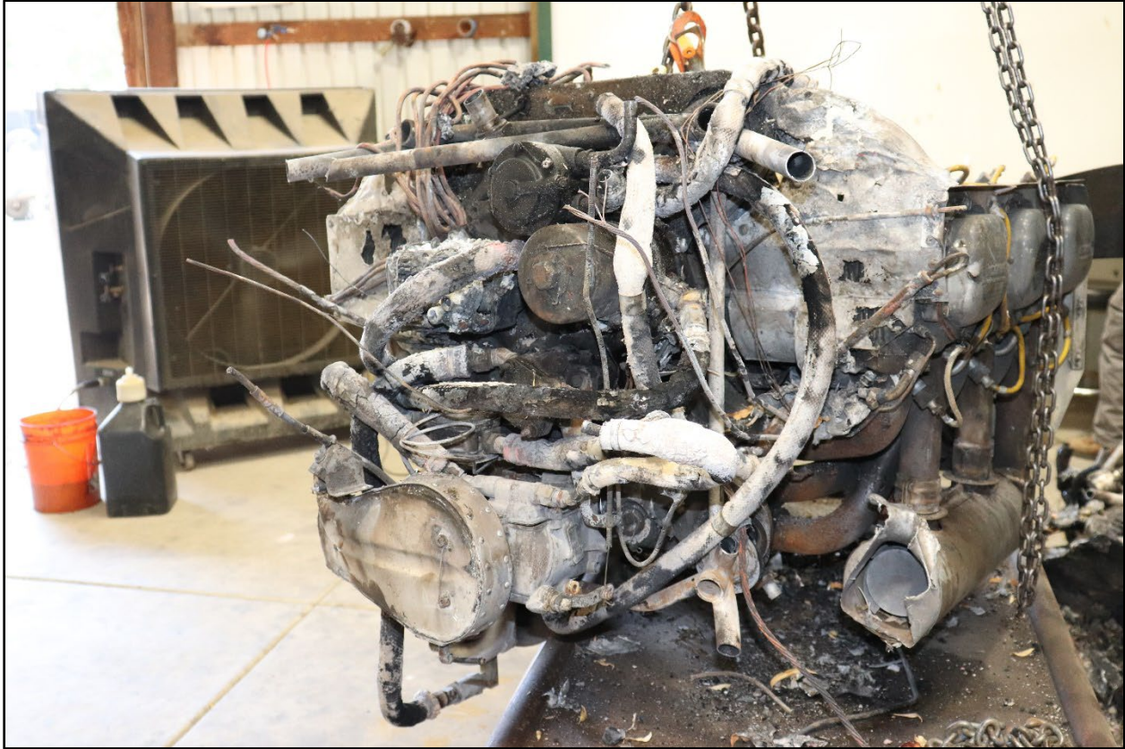
Figure 7: Rear view of engine thermal damage.
