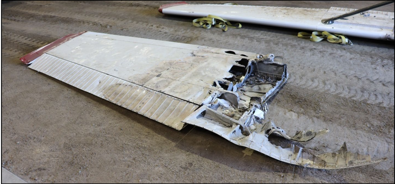
Figure 4: View of right wing thermal damage.
