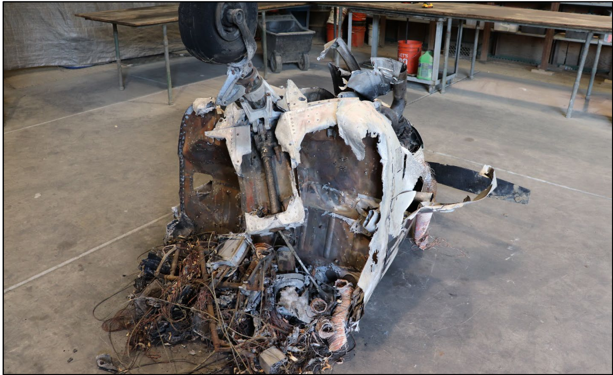
Figure 3: View firewall thermal and impact damage.
