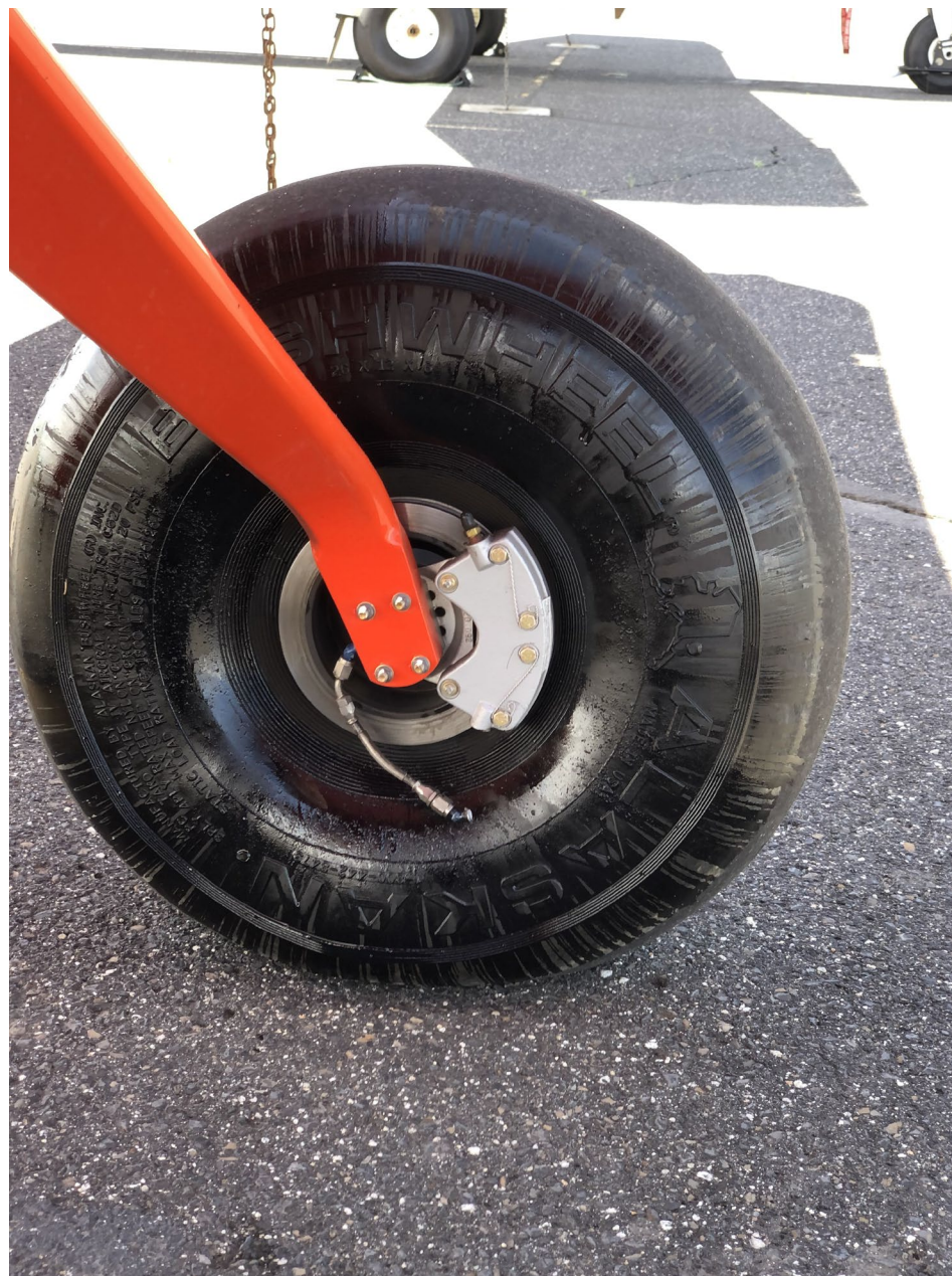
Photo 3 - View of left brake line damage (photo courtesy of the pilot)
