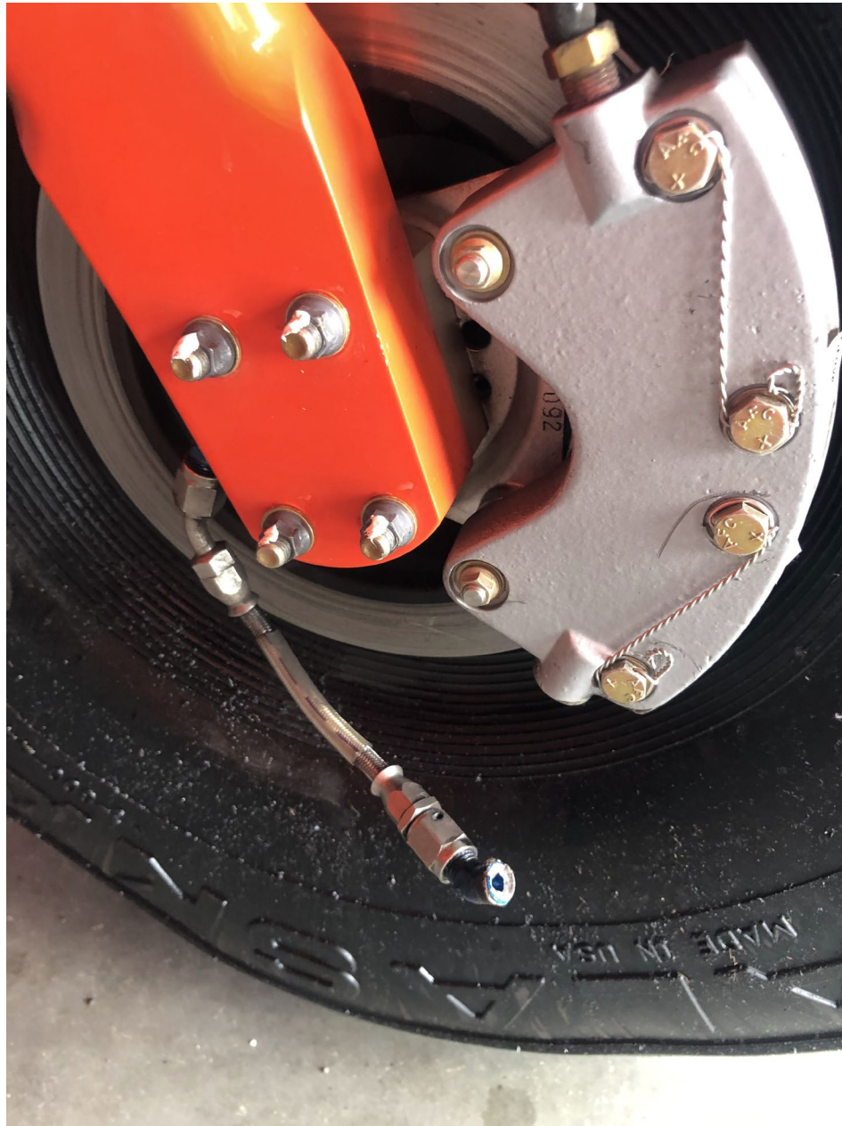
Photo 4 - View of left brake line damage (photo courtesy of the pilot)
