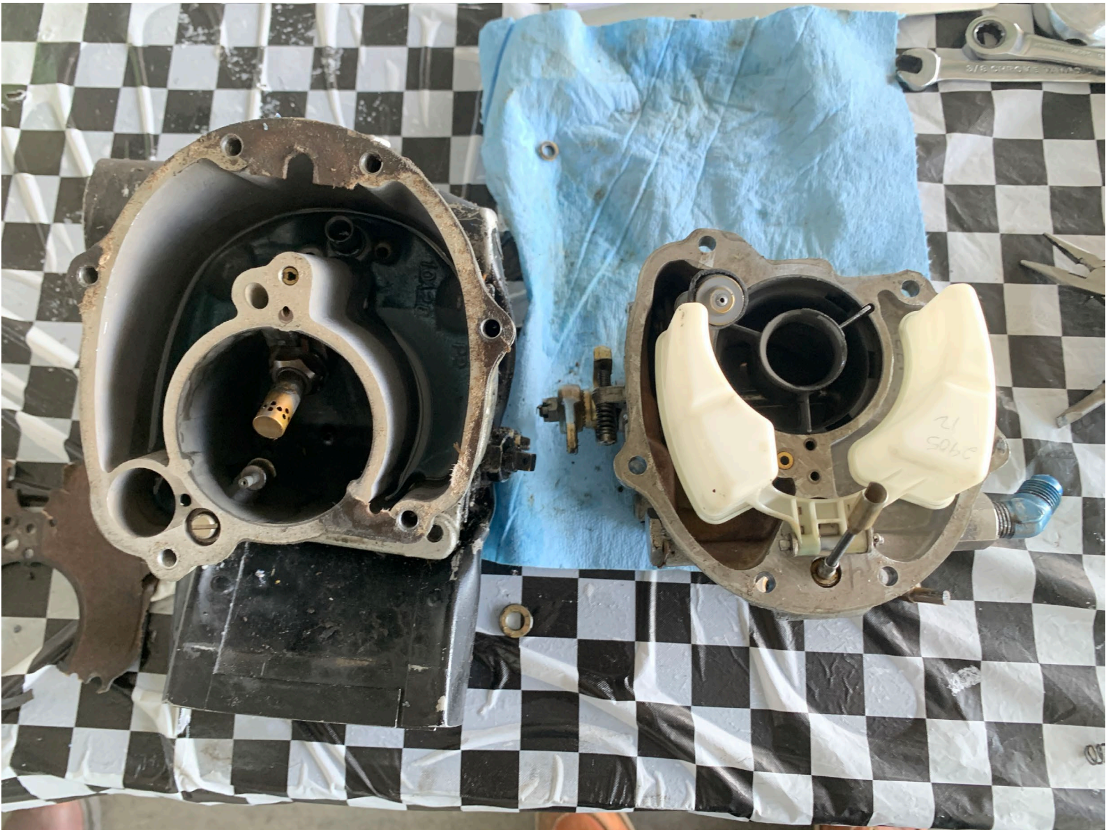
Photo 8 – View of opened up carburetor
