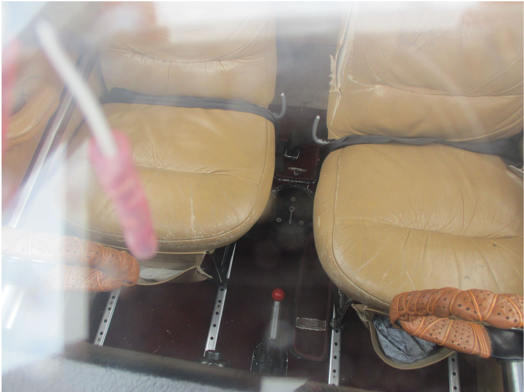
Photo 4 – View of fuel selector valve lever position in the OFF position (courtesy of the FAA)
