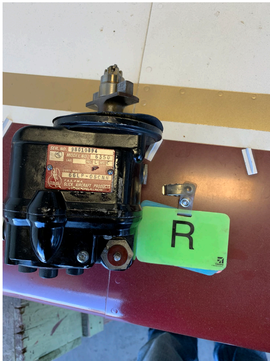
Photo 9 – View of removed right magneto
