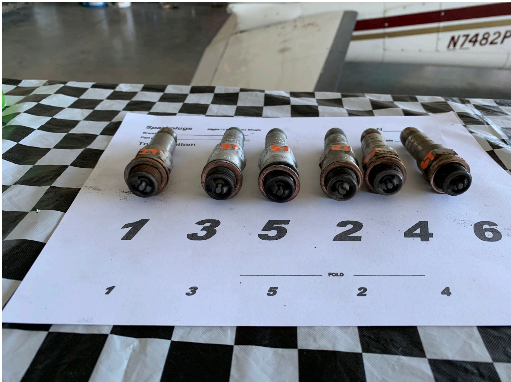
Photo 7 – View of removed top spark plugs
