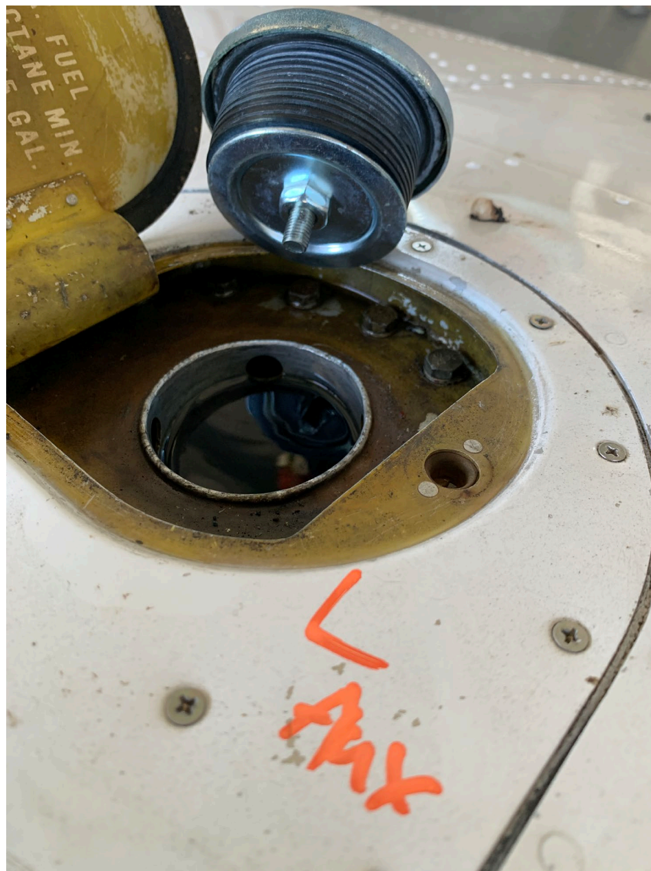
Photo 5 – View of left wing left auxiliary fuel tank opening
