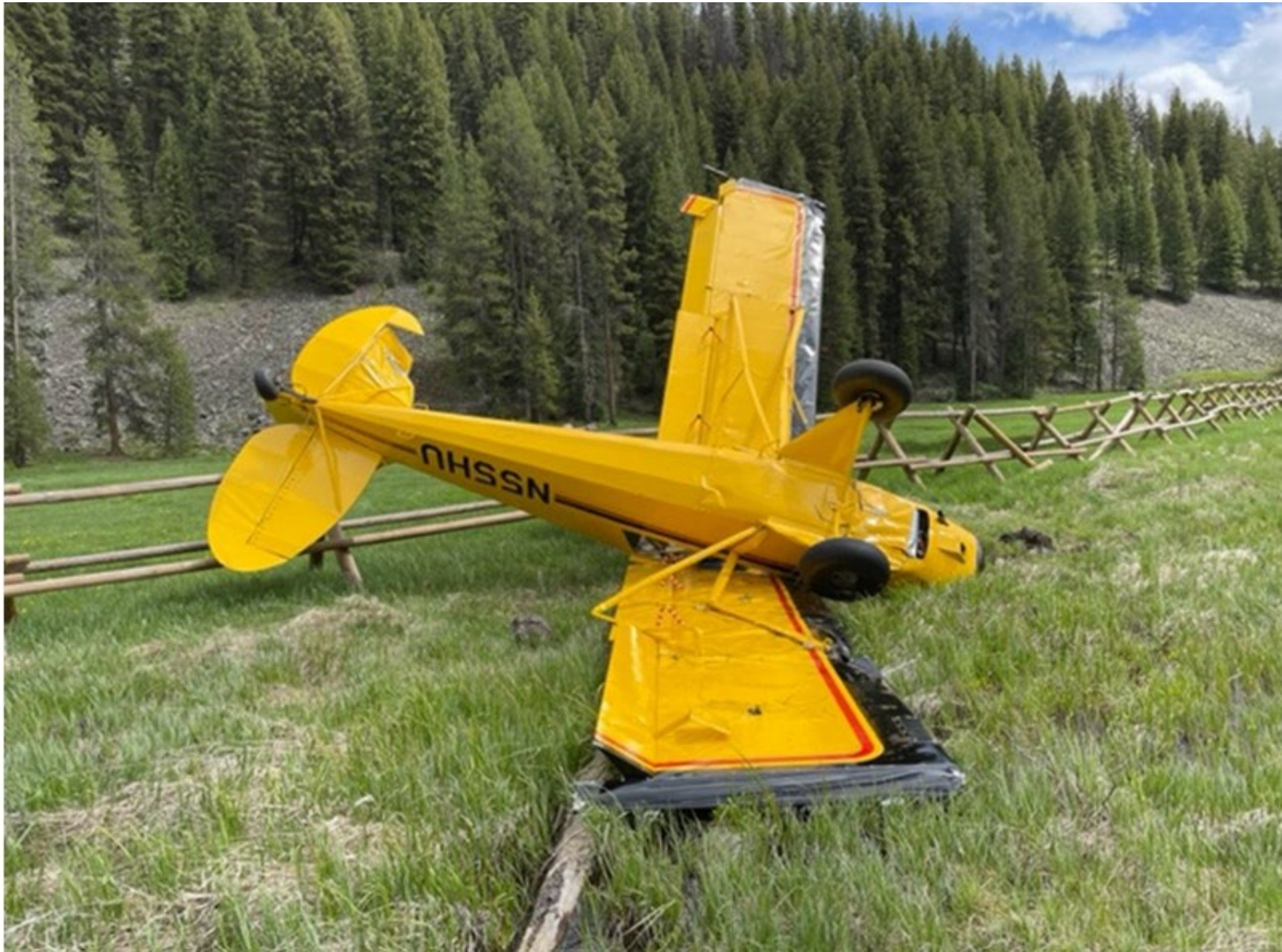
Photo 1 – Left side damage (Photos courtesy of Joey McGuire)
