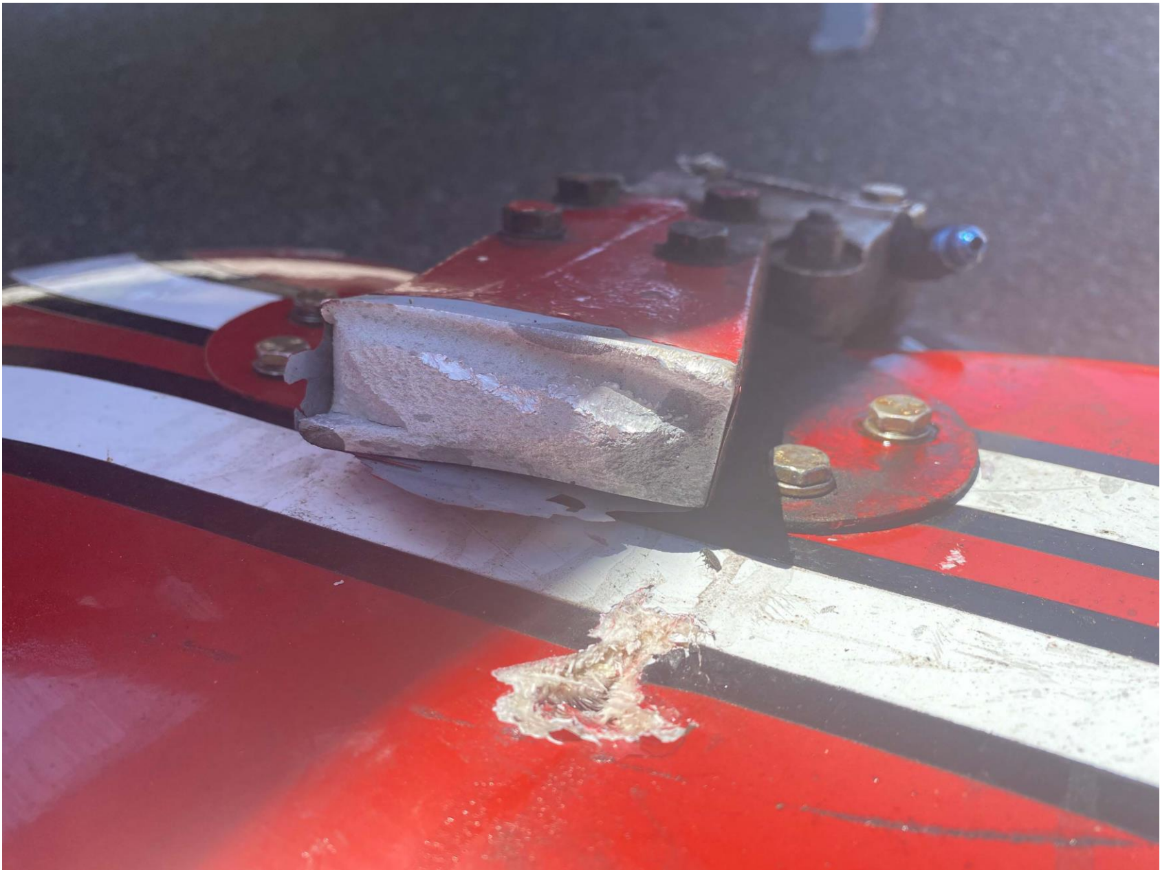
Photo 5 – Accident site, wheel pant and strut separation surface. (Courtesy of the FAA)
