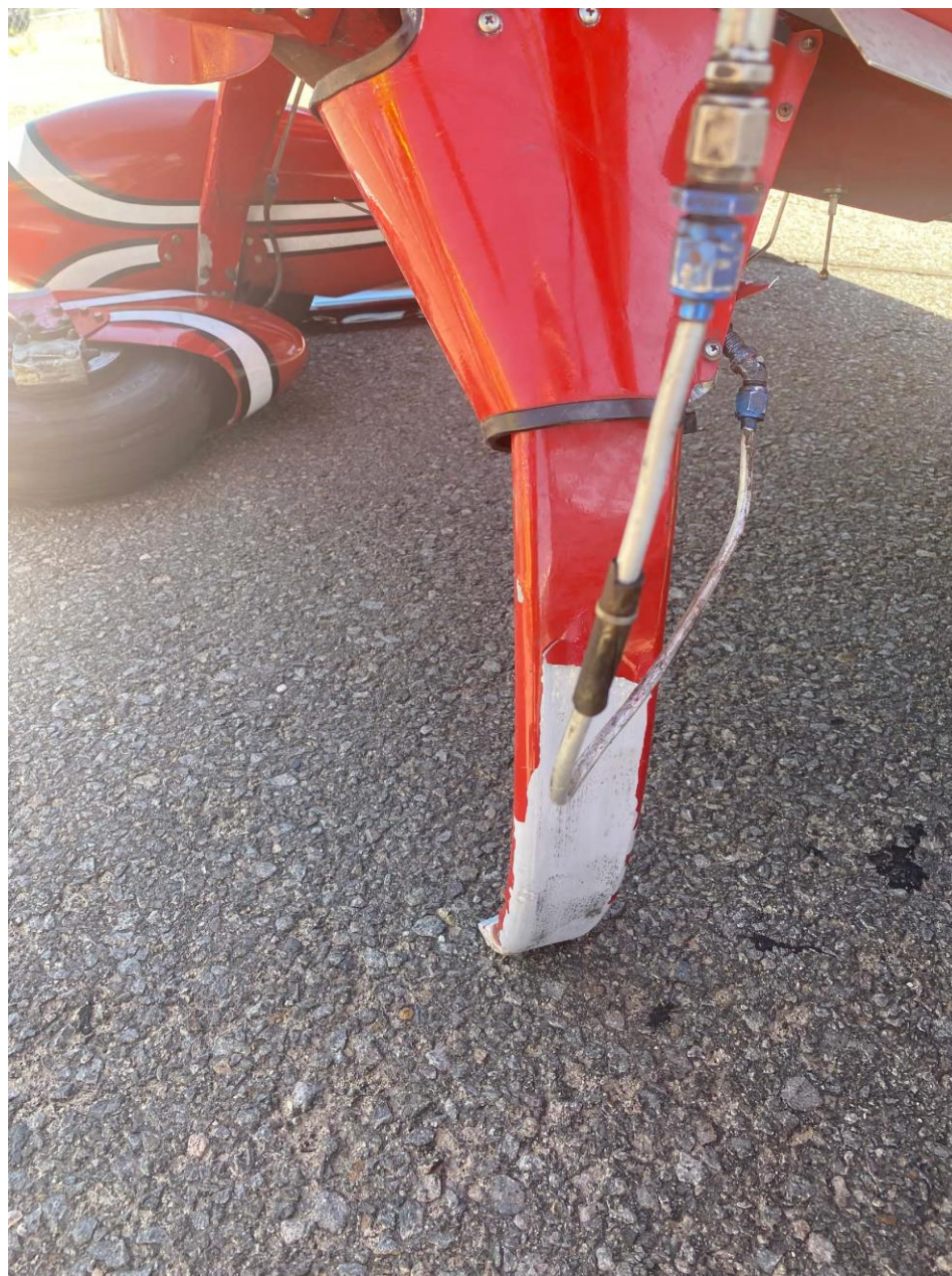
Photo 3 – Accident site, left main gear strut. (Courtesy of the FAA)
