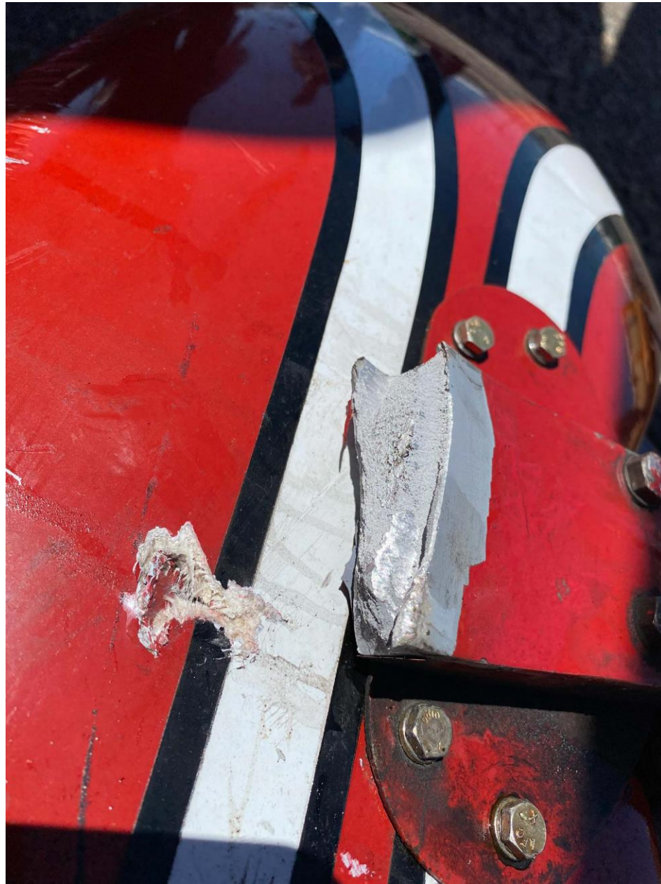
Photo 7 - Accident site, wheel pant and strut separation surface. (Courtesy of the FAA)
