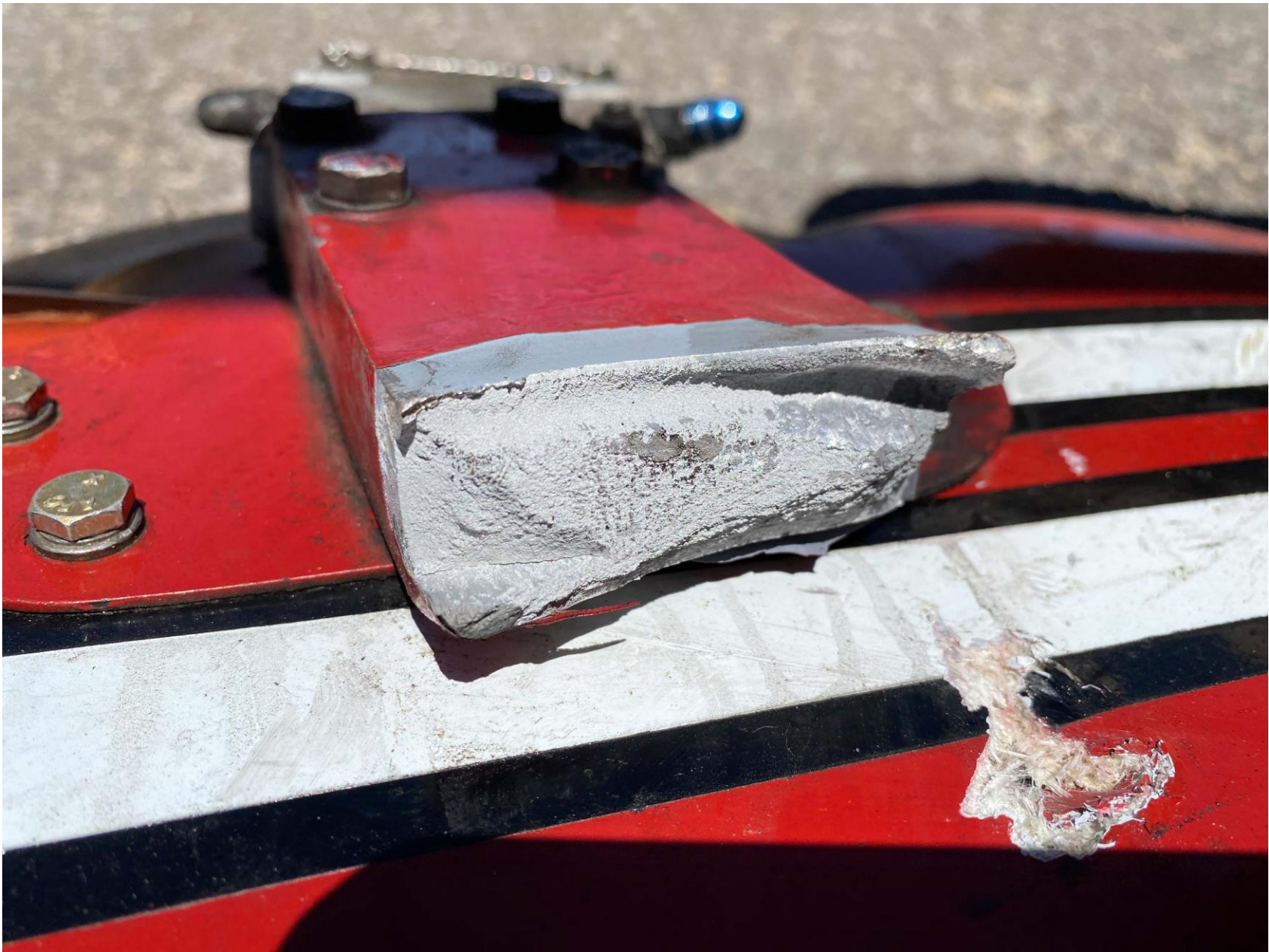
Photo 8 - Accident site, wheel pant and strut separation surface. (Courtesy of the FAA)
