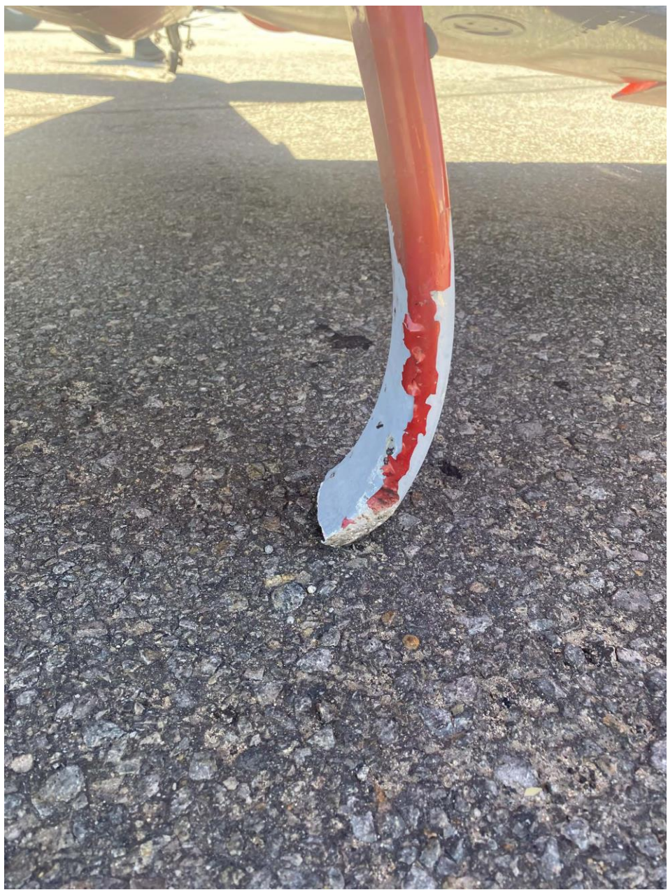
Photo 4 – Accident site, left main gear strut. (Courtesy of the FAA)
