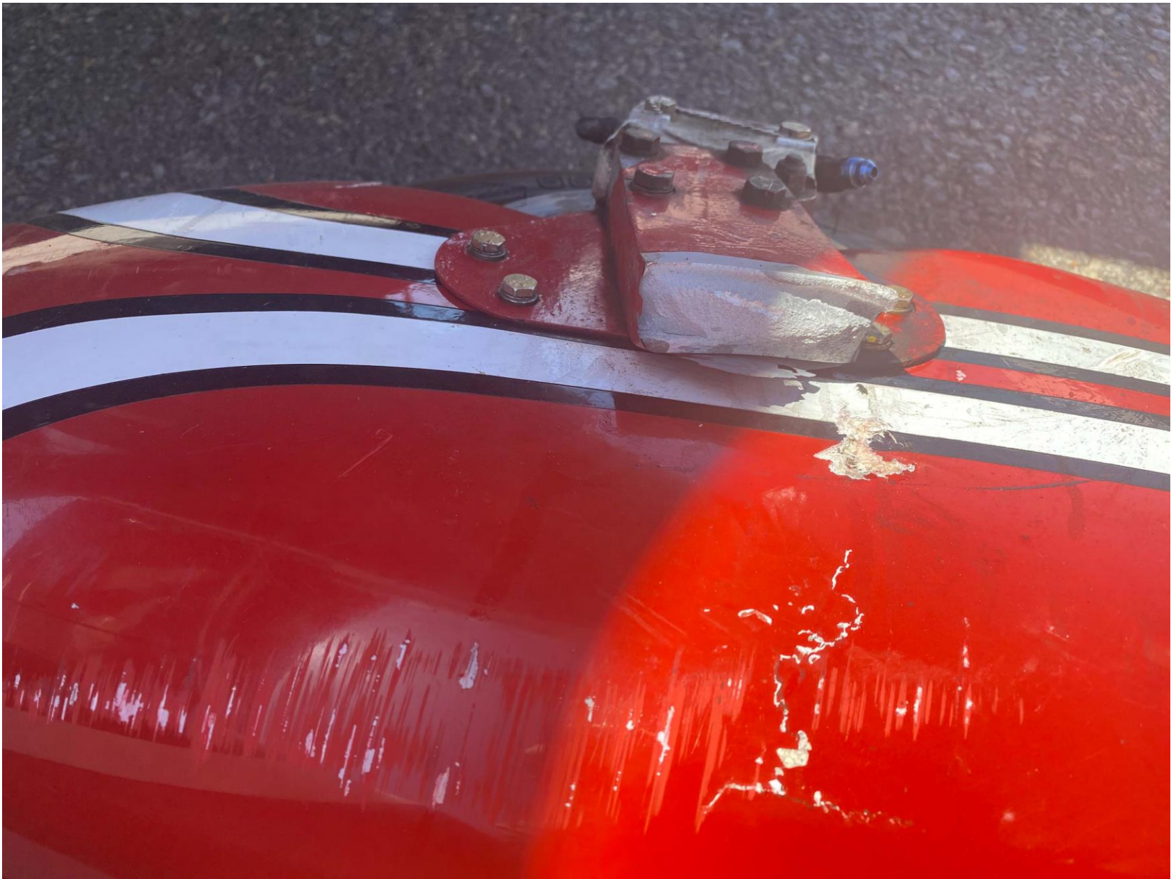
Photo 6 - Accident site, wheel pant and strut separation surface. (Courtesy of the FAA)
