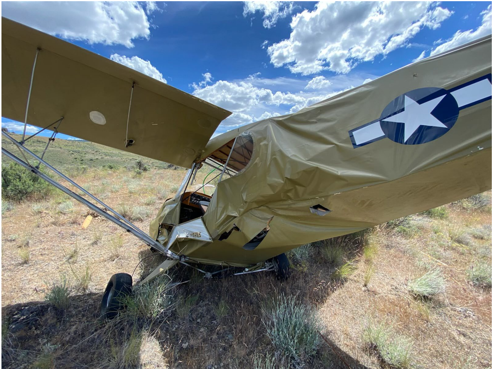
Photo 2 – N15MF, showing substantial damage to the fuselage. Photo courtesy of the pilot.
