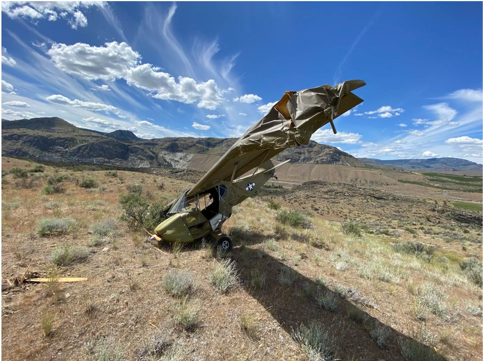
Photo 1 –N15MF, showing substantial damage to the left wing and fuselage. Photo courtesy of the pilot.
