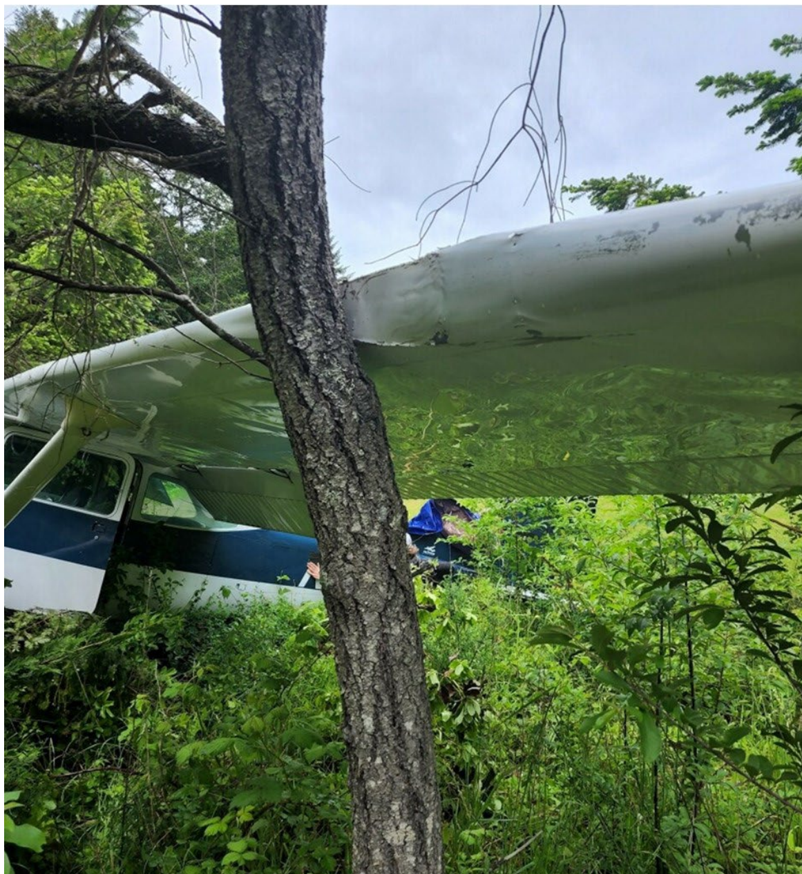
Photo 1 – Left wing damage (Photos courtesy of Operator)
