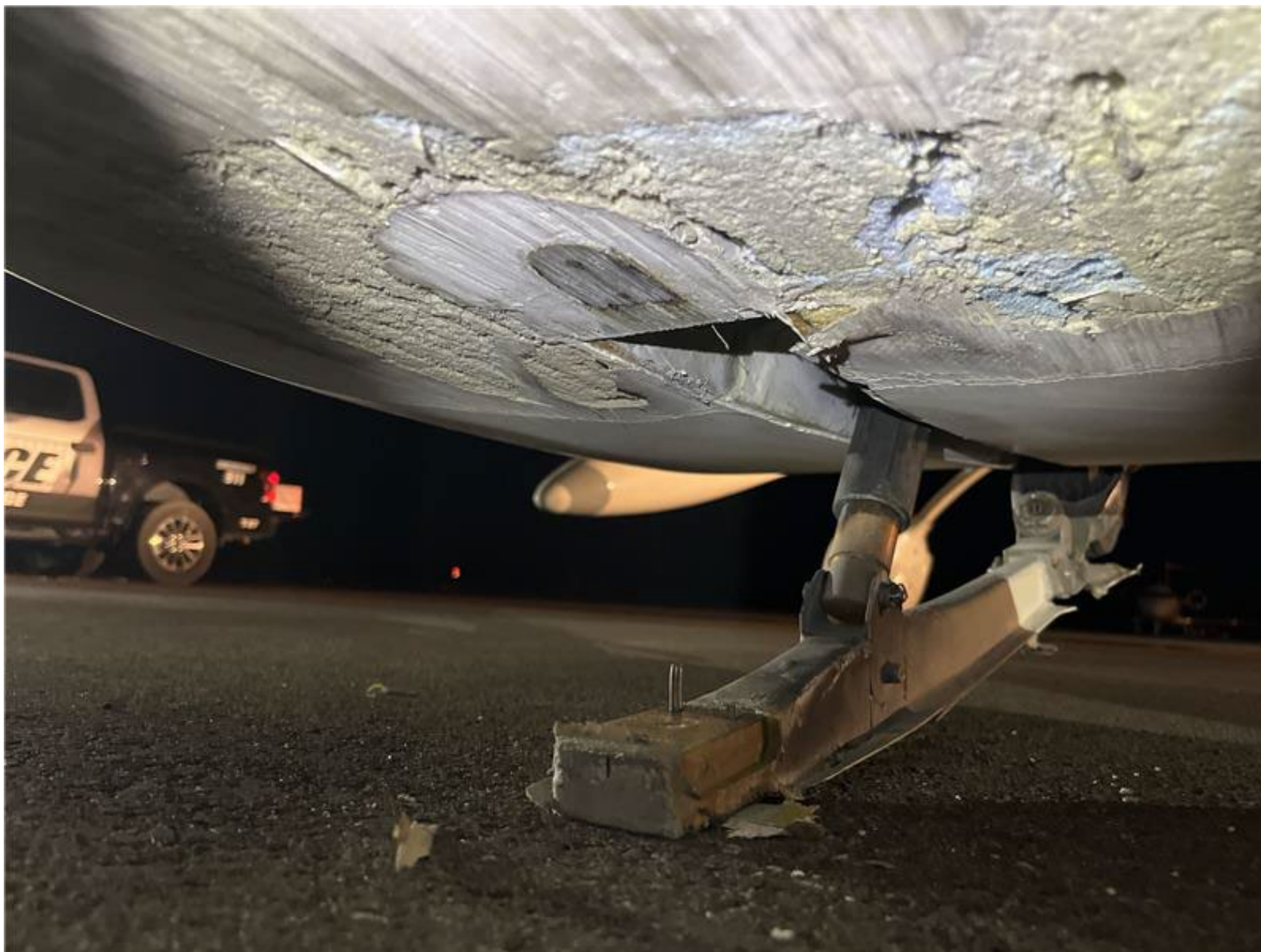
Photo 1 - View of Fuselage Damage (photo courtesy of pilot)
