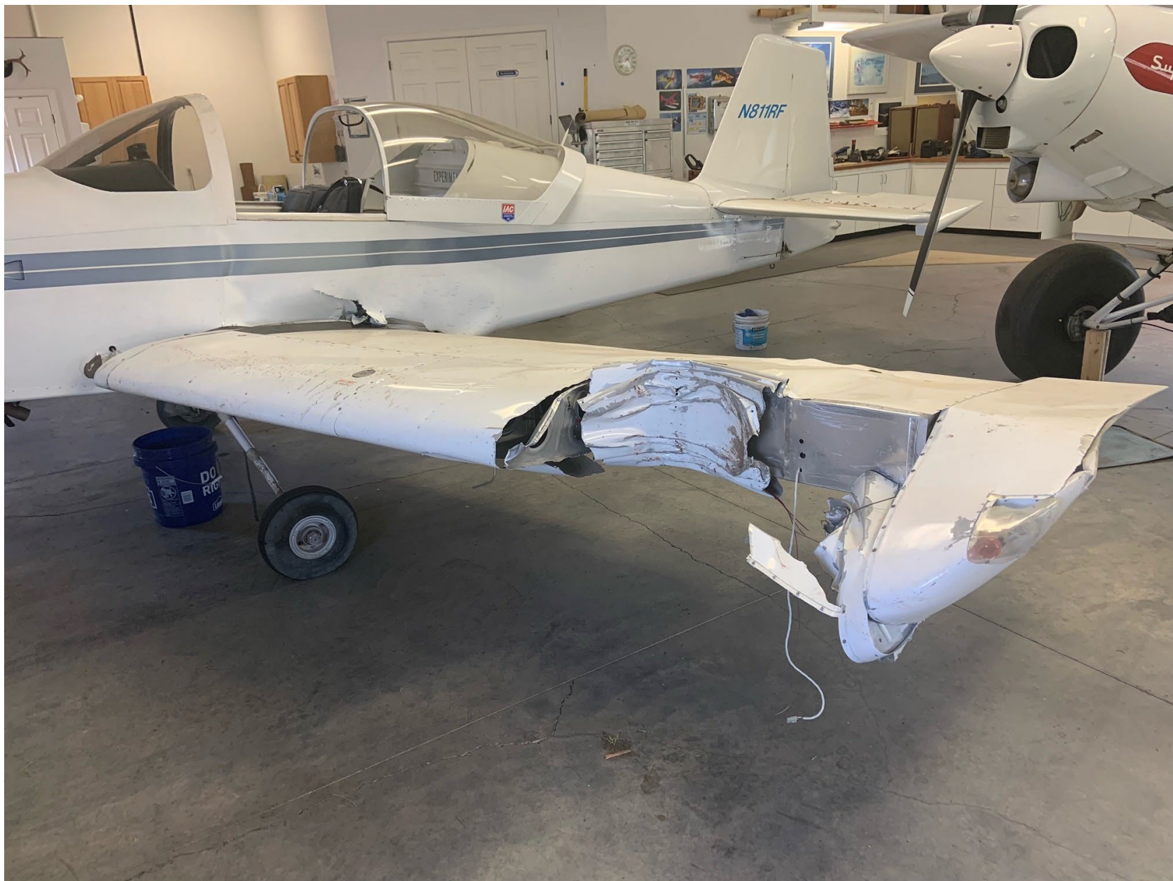
View of Left Wing Leading Edge Damage (Provided by Owner)
