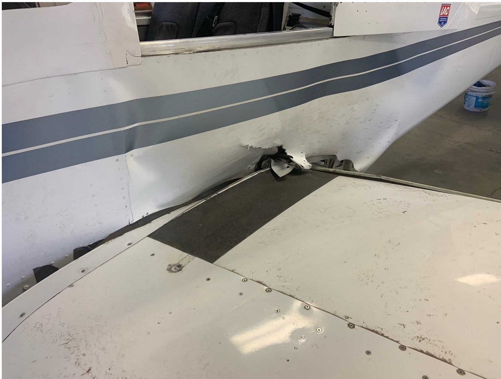
View of Fuselage Damage (Provided by Owner)
