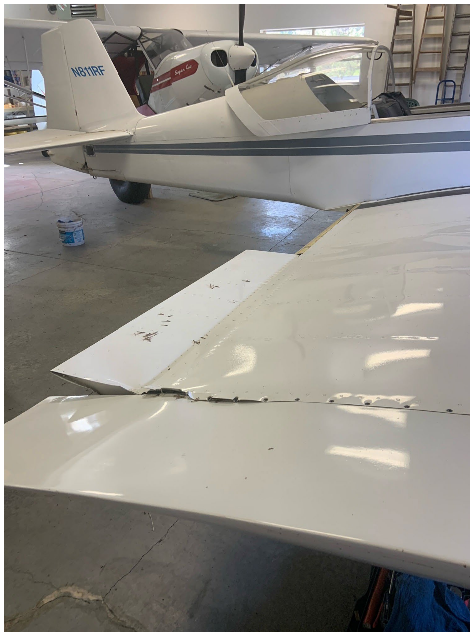
View of Right Wing Trailing Edge Damage (Provided by Owner)
