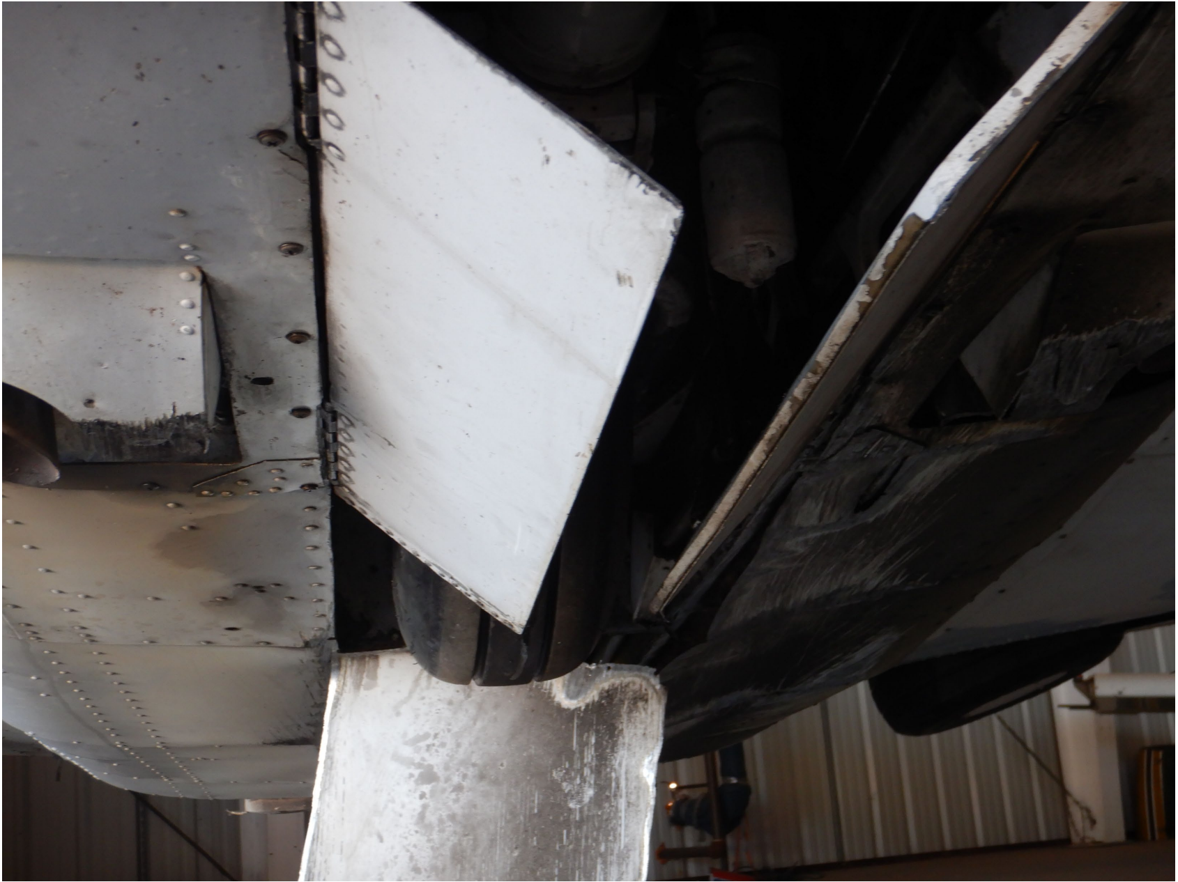
Photo 6 – Nose Gear (Partial Extension)
