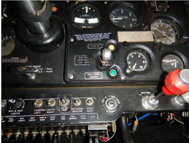
Figure 1 – Landing gear switch position
