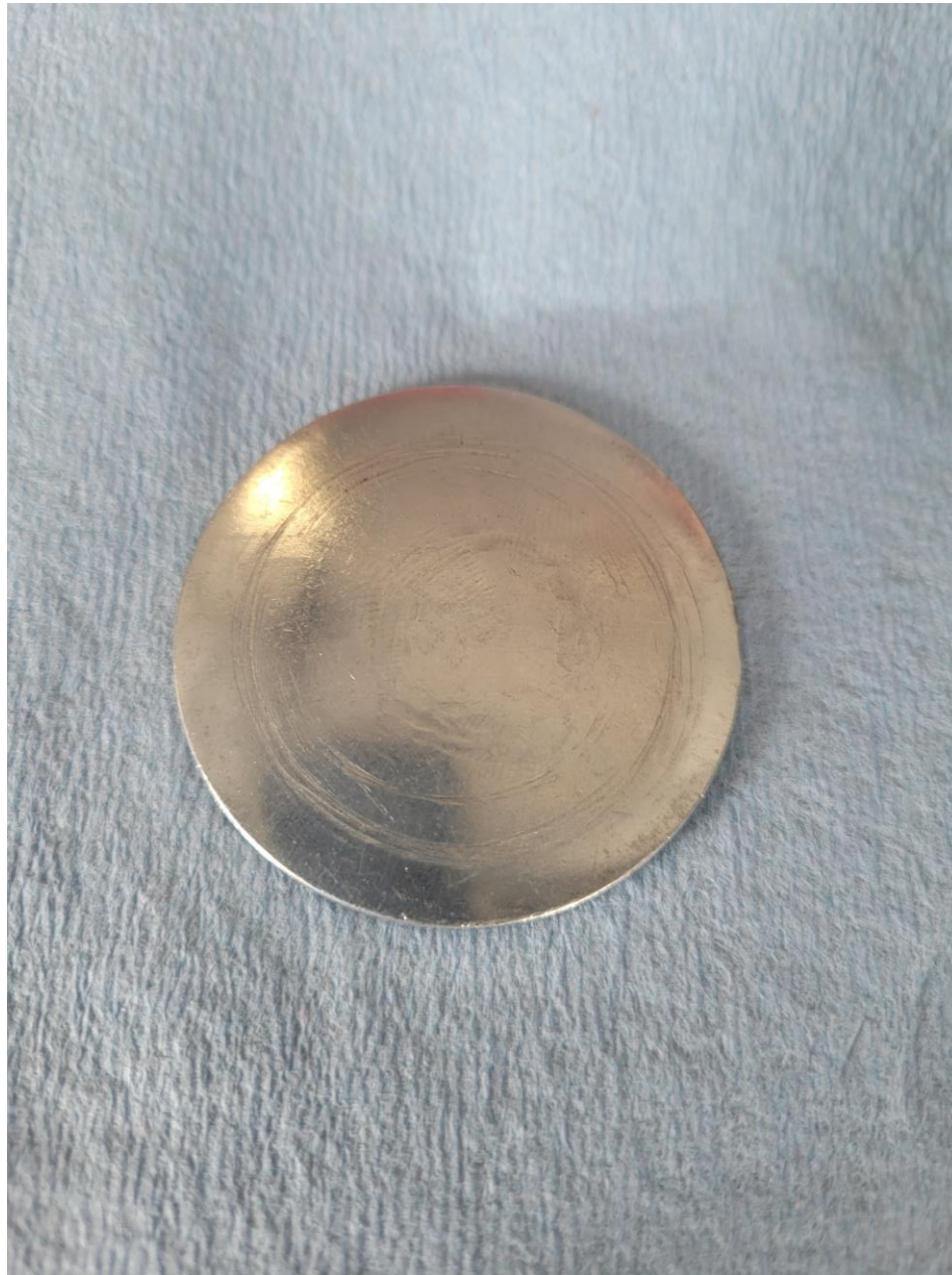
Photo 1 – Examination of the expansion plug. (Coursey of the FAA)
