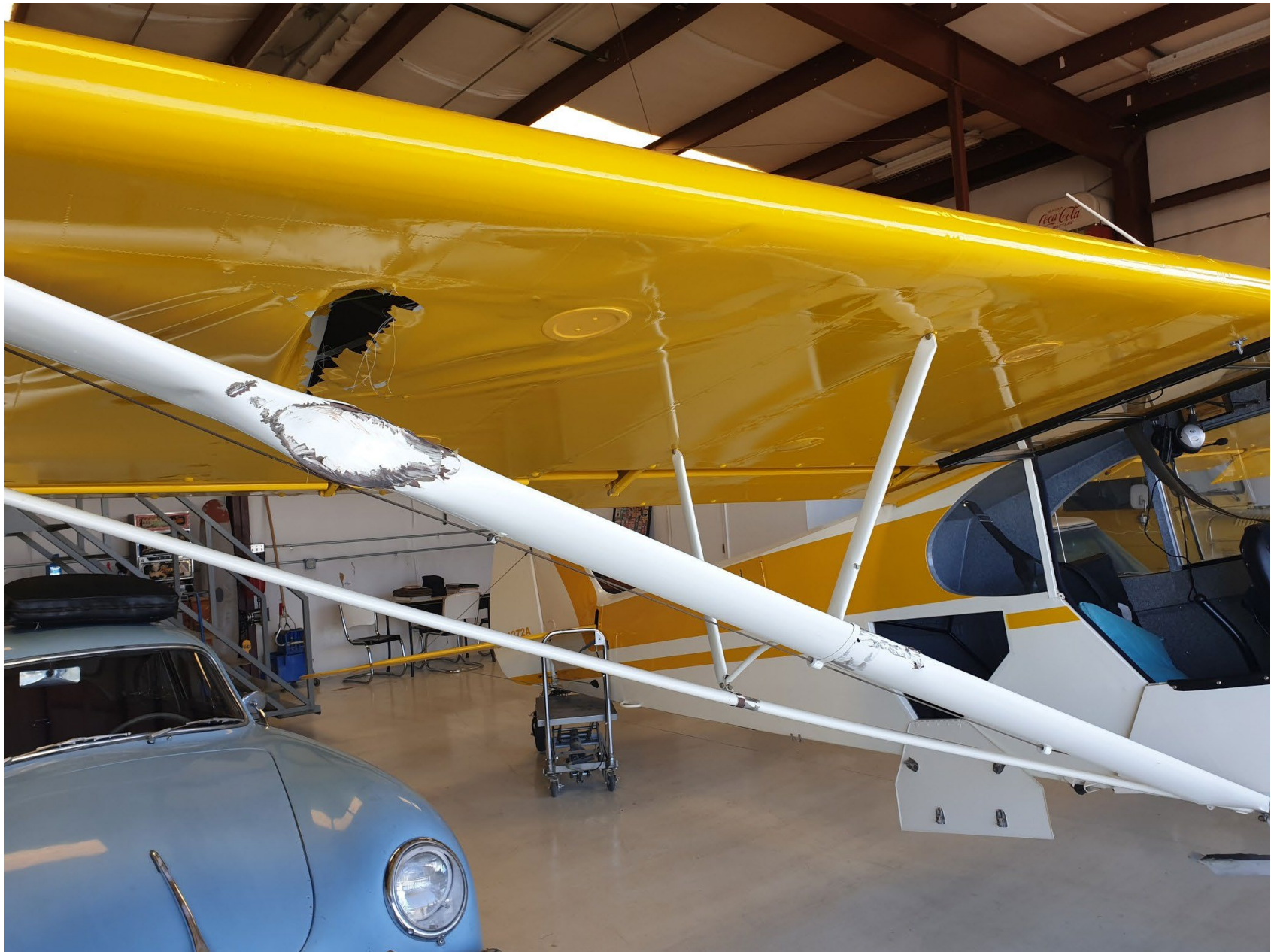
View of right wing strut damage (photo courtesy of pilot)
