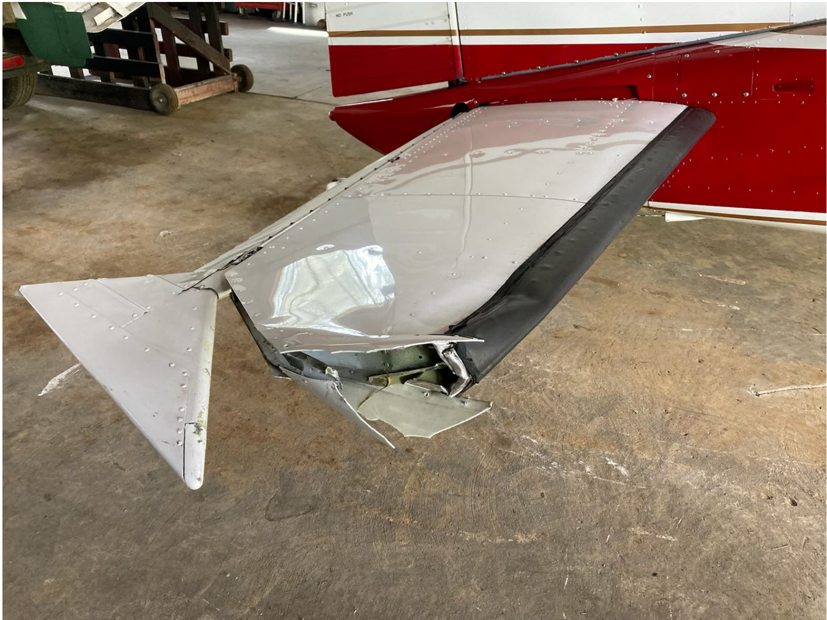
View of right side elevator damage (photo courtesy of pilot)
