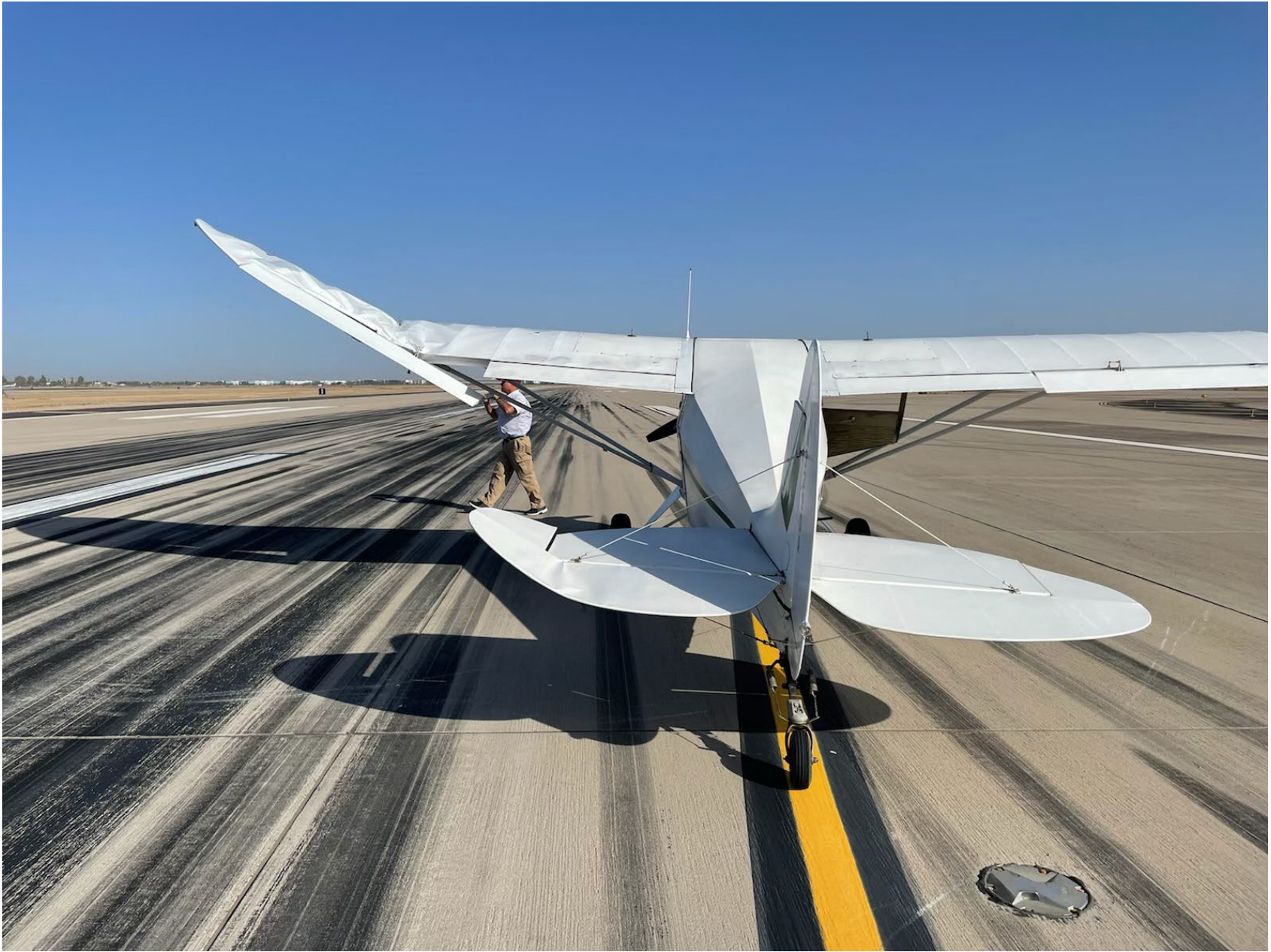
Photo 1 – Left wing and elevator damage. (Photo courtesy of pilot)
