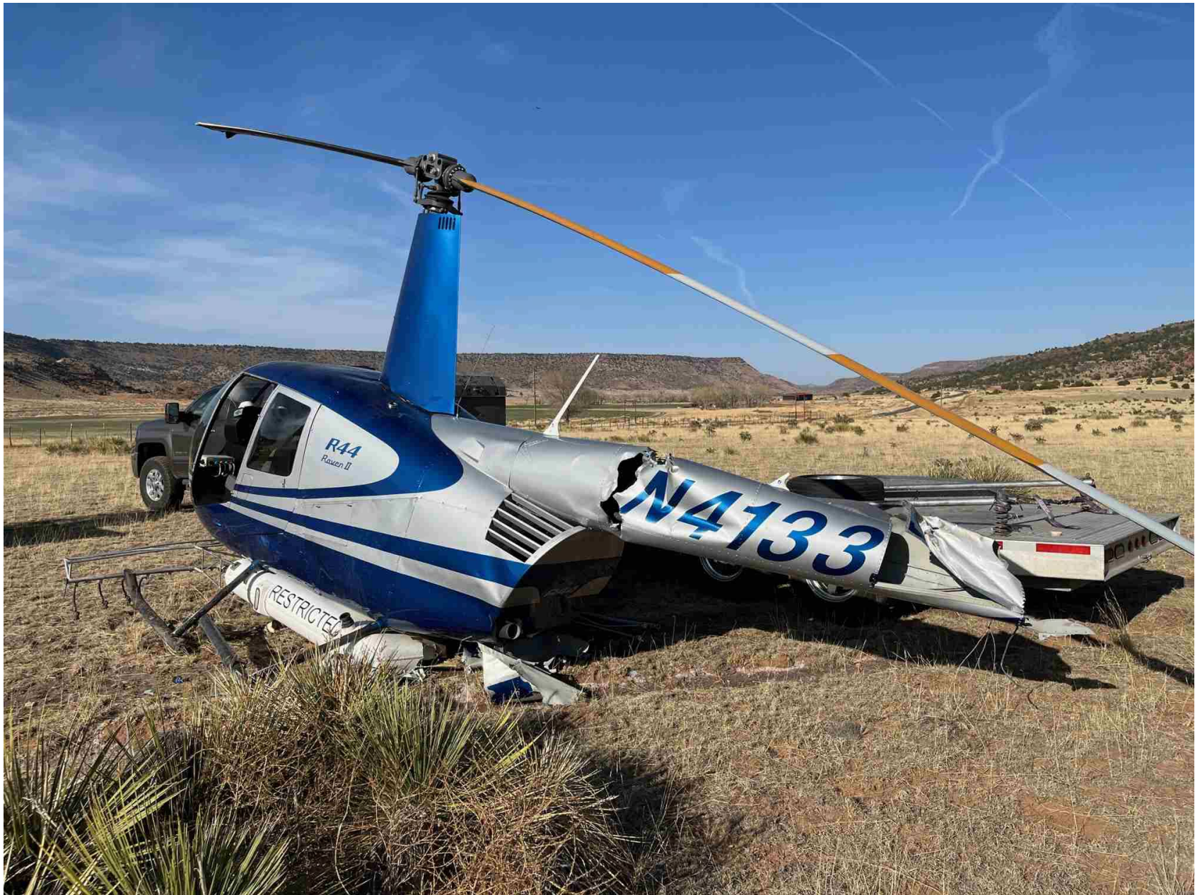
Photo 1 – View of tailboom damage (photo courtesy of the operator)
