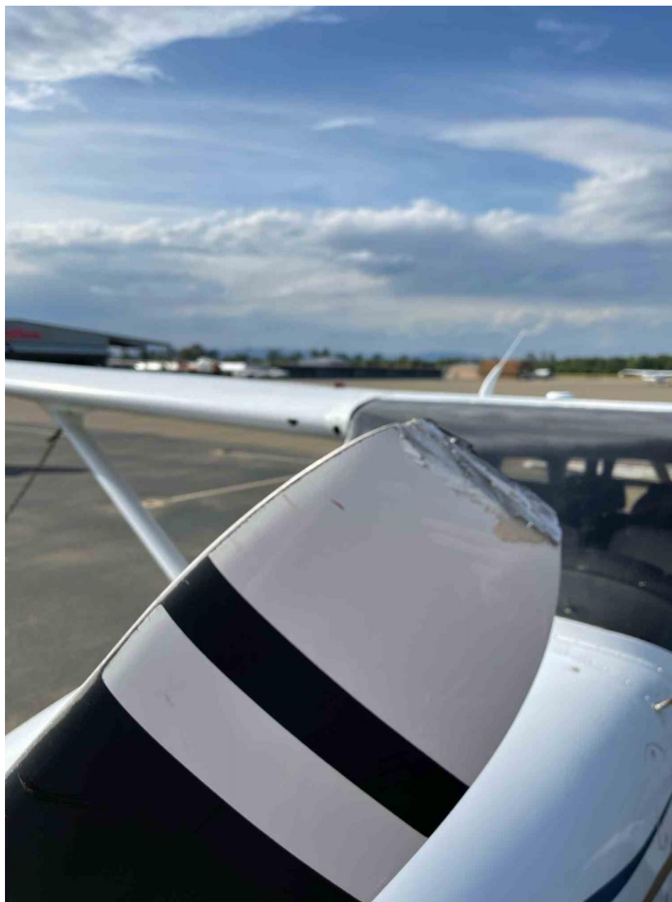
Photo 1 – Accident airplane, propeller strike. (Courtesy of the operator)
