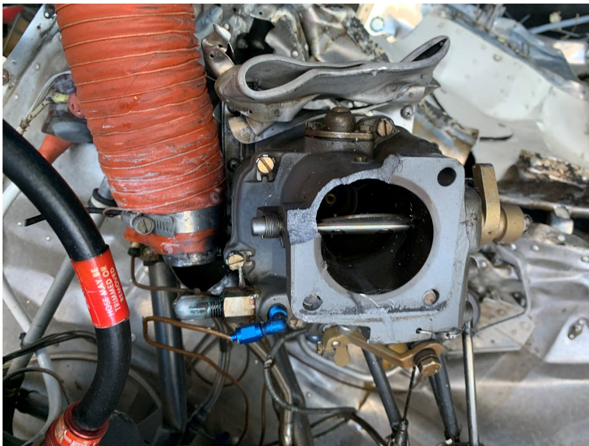
Photograph 3 - View of separated carburetor from impact damage
