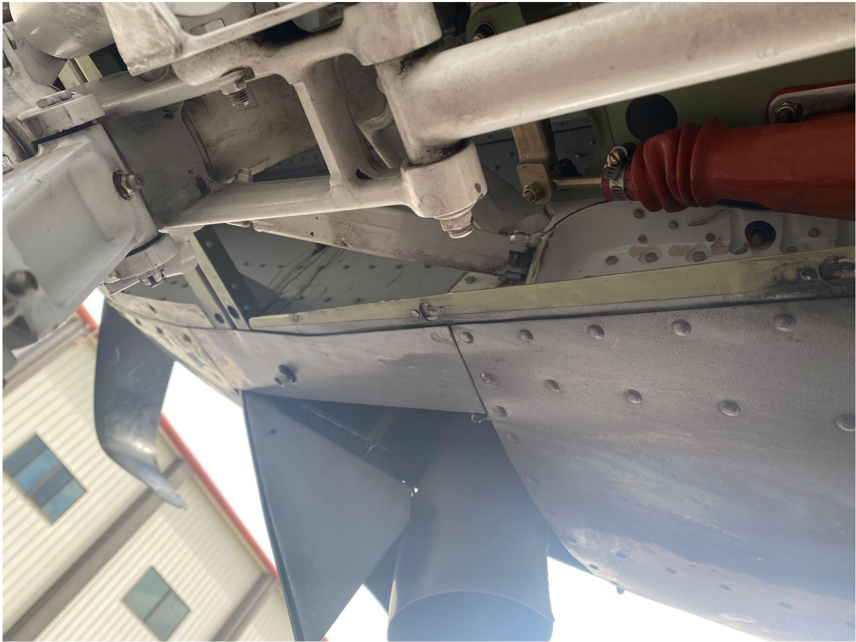
Photo 2 – View of the nosewheel trunnion area and steering link rod. Courtesy of the FAA.
