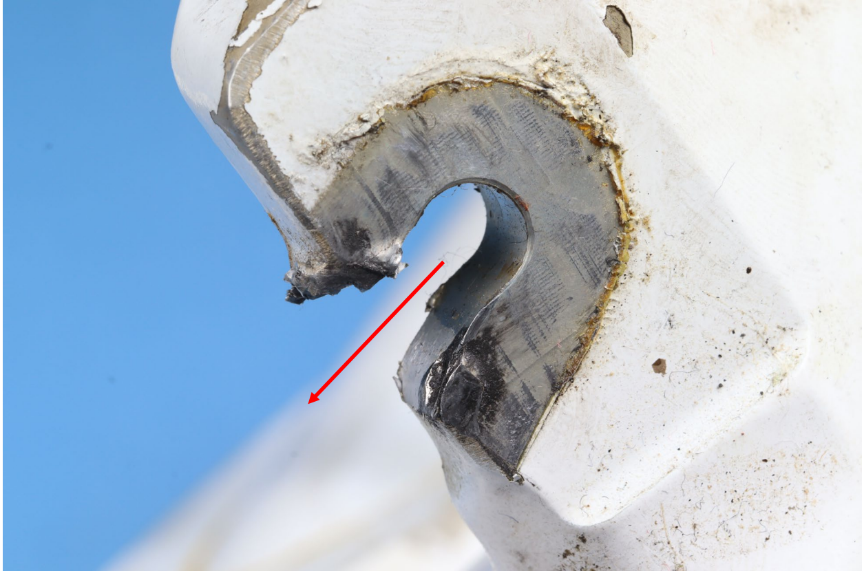
Figure 5. Tear out of bolt hole. Red arrow depicts direction of force.
