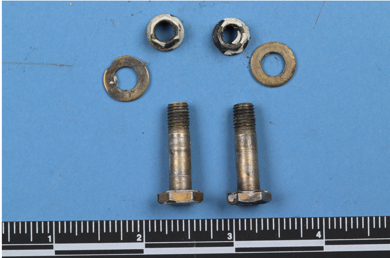
Figure 4. Brace attachment hardware exhibiting a slight bend.
