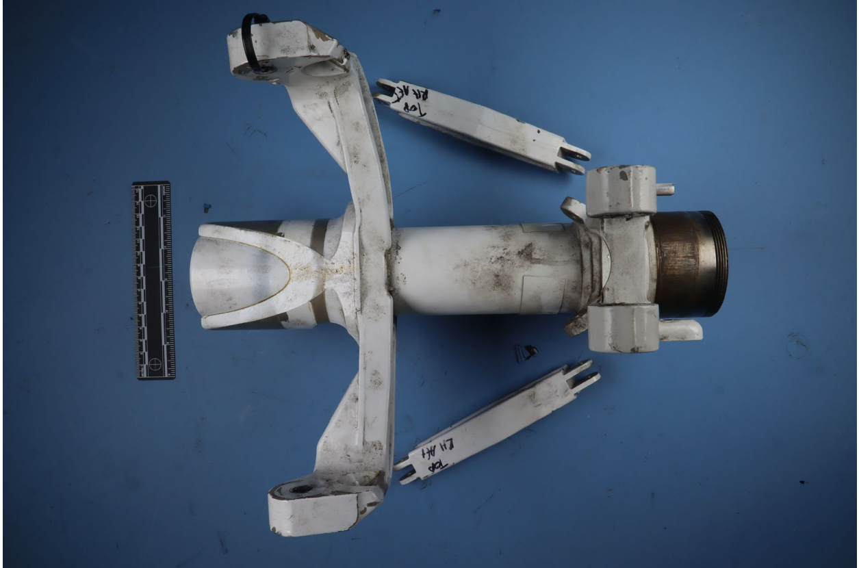
Figure 1. Upper nose gear shock strut with upper and lower trunnions and braces as received.
