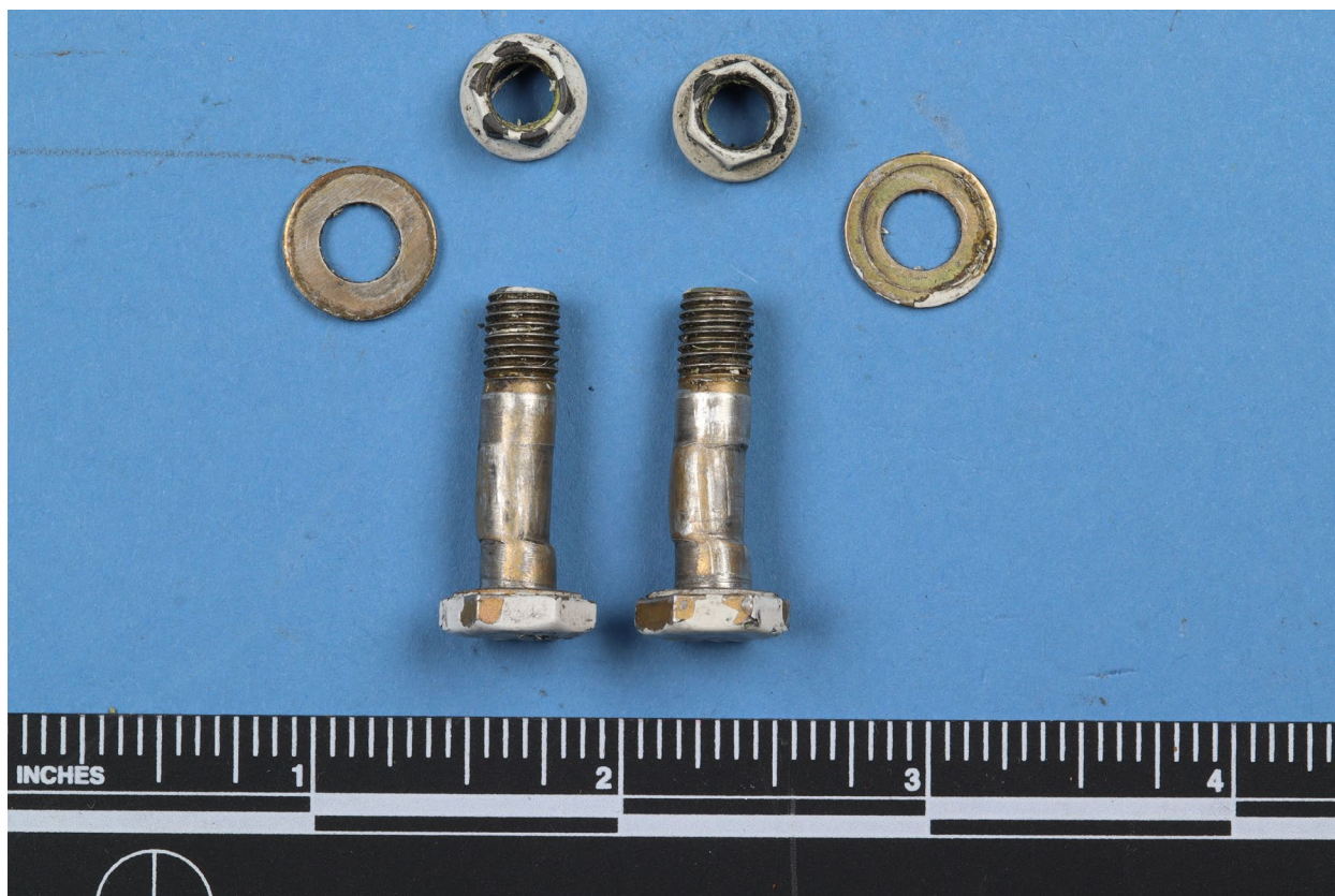
Figure 3. Brace attachment hardware exhibiting gross plastic deformation.
