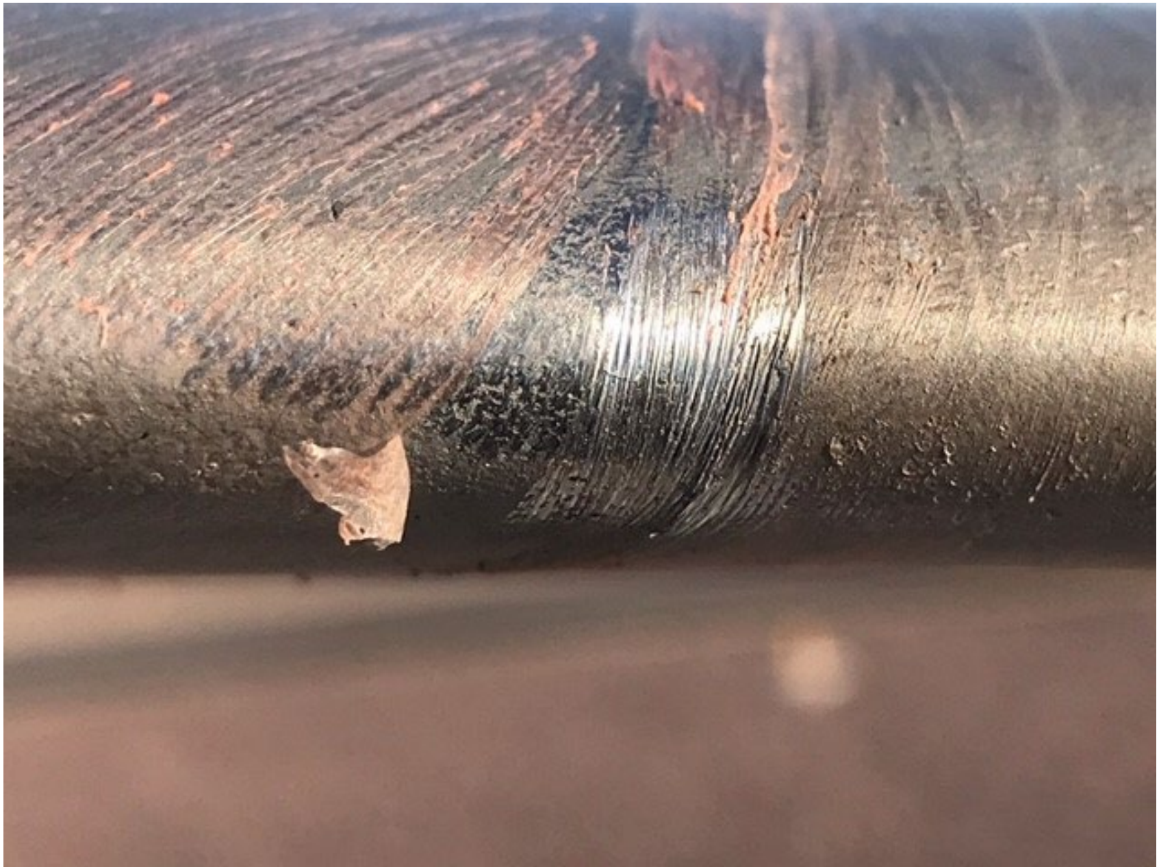
View of Main Rotor Damage (Source Unknown)
