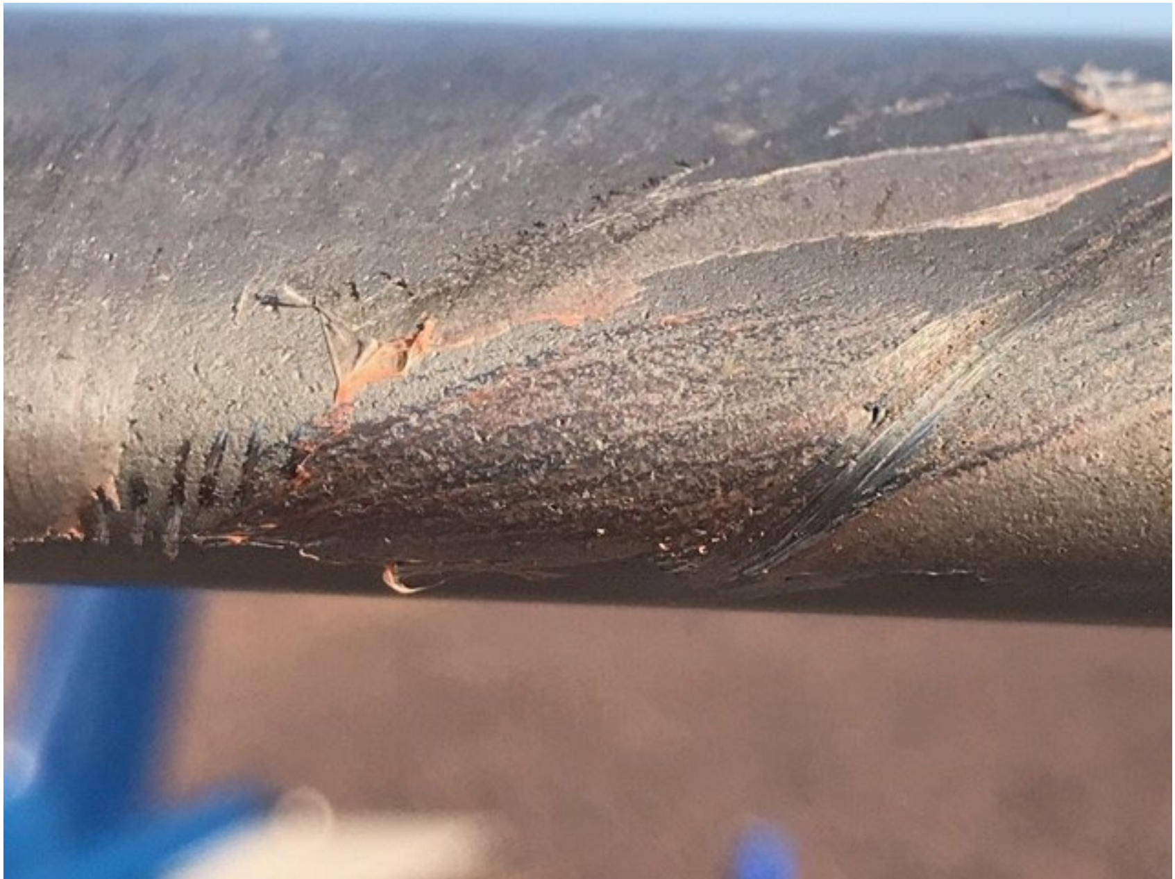
View of Main Rotor Damage (Source Unknown)
