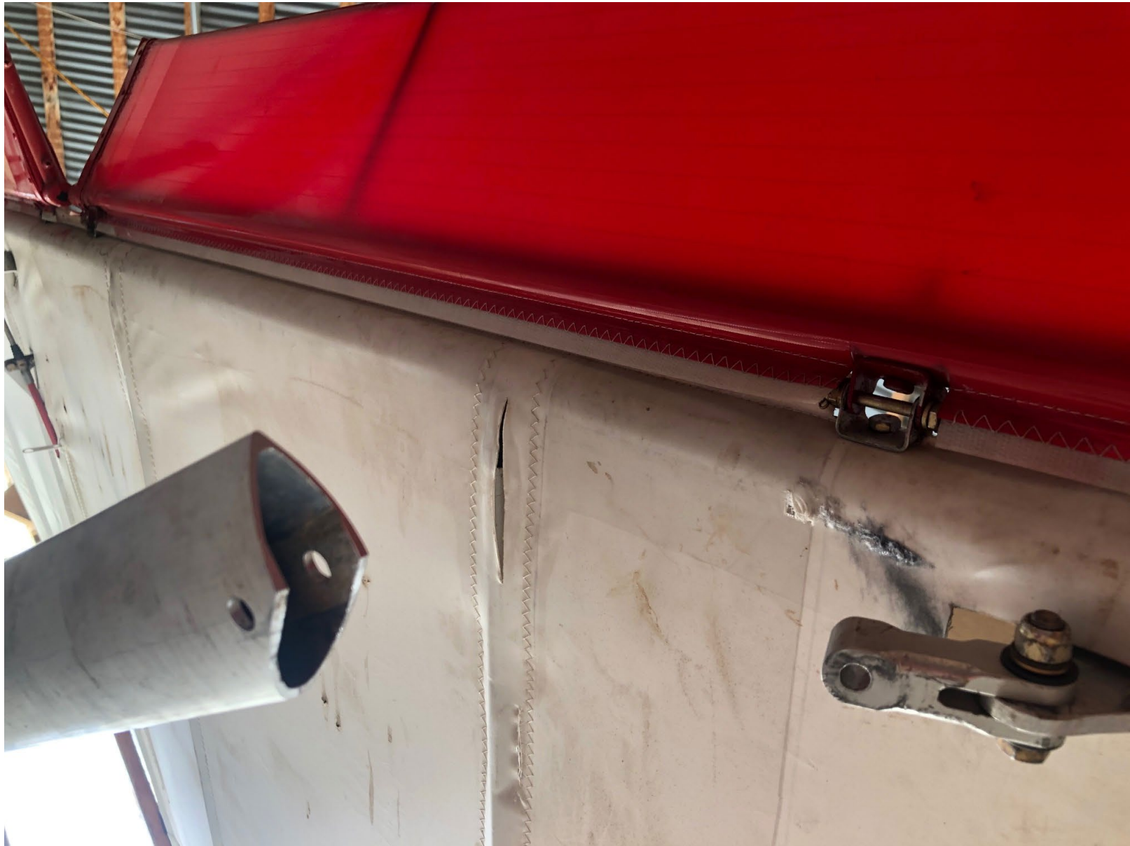
Photo 3 – View of right wing aft strut and attachment clevis (courtesy of accident pilot)
