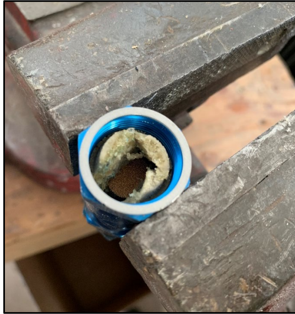
Figure 3: Material that clogged and surrounded the left fuel filter.
