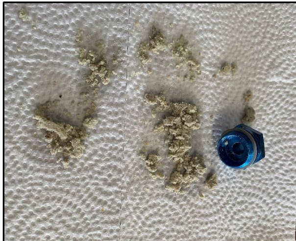
Figure 4: Material found inside the left fuel filter cover as viewed from the top.
