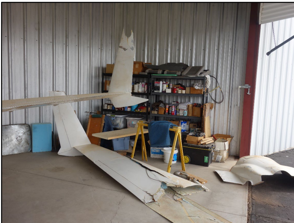
Figure 2: View of the portion of the left wing that separated.
