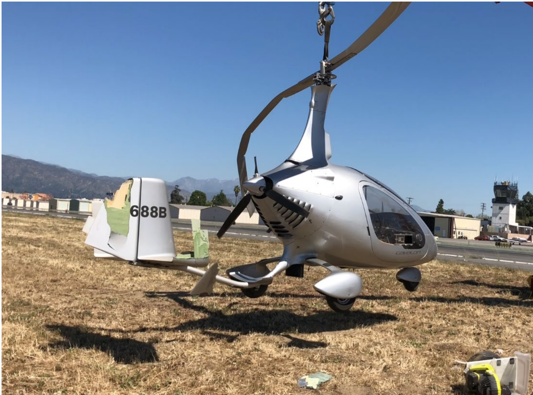
Photo 1 –View of damages to stabilizer and rudder (photo courtesy of pilot)
