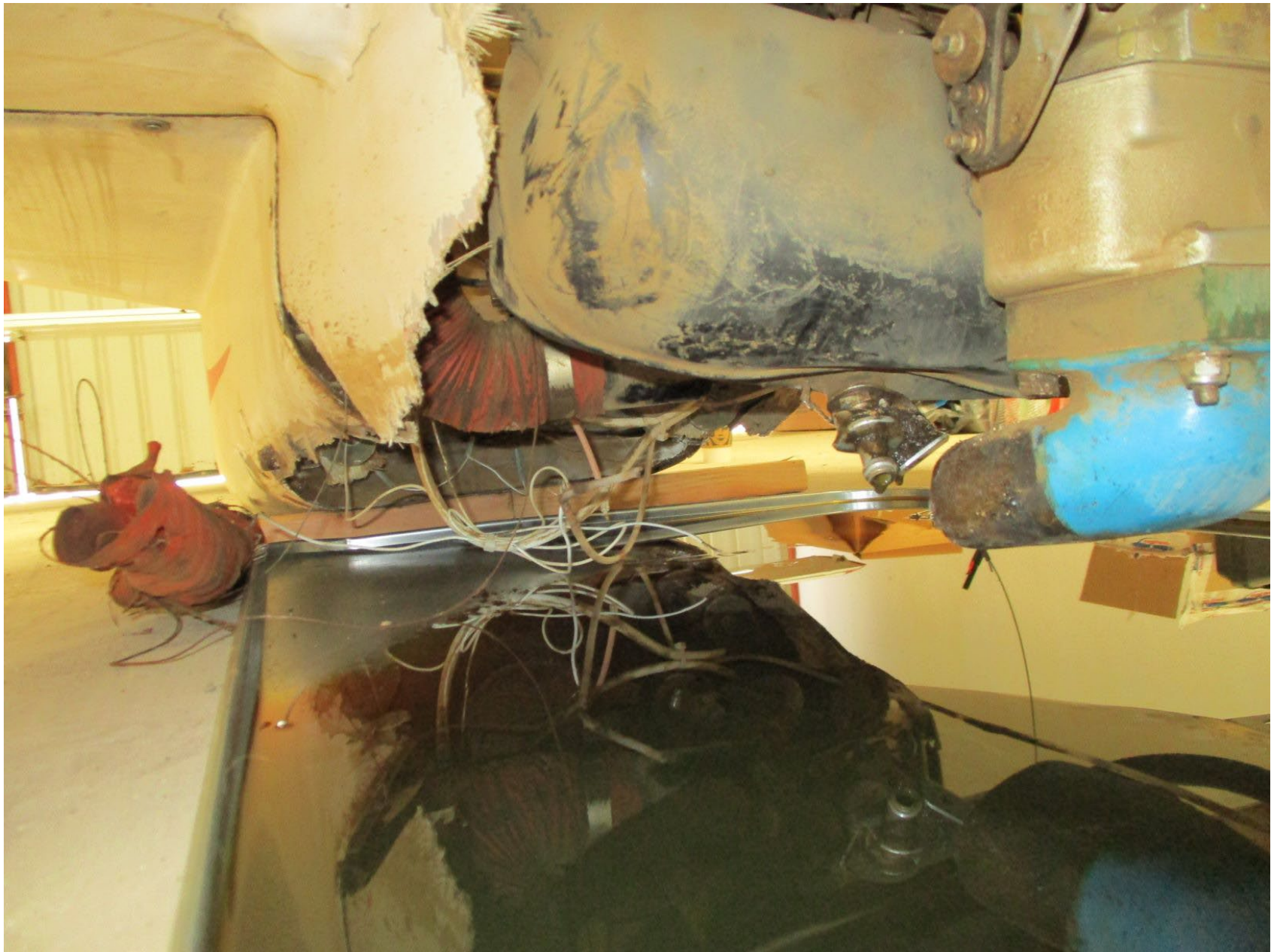
Photo 3 - Rear view of fuselage undercarriage damage (photo courtesy of the FAA)
