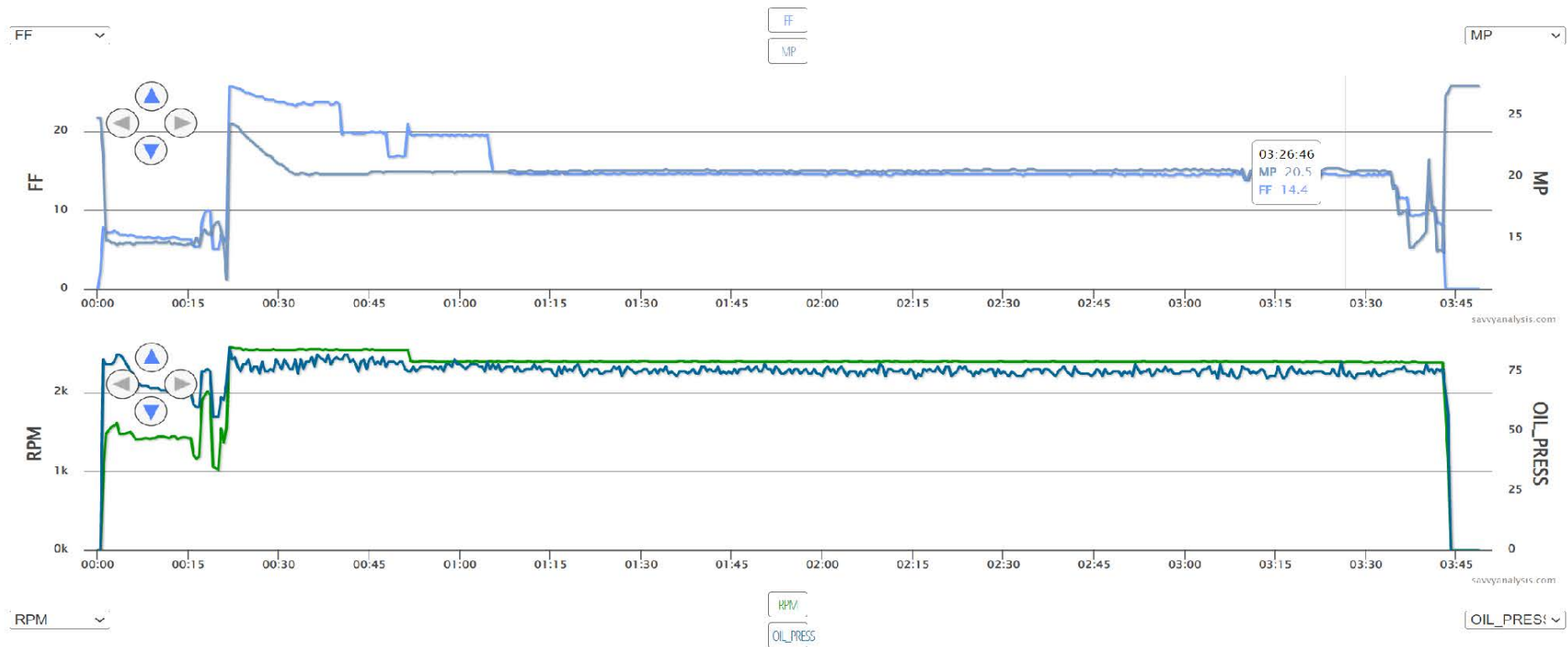
Figure 3-Accident flight data-fuel flow, manifold pressure.
