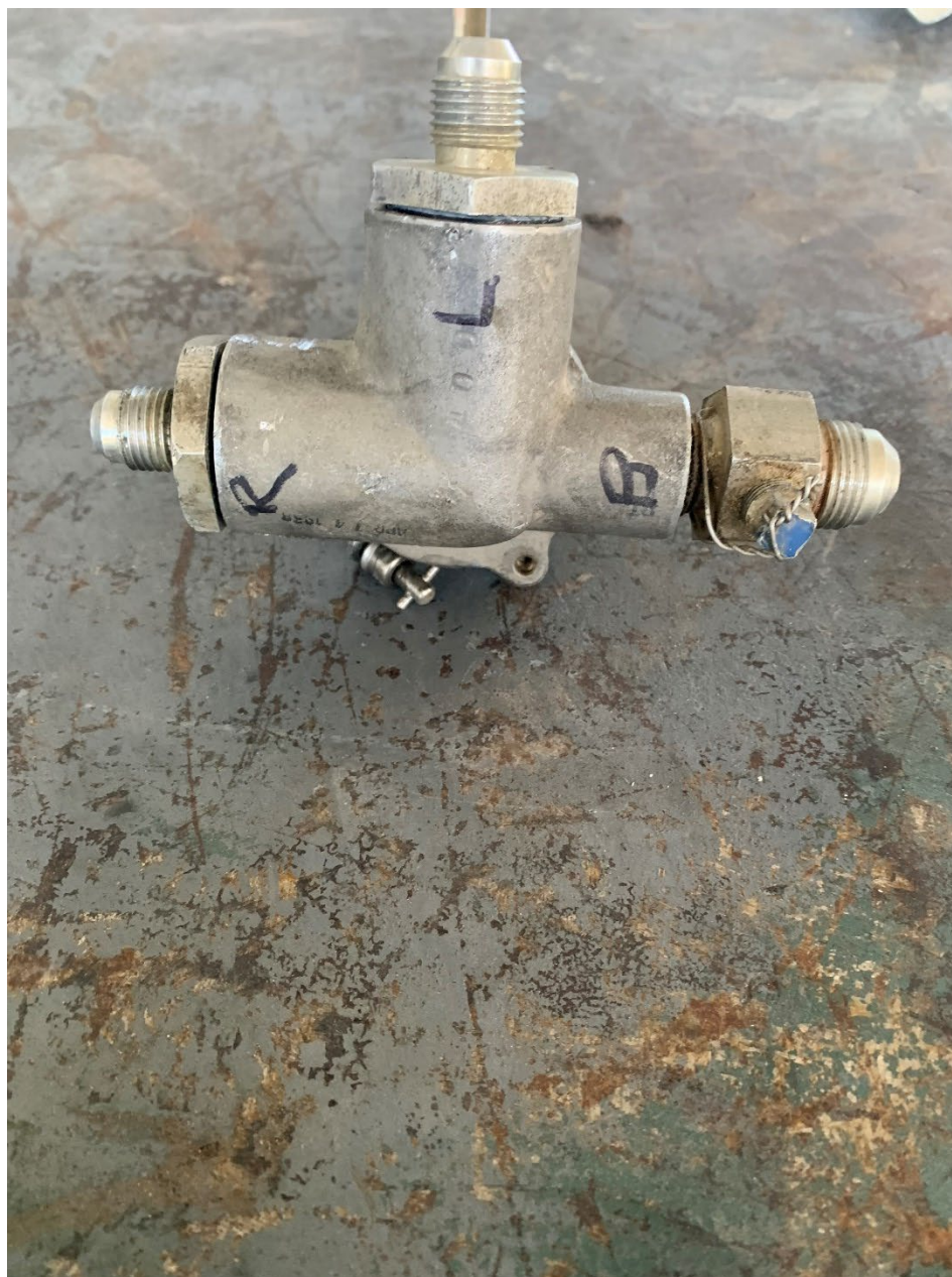
Photo 4 – View of N8814X fuel selector and valve post-accident examination (Courtesy of FAA)
