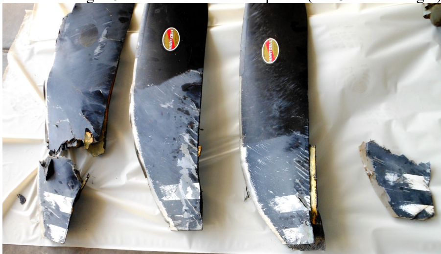
Photo montage #5 – Camber side blade tip area (1-4-3-2 left-to-right)
