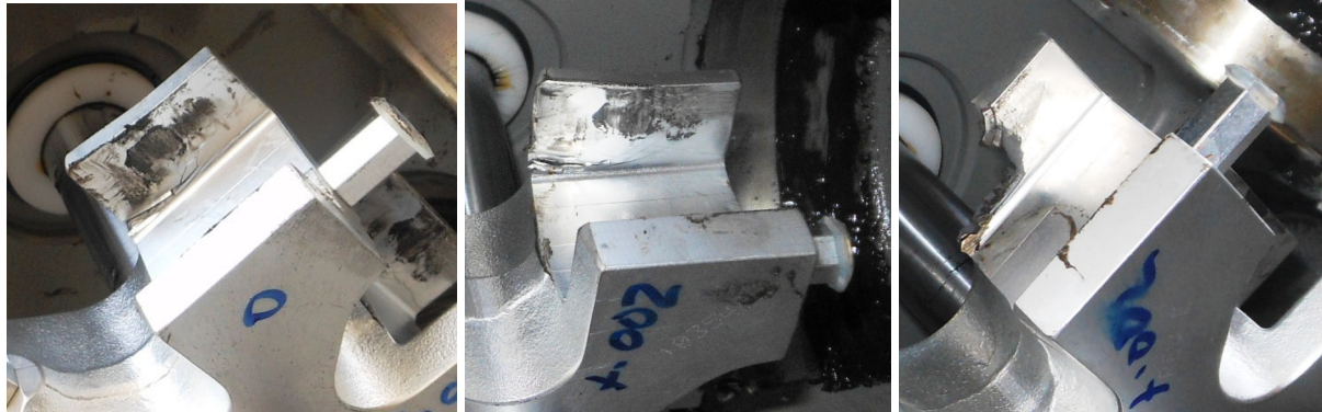
Photo montage #3 – Fractured fork tangs montage
