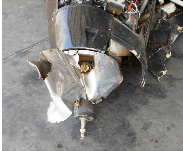
Photo #1 – Propeller as-presented for examination
