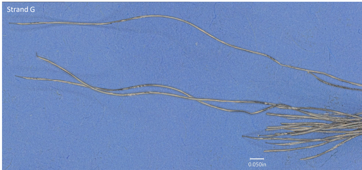
Figure 7. Digital microscope image of the left side forward rudder cable piece (see Figure 1) showing the fractured wire ends in strand G.
