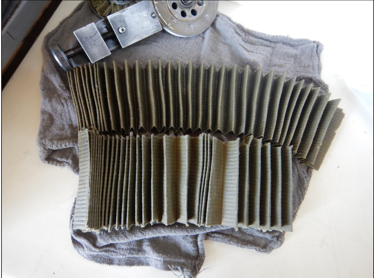
Figure 4-Disassembly of the oil filter.
