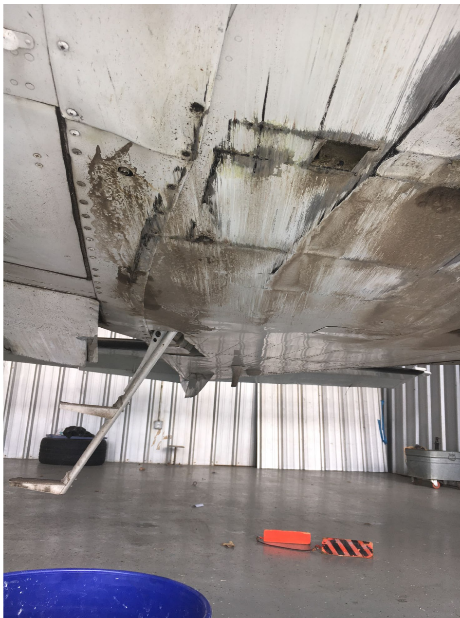
Photo 1 – View of substantial damage to lower fuselage (courtesy of FAA)
