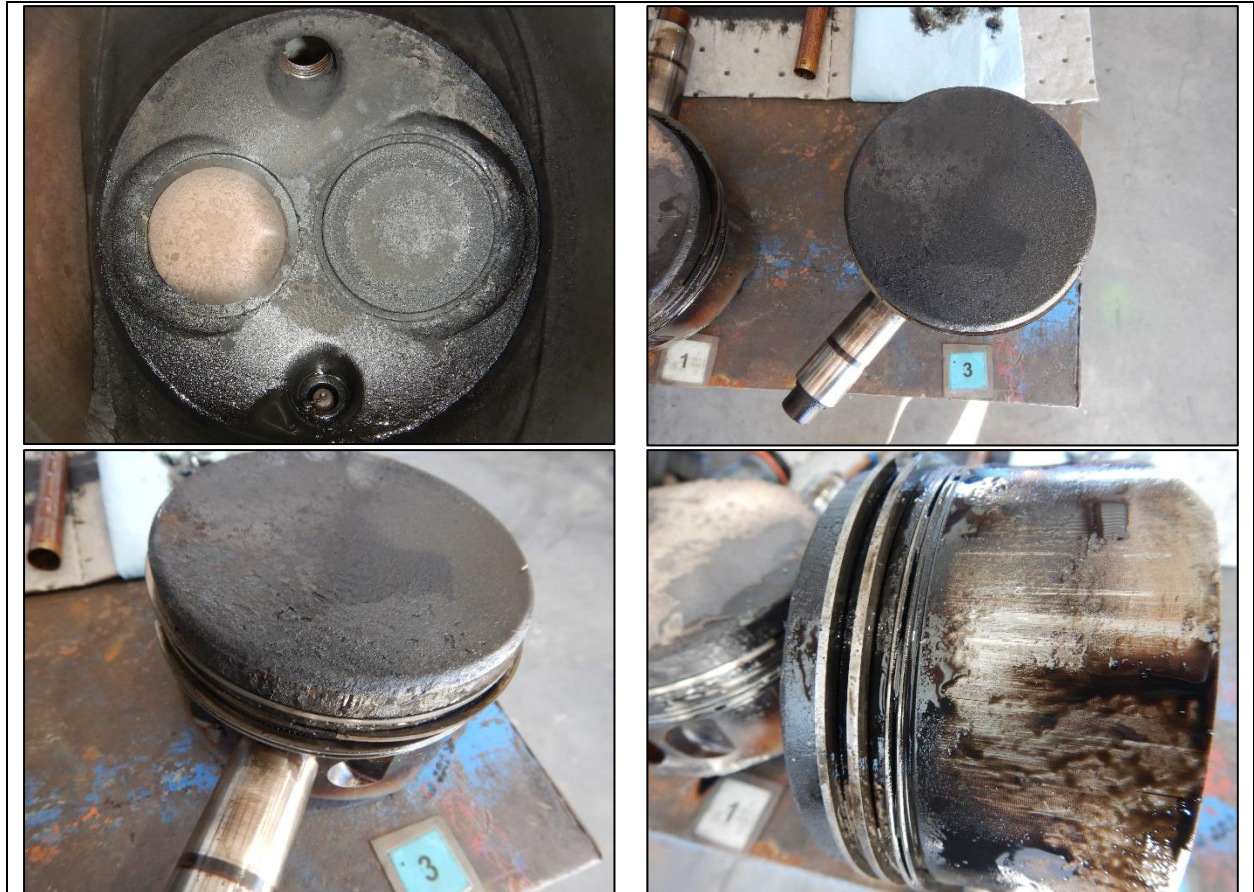
Figure 10-No. 3 Cylinder combustion chamber, piston head and rings.
