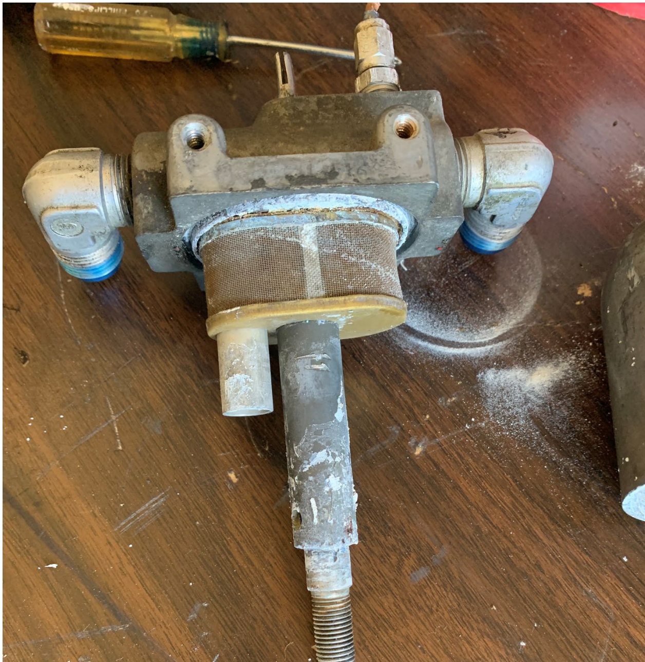
Photo 5 – View of the gascolator standpipe, and fuel filter screen containing rust and corrosion substance with vivid fluid line corrosion (NTSB IIC)
