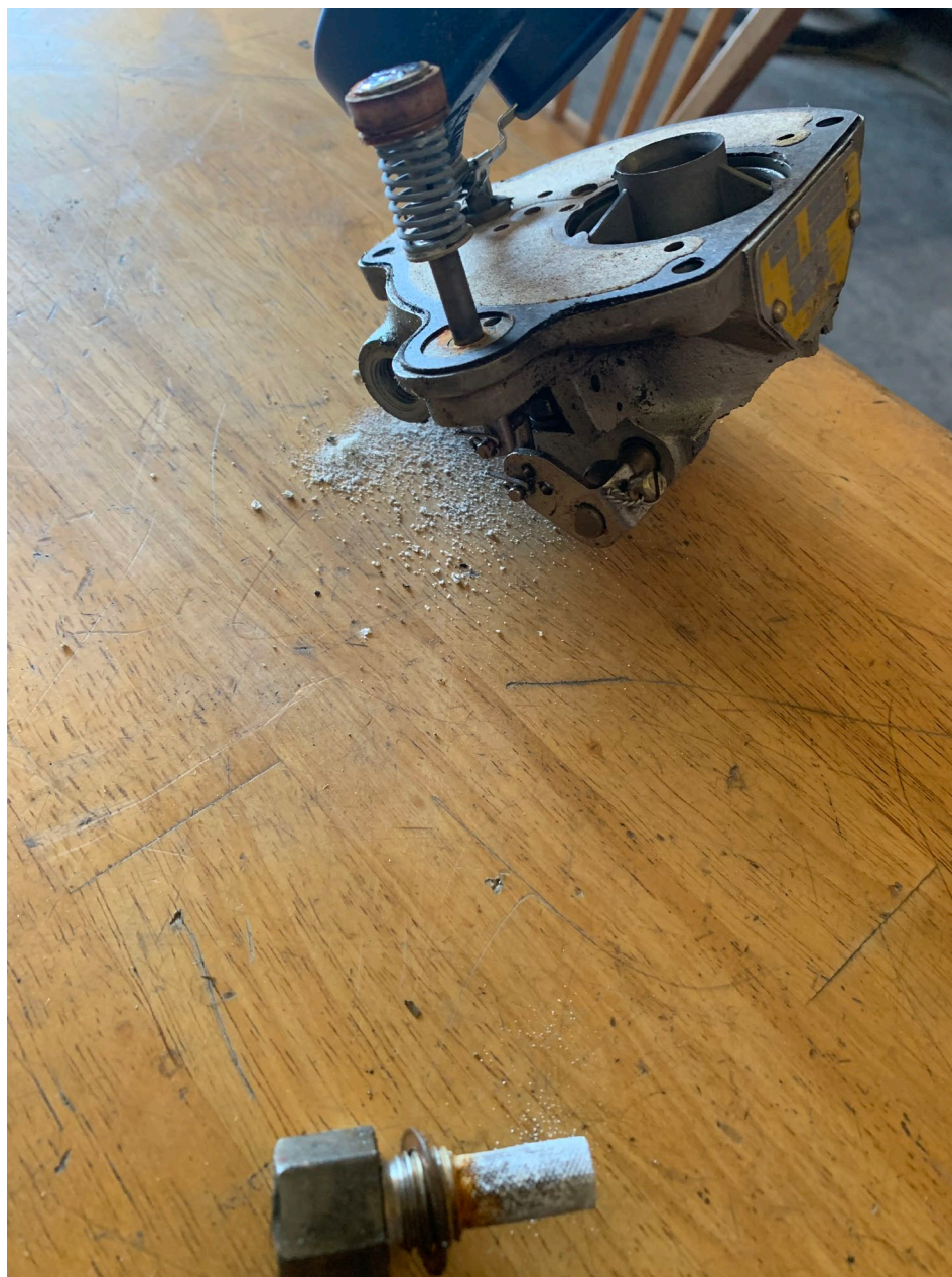
Photo 10 – View of the rusted carburetor fuel inlet screen encapsulated with the corrosion substance and about ½ teaspoon of extracted corrosion substance from the fuel inlet screen and housing (NTSB IIC)
