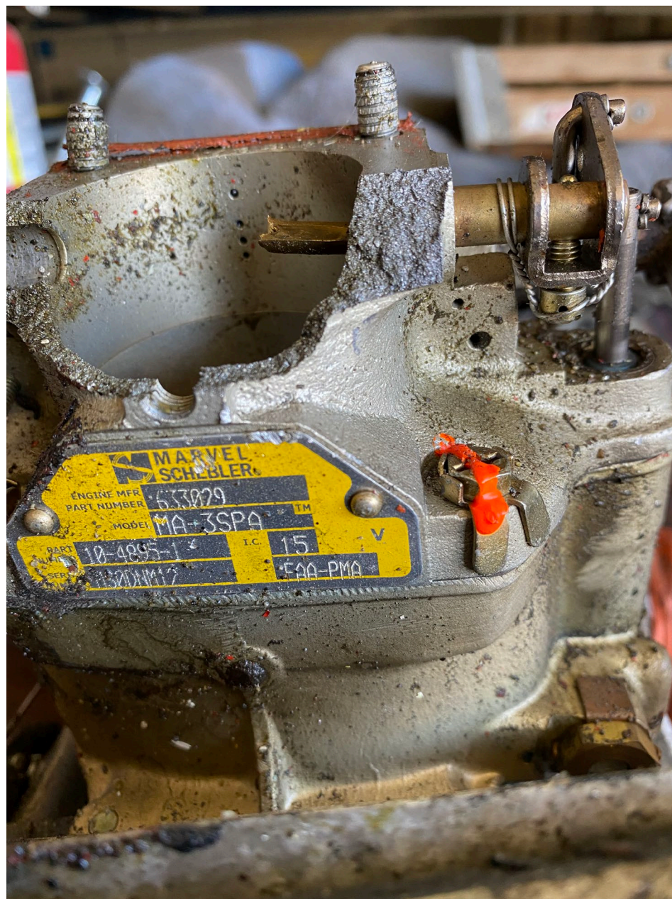
Photo 6 – View of impact damaged carburetor before disassembly (NTSB IIC)
