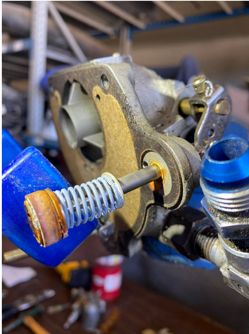
Photo 7 – View of the accelerator pump containing rust and corrosion substance (NTSB IIC)
