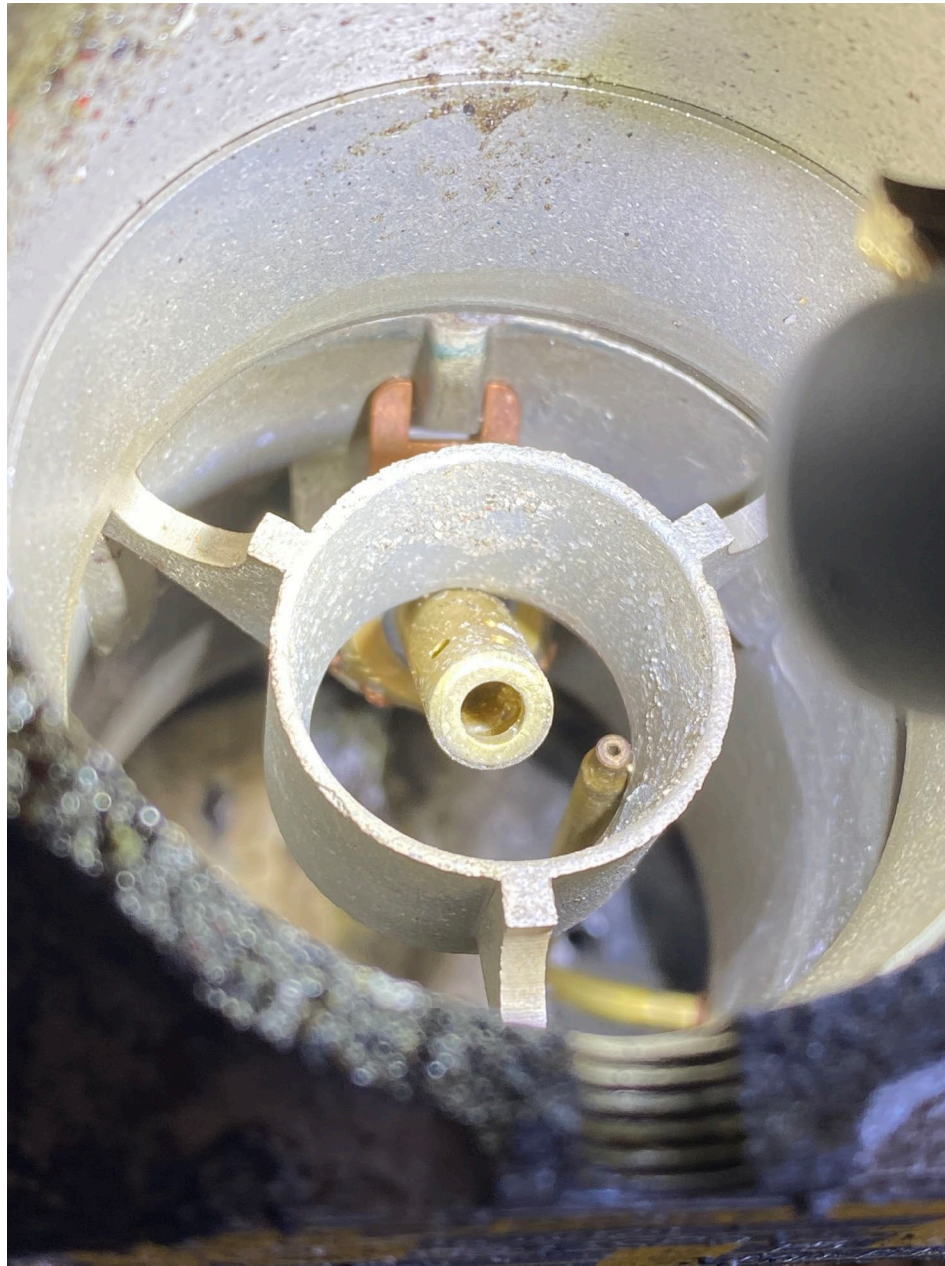
Photo 9 – View of the carburetor fuel nozzle pitting and the accelerator pump discharge tube containing corrosion substance (NTSB IIC)
