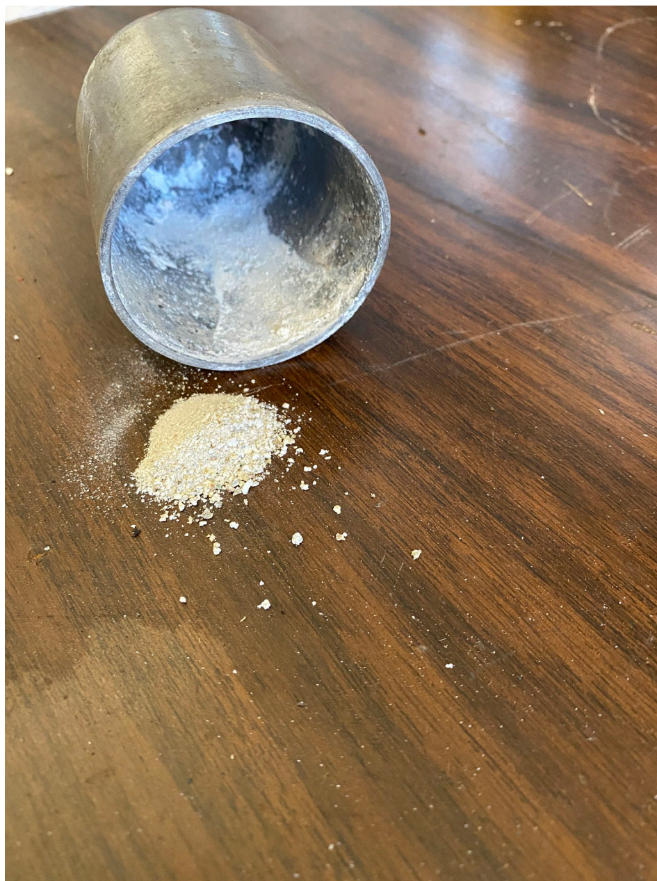
Photo 4 – View of the gascolator fuel bowl internal pitting and the granulated, white powder, corrosion substance (NTSB IIC)
