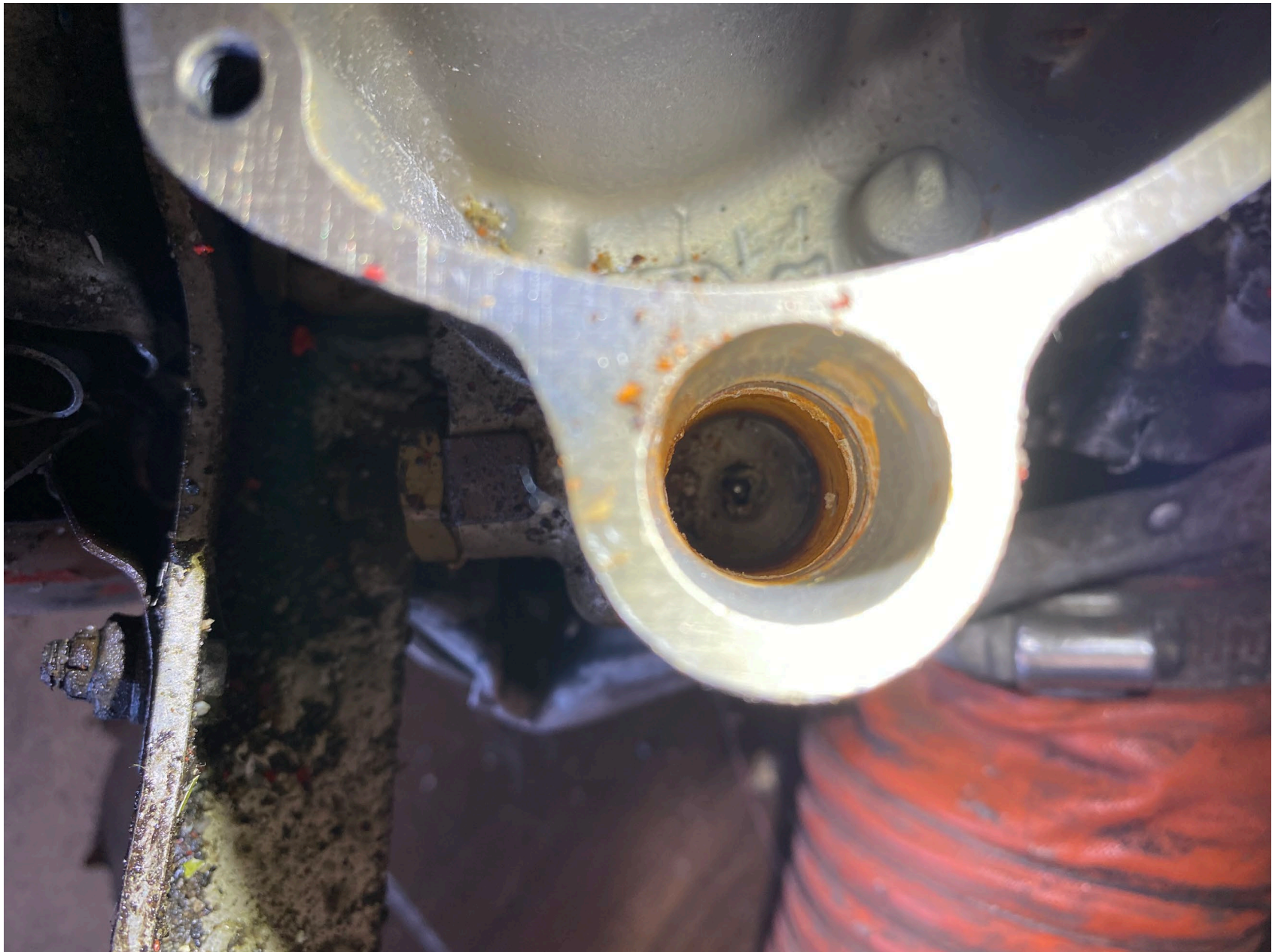
Photo 8 – View of the accelerator pump housing containing rust and corrosion substance (NTSB IIC)
