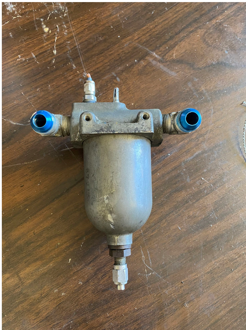
Photo 3 – View of the gascolator before disassembly (NTSB IIC)
