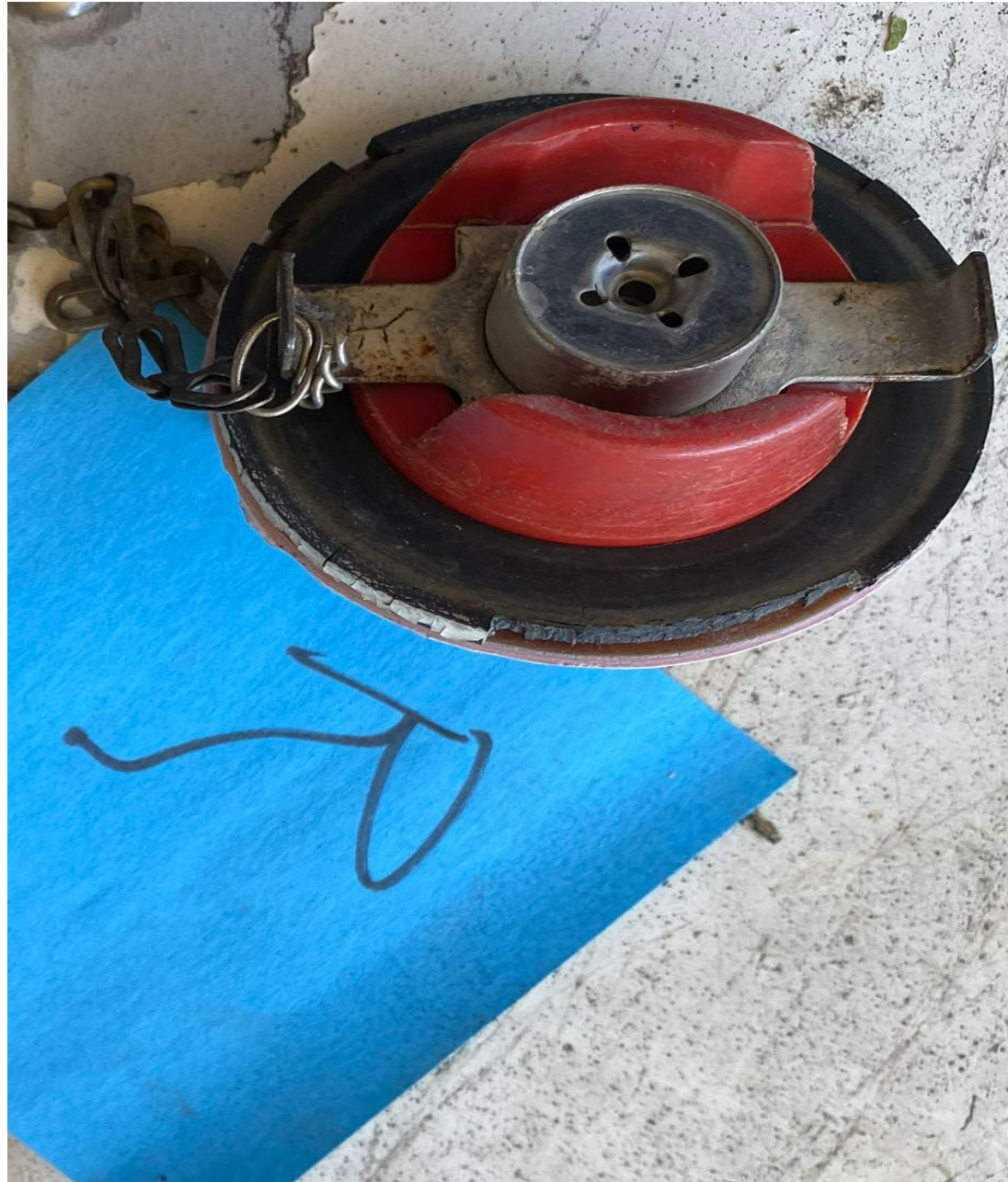
Photo 1 – View of the right wing tank fuel cap containing rust, missing silicone vent, and the deteriorated rubber gasket missing outer sections (NTSB IIC)
