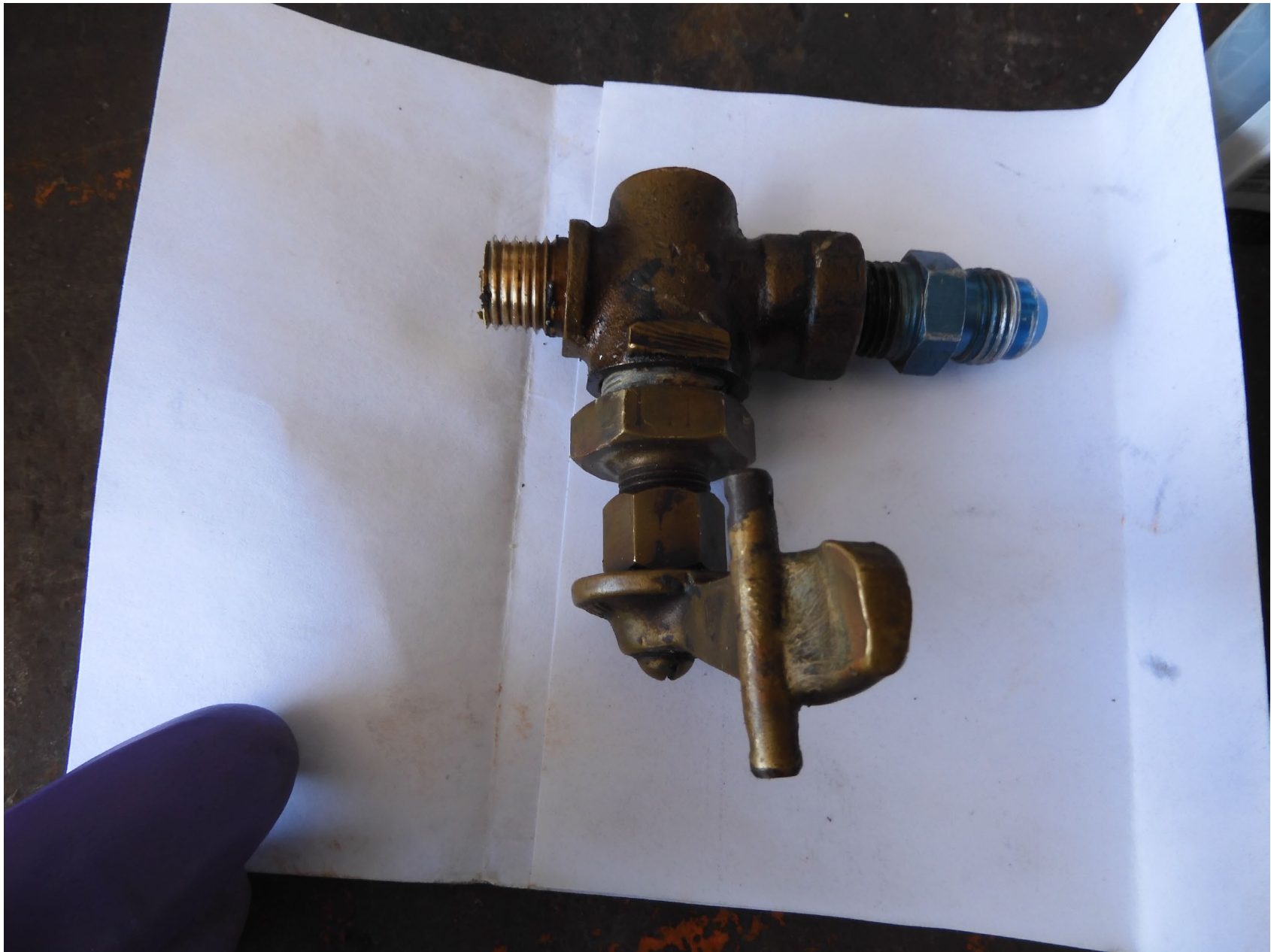
Photo 5 - Fuel shut off valve with the valve handle as found.
