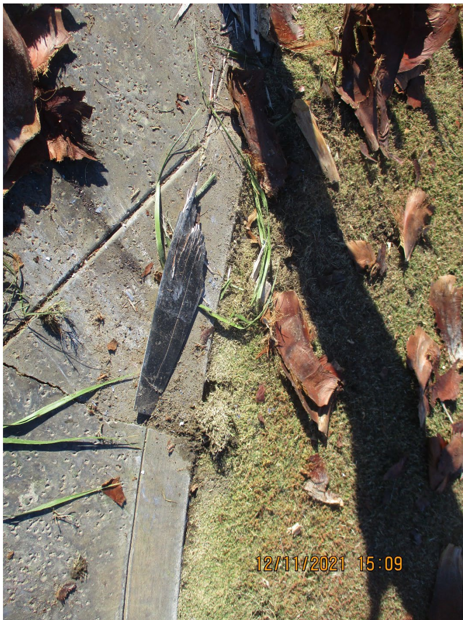
Figure 32. Back-side view of the separated propeller at the accident site, near the palm tree.
