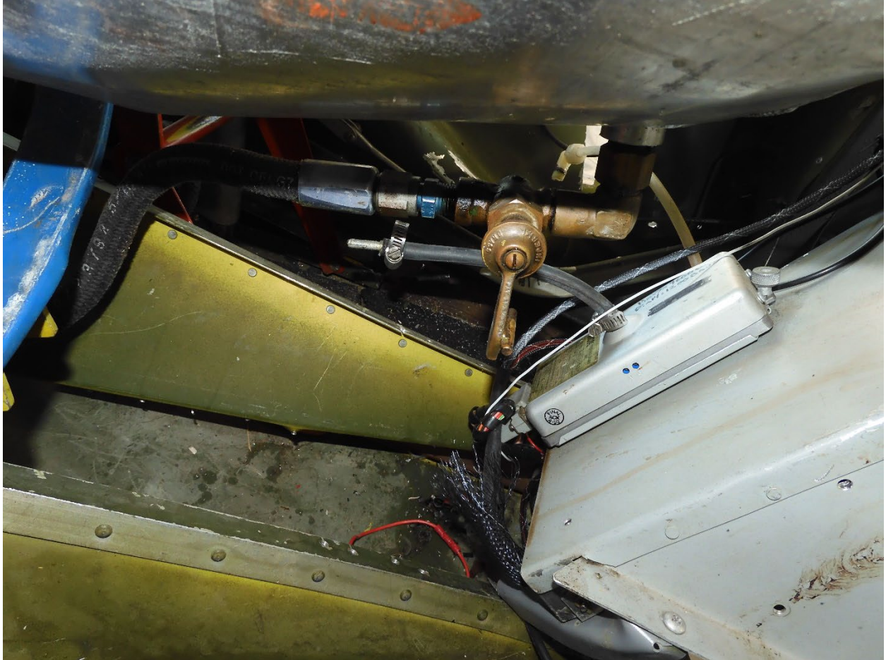
Figure 15. Fuel shutoff valve in intermediate position, as found.
