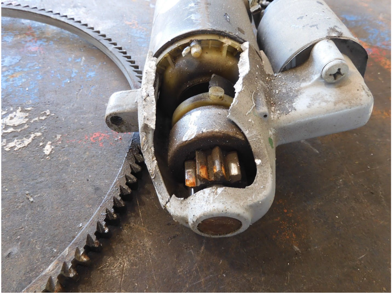
Figure 29. Starter and ring gear, showing no rotational damage to the starter from the ring gear.
