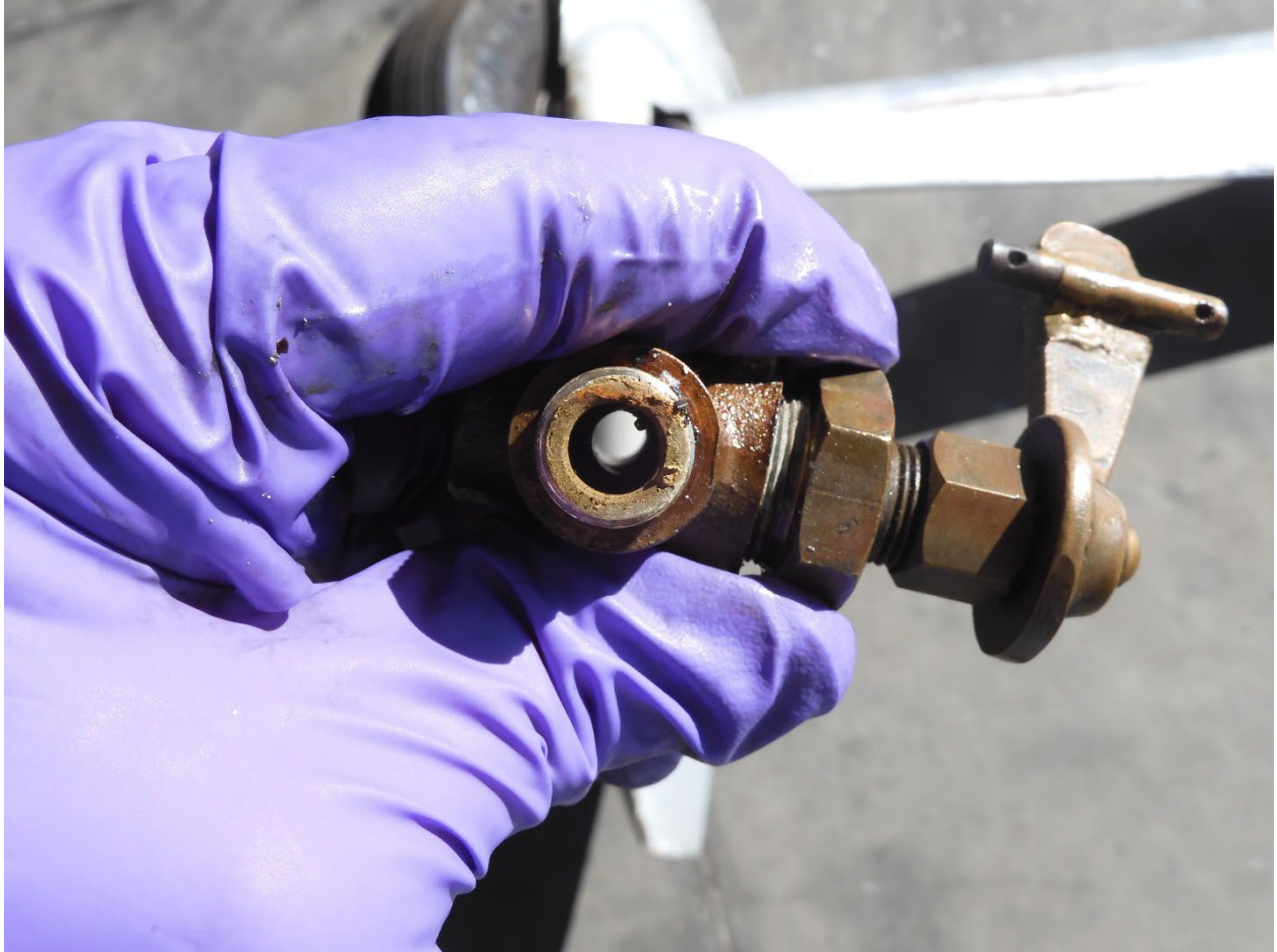
Figure 18. Fuel shut off valve showing the valve at 100% open and the fuel handle at 45° forward.
