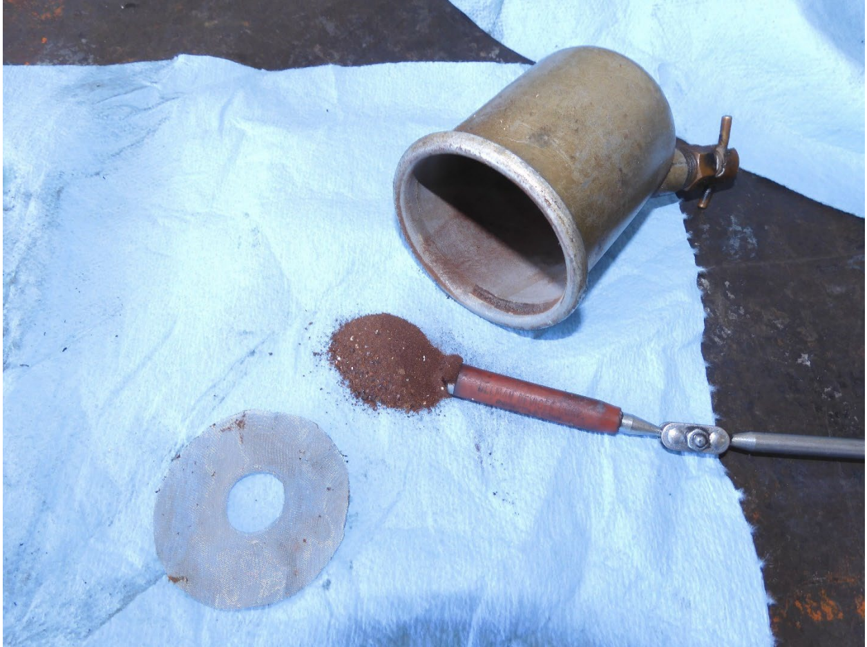
Figure 28. Gascolator bowl and screen, showing metallic rust debris found at the bottom of the bowl.
