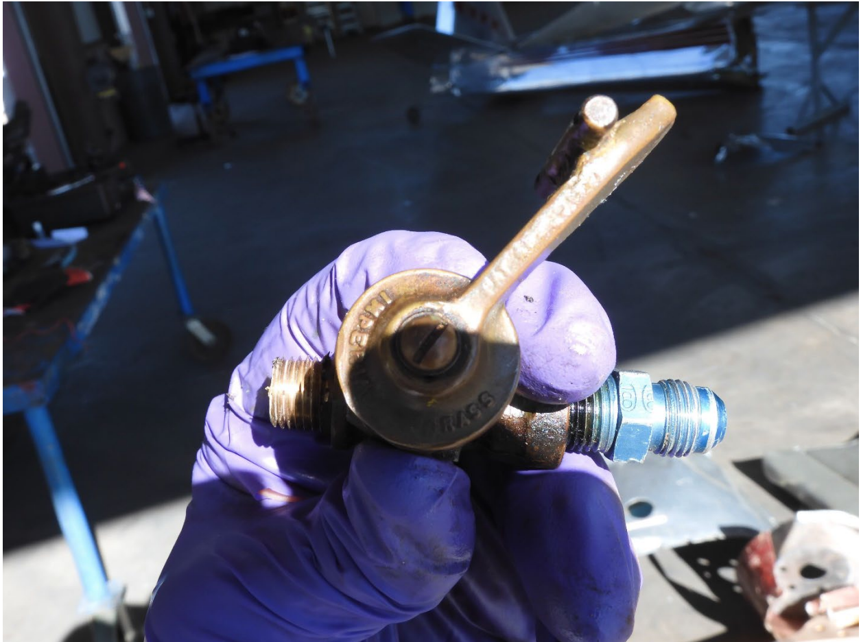
Figure 17. Fuel shutoff valve showing the valve handle position when the opening is at 100% open.
