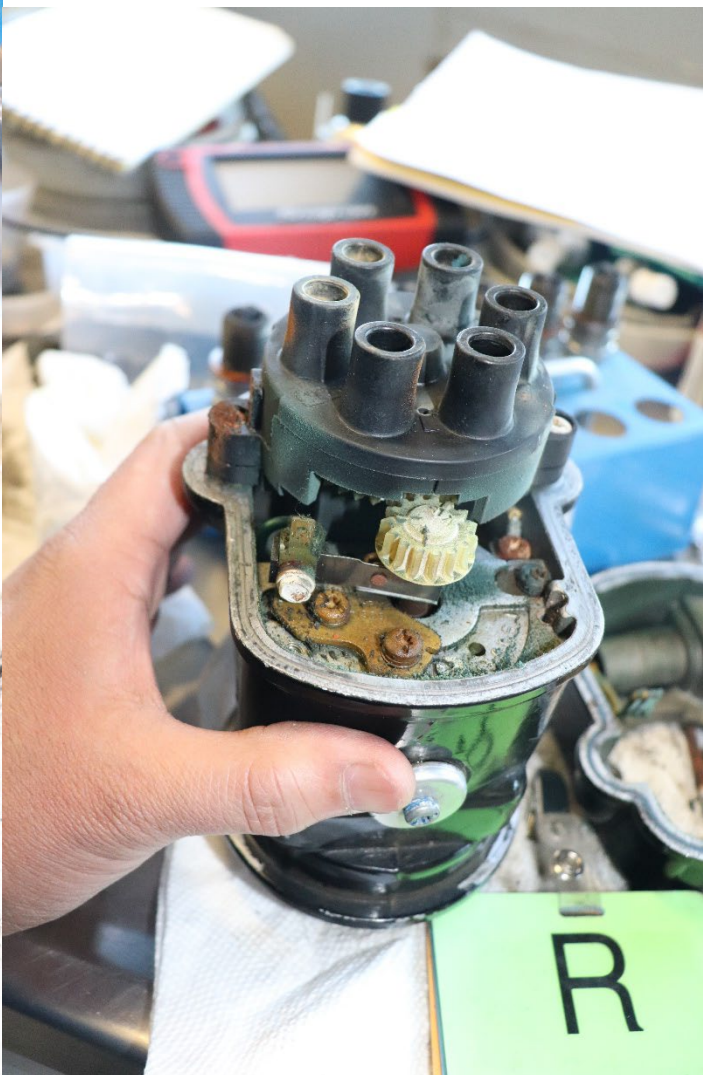
Photograph 5 - View of internal components for right had magneto
