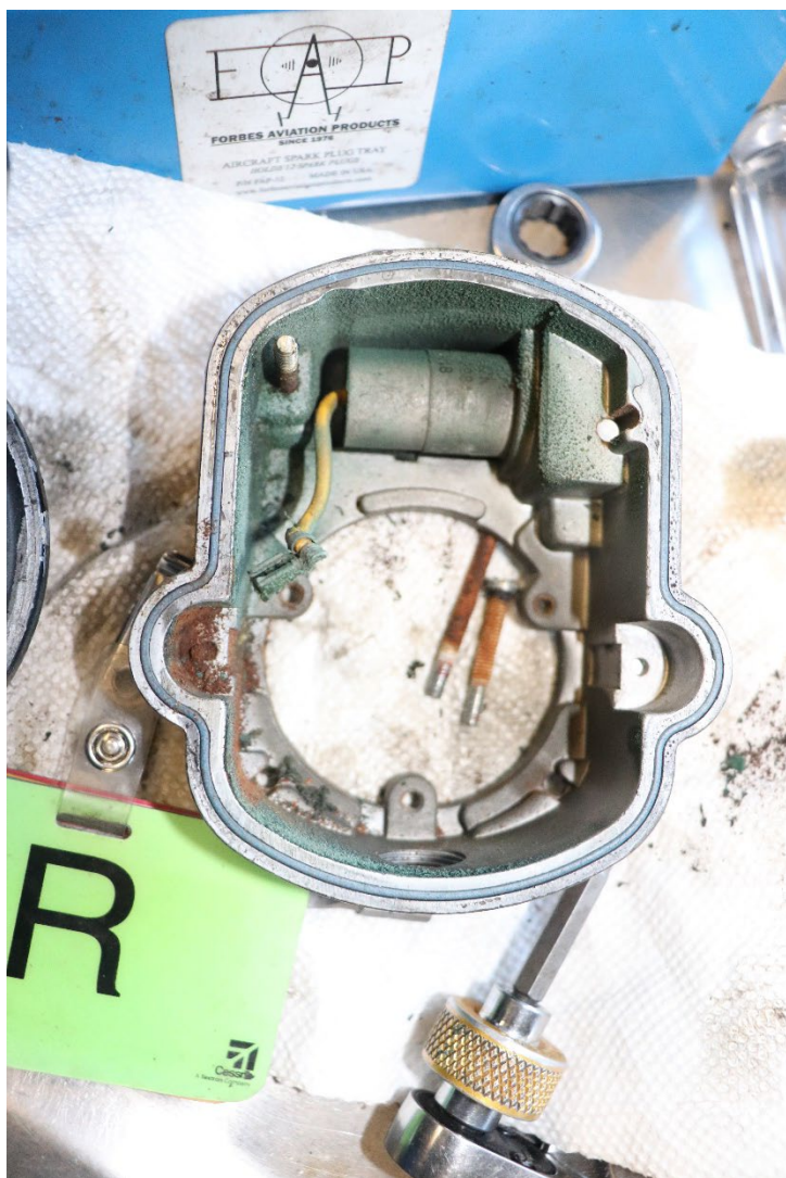
Photograph 5 - View of internal components for right had magneto
