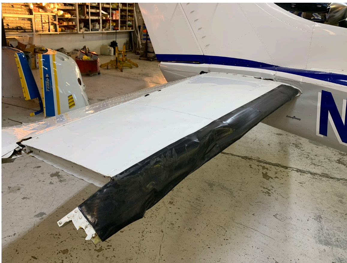
Photograph 2 - View of damaged right horizontal stabilizer
