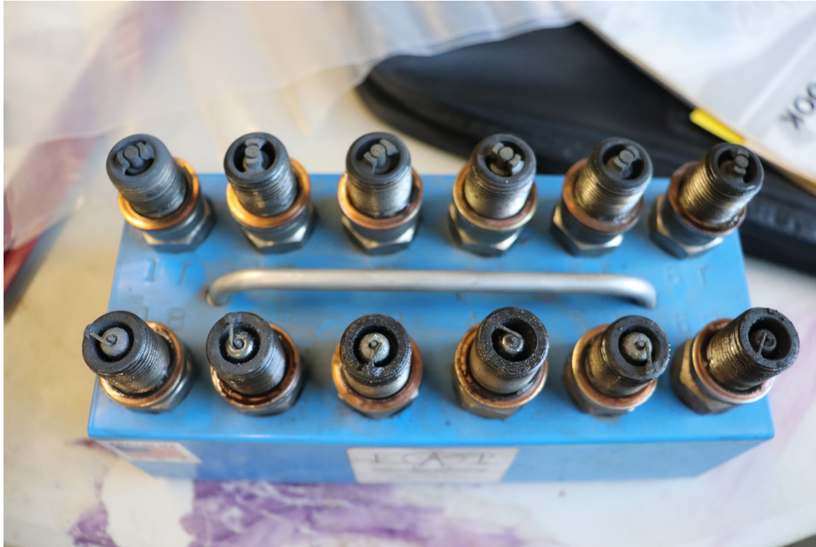
Photograph 4 - View of removed top and bottom spark plugs
