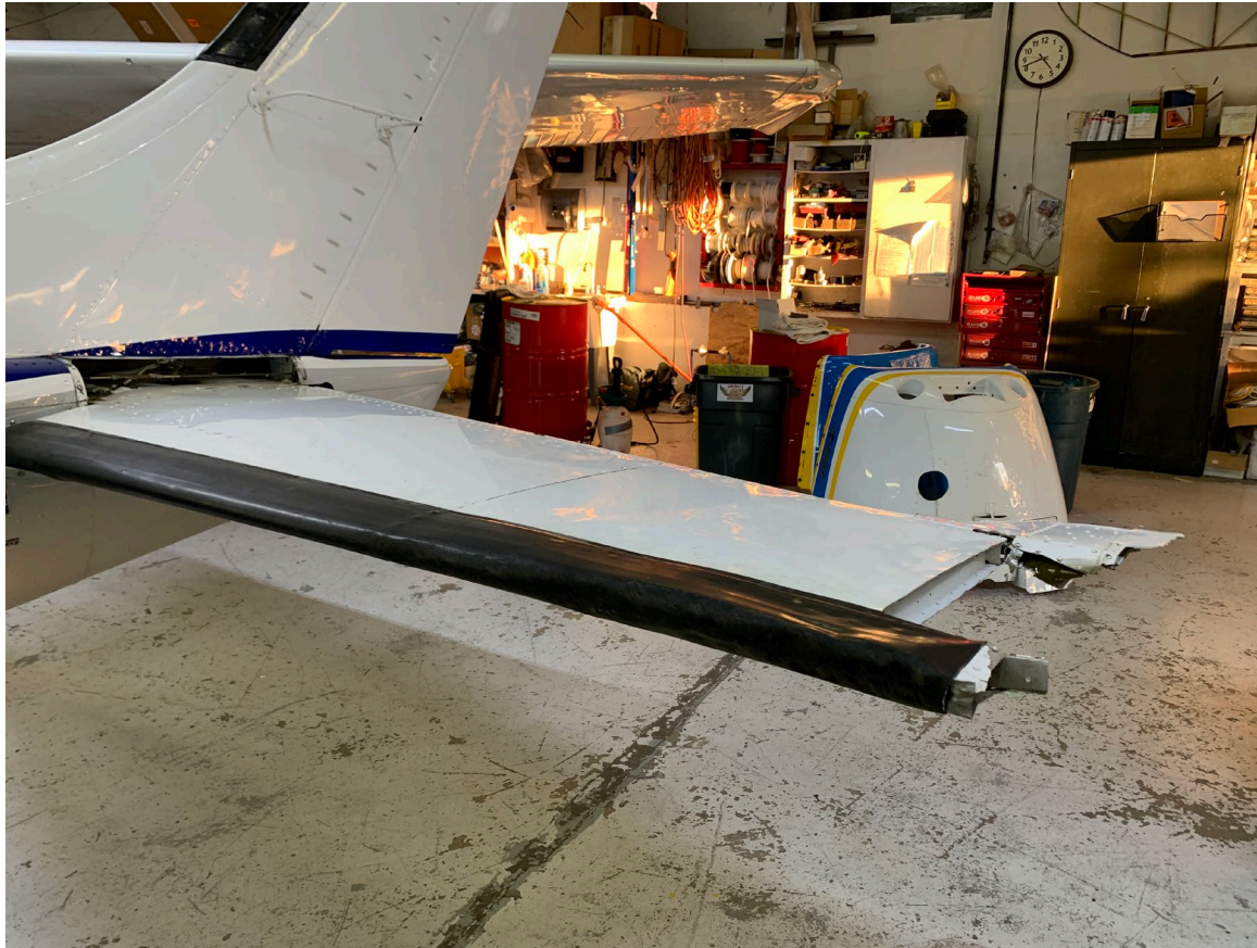
Photograph 1 - View of damaged left horizontal stabilizer
