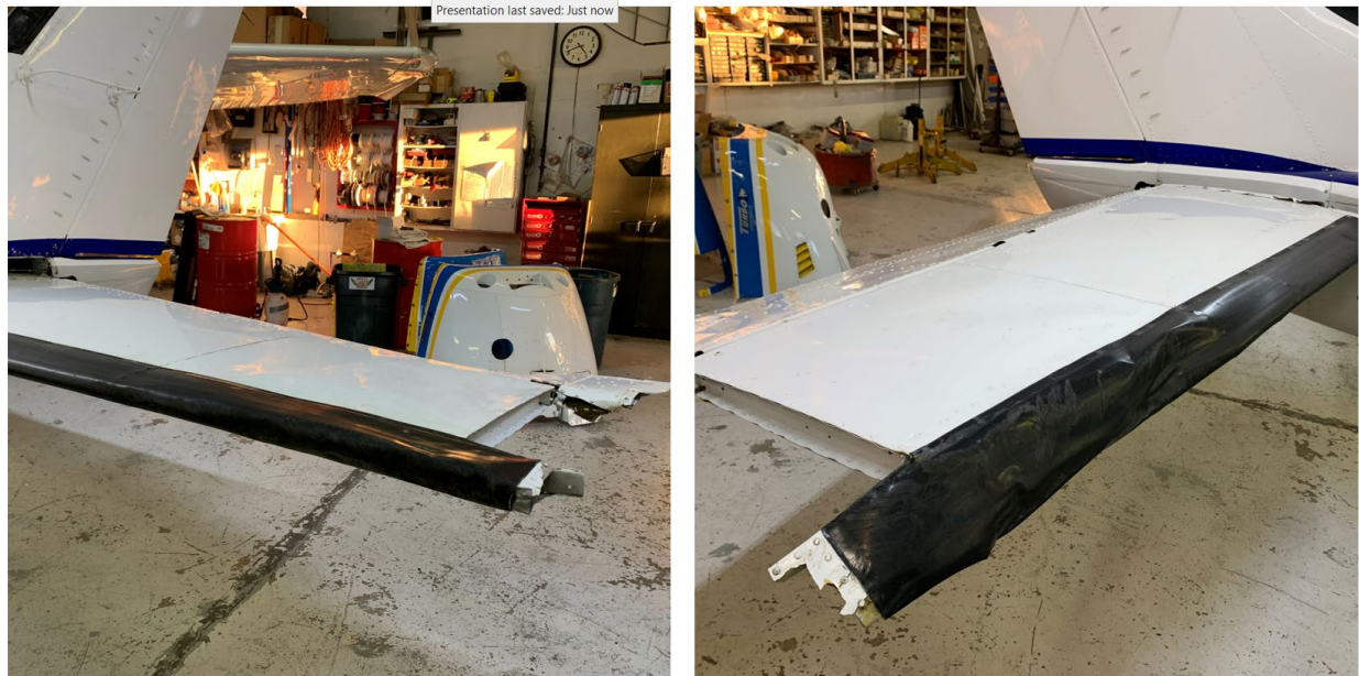
Figure 1. View of damage to left and right horizontal stabilizer.
