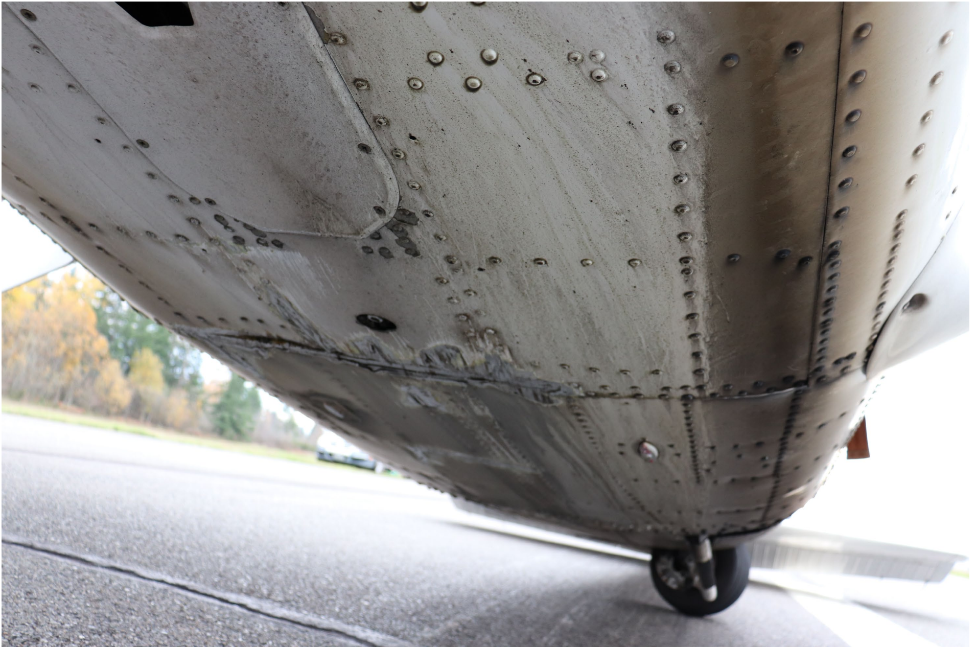
Photo 4 - View of airplane undercarriage damage (photo courtesy of the NTSB)
