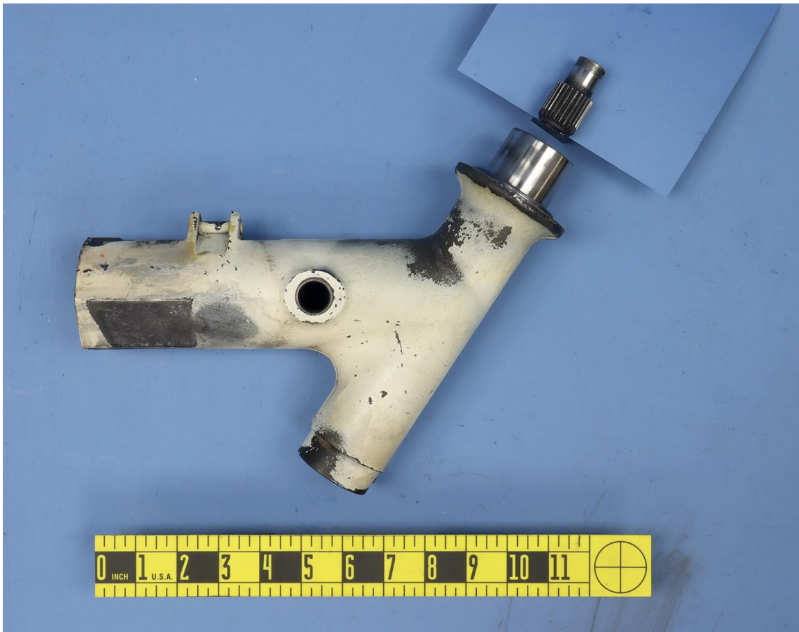
Figure 1: Left main landing gear pivot assembly in two pieces, as received.
