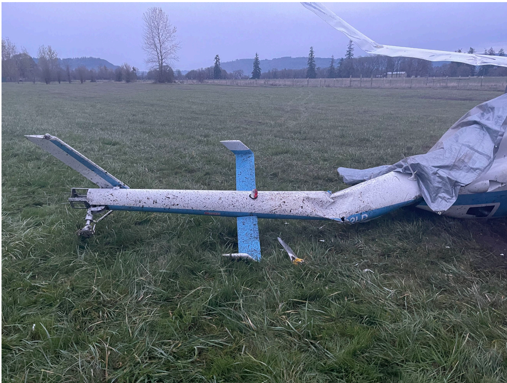
Photo 1 – Right-rear view of N102LD, showing substantial damage to the tailboom. Photo courtesy of the pilot.
