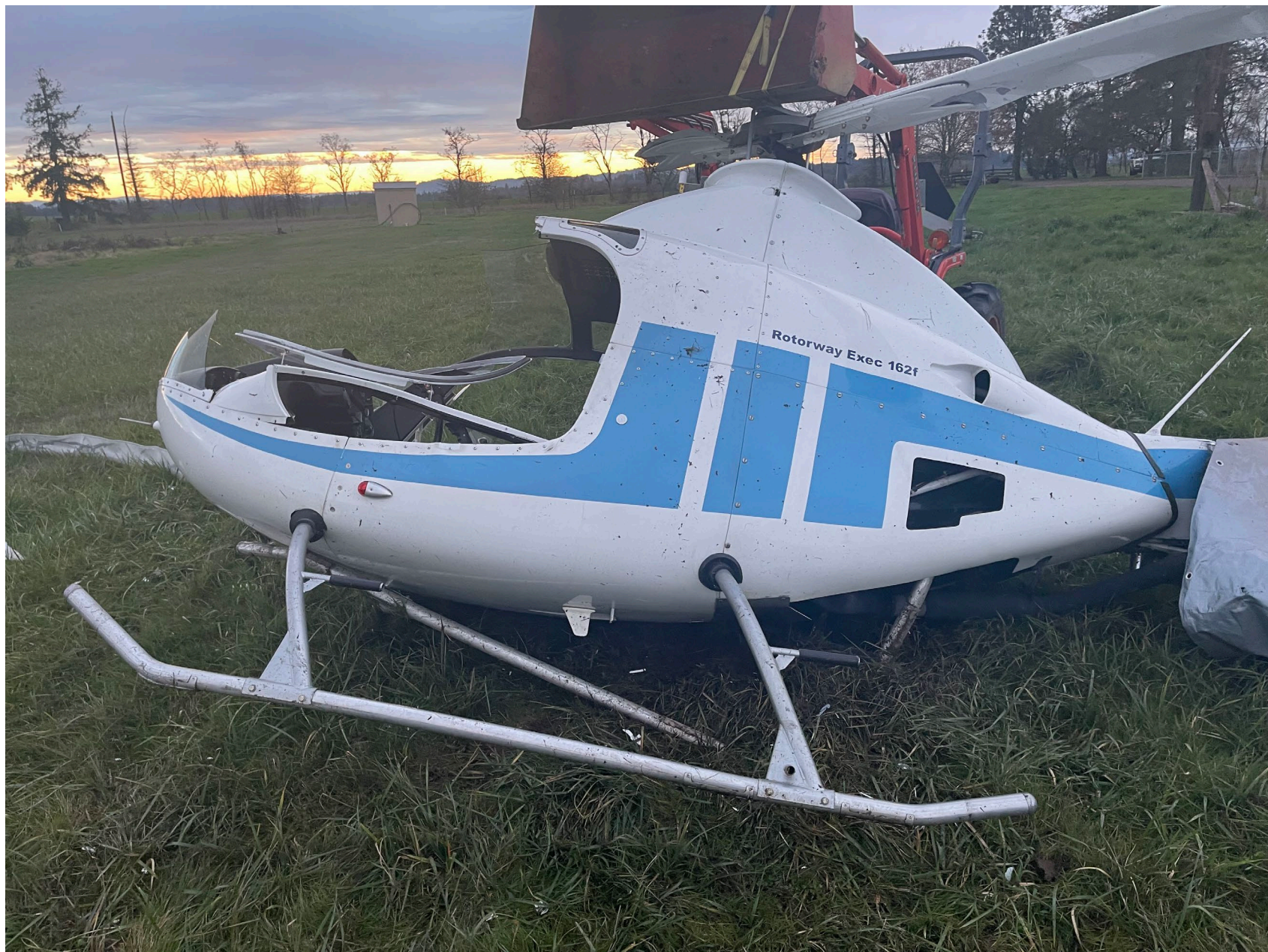
Photo 2 – Left-side view of N102LD, showing substantial damage to the fuselage. Photo courtesy of the pilot.
