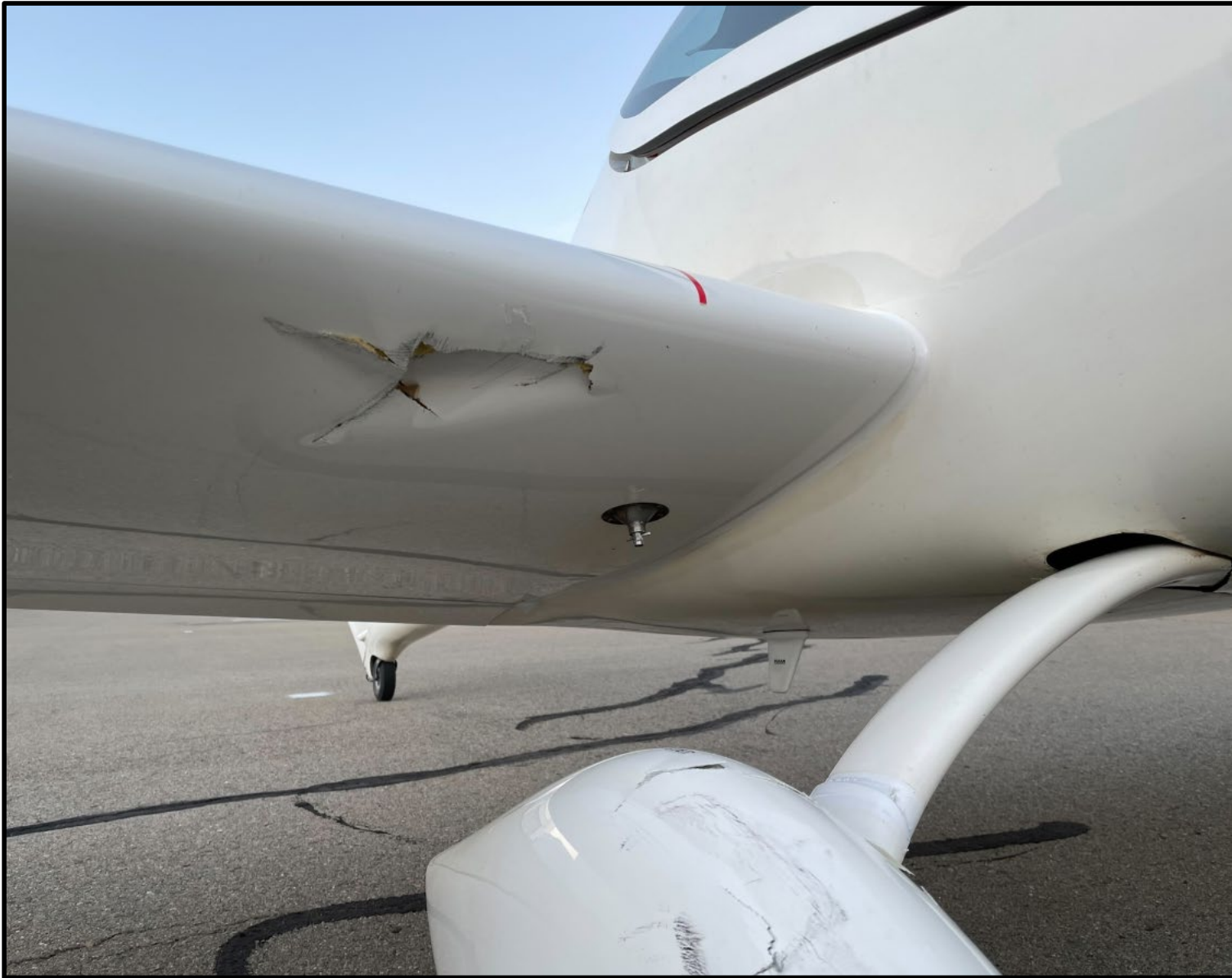
Figure 2: Wing damage (photo provided by Airport Operations)
